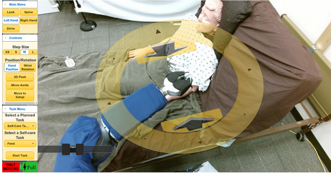
Figure 3.3: The web-based user interface. This interface enables low-level teleoperation by the user as well as the selection of autonomous planned tasks, with optional parameters, selected from a drop-down menu.
