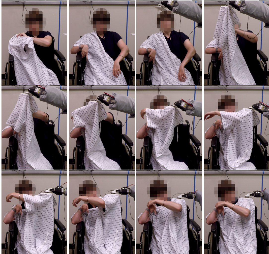
Figure 4.9: A sequence of images (going left-to-right, top-to-bottom) showing a participant successfully putting on the sleeves of the hospital gown with assistance from the robot. This participant independently put on the right sleeve of the gown onto his/her more impaired arm and received assistance with putting on the left sleeve onto his/her less impaired arm. The expected configurations of the participant's body is shown in Figure 4.6(d). The participant's arm pose differed from the expected configuration.
