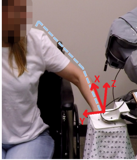
Figure 4.7: The axes used by the controller are shown in red. The axes translate and rotate with the tool. The trajectory for moving along the forearm, upper arm, and shoulder are illustrated in light blue.
