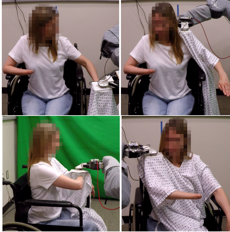
Figure 4.1: Through our system implementation of TOORAD, four participants with disabilities were able to dress themselves with assistance from the robot. (left-to-right) Prior to dressing the left arm; end of dressing the left arm; prior to dressing the right arm; end of dressing the right arm. After successful dressing, both of the participant's arms are in the hospital gown.
