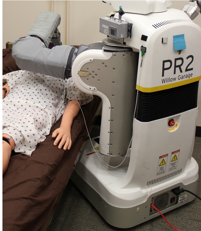
Figure 3.9: Physical collaboration between the two robots. A solution frequently used by the system was to raise the bed and to move the PR2's base under it, so the PR2 could better reach task areas.
