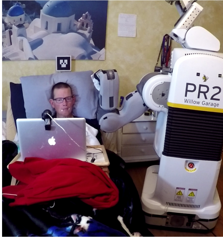
Figure 3.1: The system in use in a person’s home. Henry Evans, a person with severe quadriplegia, used our system in his own home to wipe yogurt from his mouth, visible as white dots on his face.
