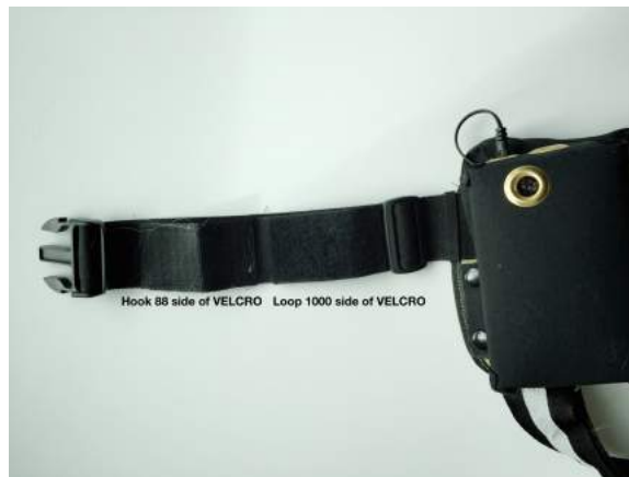
Figure 11: The folded strap mechanism was made to account for dogs of multiple sizes.
