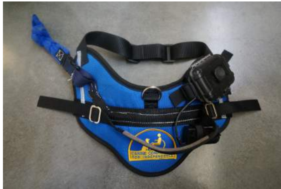
Figure 6: Prototype 2 with the opaque enclosure now placed on the side.
