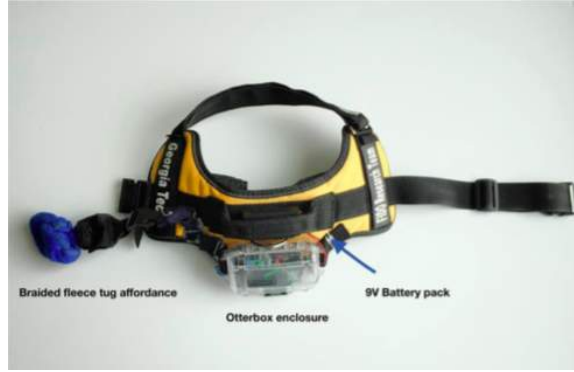
Figure 5: Prototype 1 used a Julius K9 harness with electronics components mounted on the top.
