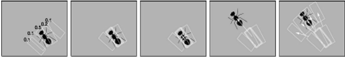
Figure 2.5: (a) White rectangles represent particles, scored based how well the underlying pixels match the model. (b) New particles are sampled according to the probabilities. (c) Estimated location (white plus) is calculated from the new particles. (d) The next image frame. (e) Particles are advanced according to the stochastic motion model. From [Balch et al 2005].
