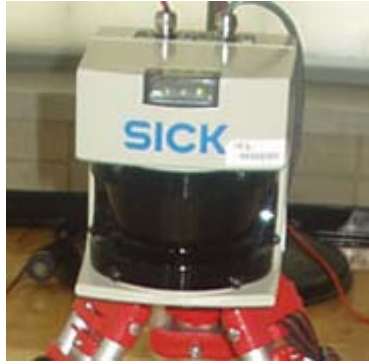
Figure 2.2: A SICK LMS-291 laser range finder.
