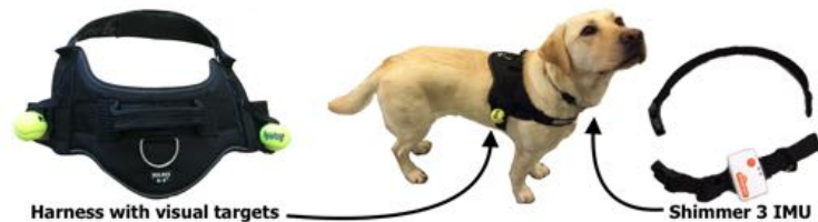
Figure 26. Participant wearing the instrumented Julius K9 harness and Shimmer 3 before a training session.
