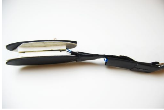
Figure 8. The oval-shaped bite interface improved results by inducing the bite force to be applied vertically.
