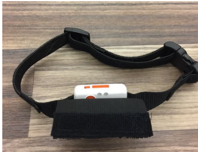
Figure 33. Final enclosure and orientation to hold the shimmer sensor parallel to the collar.
