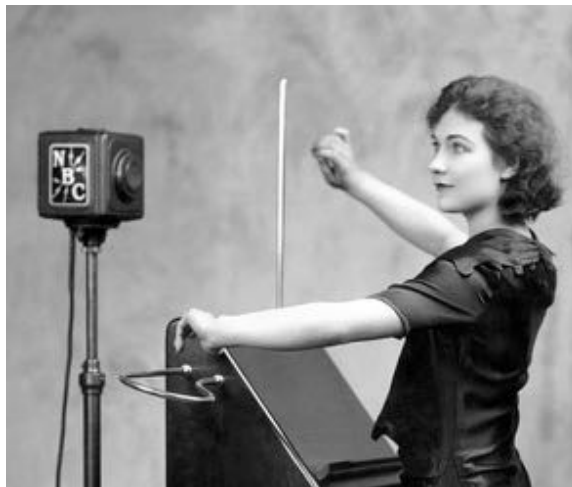
Figure 5. The Theremin, an early gesture-based system, is an electronic musical instrument controlled by the movements of a performer.
