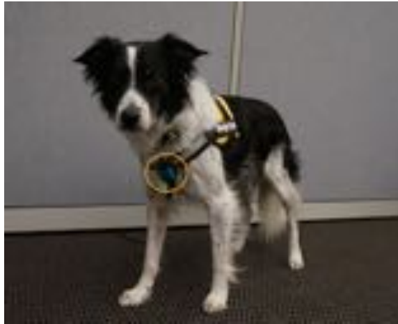
Figure 13. We used the Axivity accelerometer (circled) in this first experiment.
