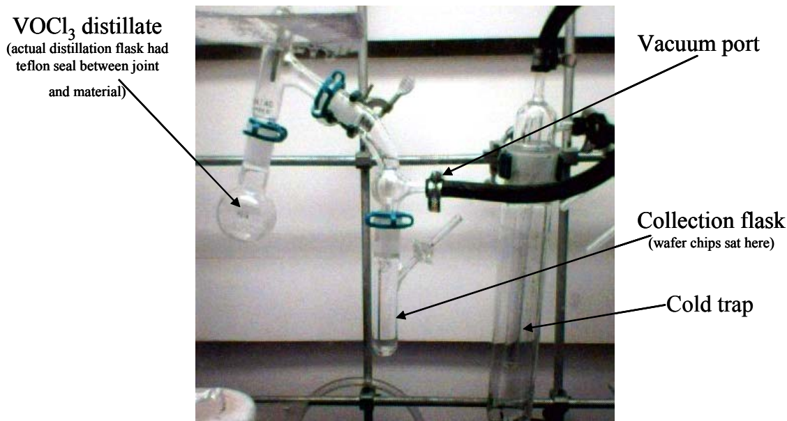
Figure 4.3: Apparatus used for \text{VOCl}_3 reaction
