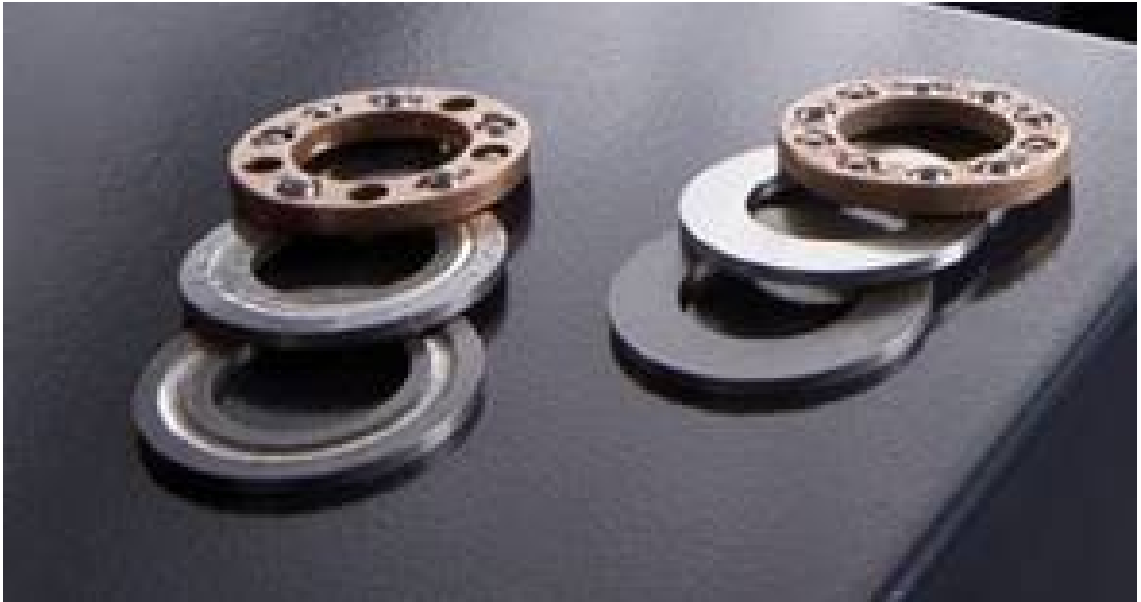
Figure 6 A new bearing (right) and a failed bearing (left).
