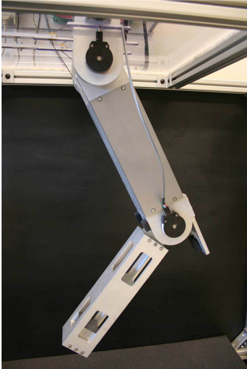
Figure 8: The completed robotic leg with both joint flexed. The joint angle encoders can be seen as the black sensors at each joint. The padded metal component extending from the thigh models the hard-stop component of knee asymmetry.
