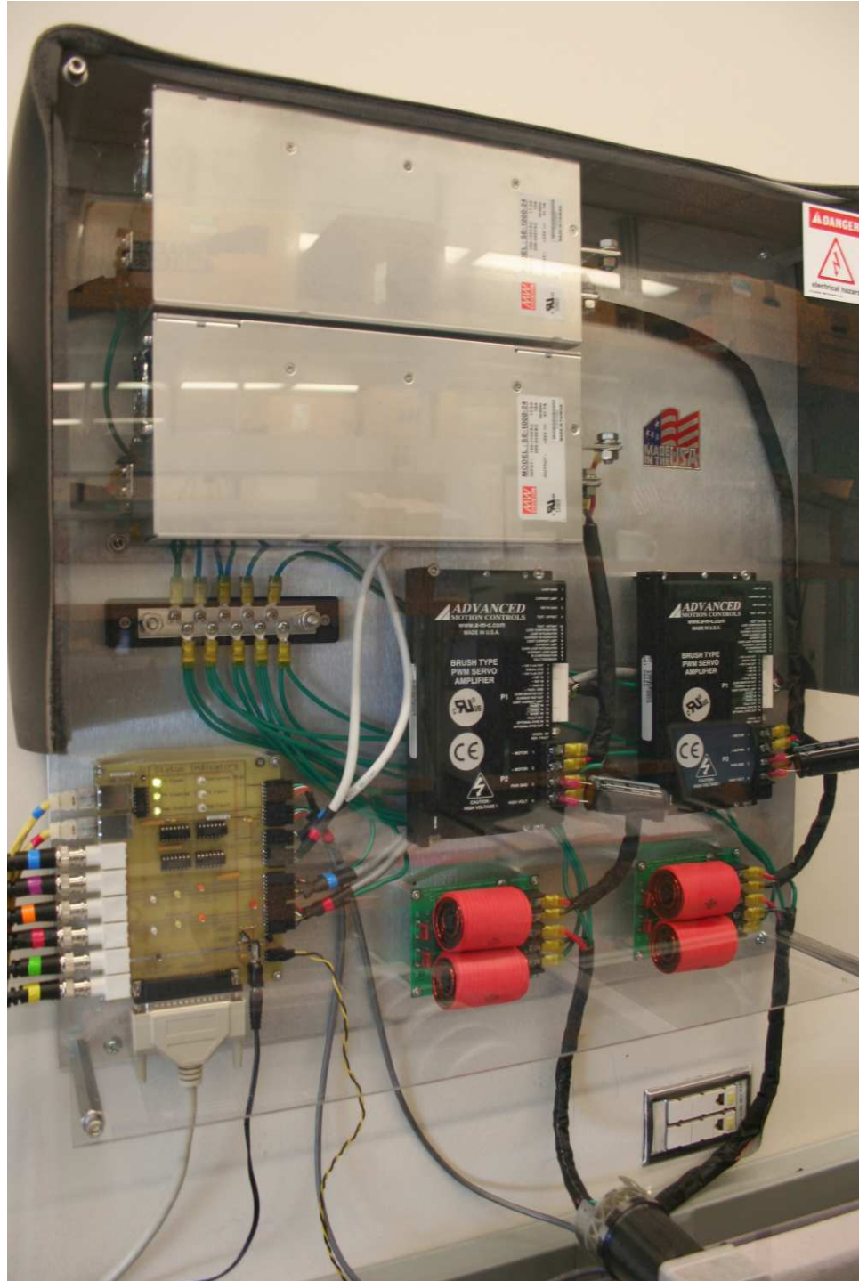
Figure 11: Electrical system used to provide power and signal amplification to the robotic leg's actuators and sensors. The power supplies are the two large silver boxes at the top; the amplifiers are the two black rectangular components to the center right; the series inductor boards are located at the bottom right; and the custom interface board is located at the bottom left. Directly above the interface board is a grounding strip used to provide a common reference voltage for all components.
