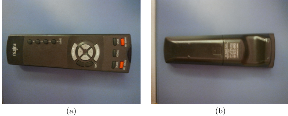
Figure 17: The top and bottom of the television remote. The support distribution of the remote is much more complex than a simple polygon. Additionally the narrow end is significantly more massive than the wider end owing to the batteries inside.
