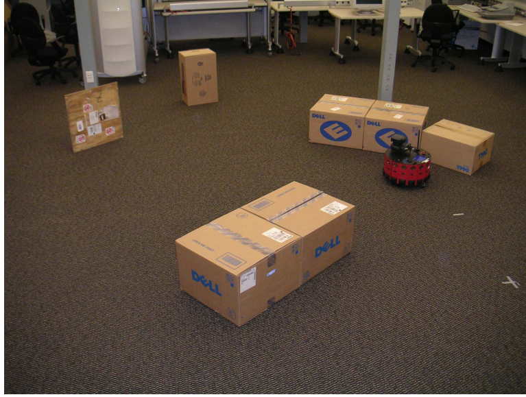
Figure 32: Experimental setup for testing our real time reactive navigation method.
