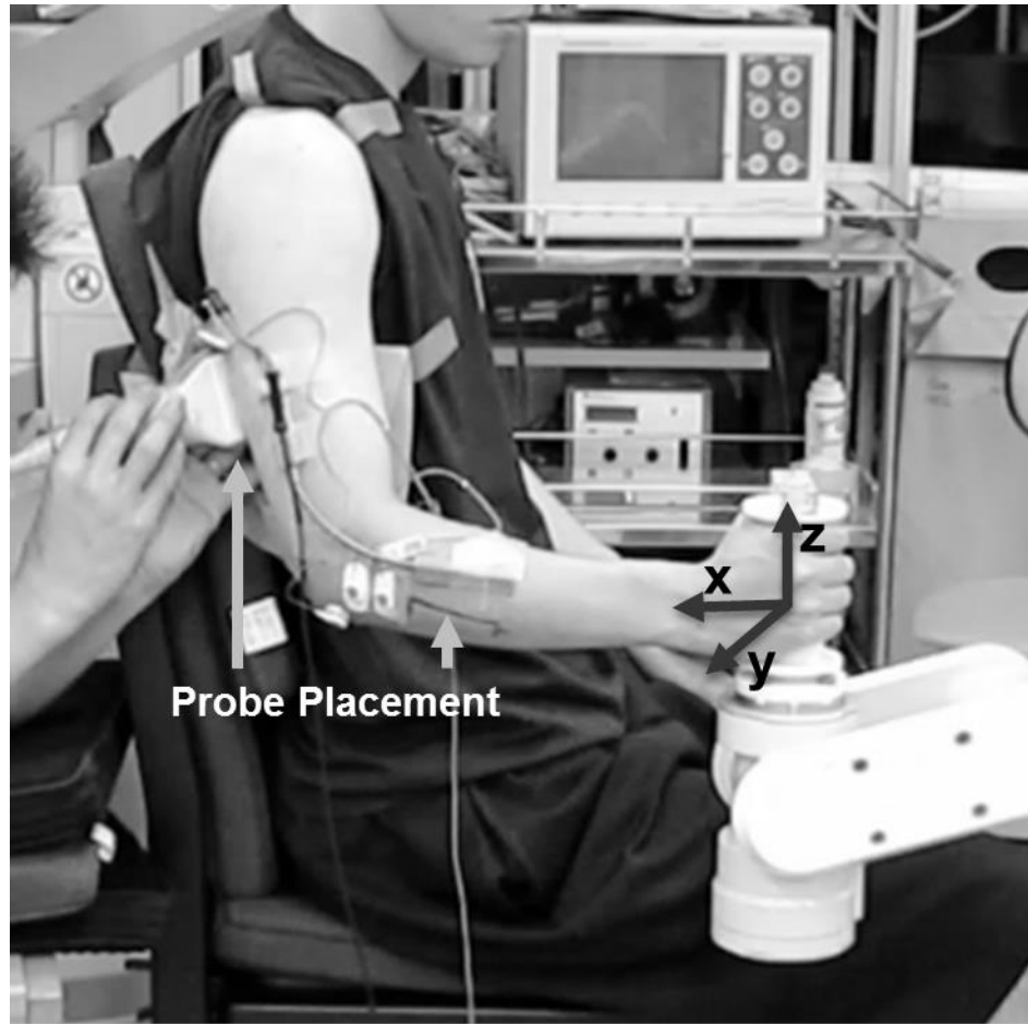
Figure 6: A photo that includes the current experimental setup, taken during a pilot experiment. Axes of loading for robotic manipulator are: positive x , y and z axes point toward the subject, to the right of the subject, and upward, respectively. Note that the subject is being prepared for an upcoming trial, thus the elbow has not yet been adjusted to 90^\circ of flexion. In addition, pilot EMG signals were explored for a purpose not addressed in this dissertation but were deemed unreliable due to motor noise from the robot.
