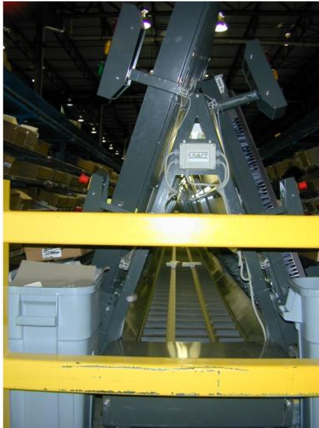
Figure 1.7: Cross-section view of A-frame, with safety rail.
