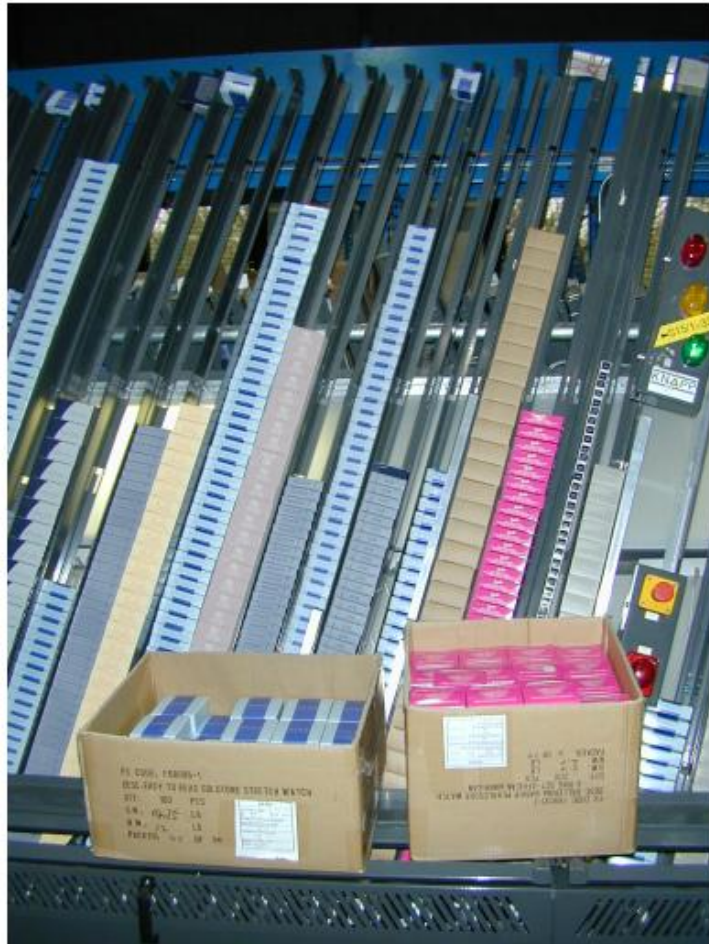
Figure 1.8: Dispenser channels on A-frame
