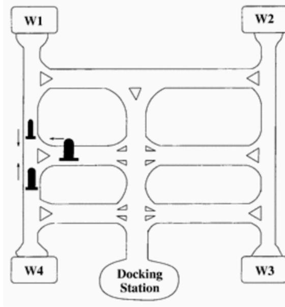
Figure 2.1: Depiction of deadlocked AGVs at an intersection. Any multi-agent scheduling algorithm must prevent such situations from occurring.
