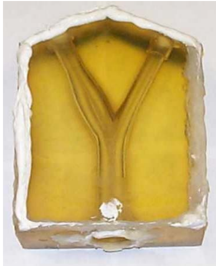
Figure 1. Sylgard phantom based on the model developed by Balasubramanian (1980).
