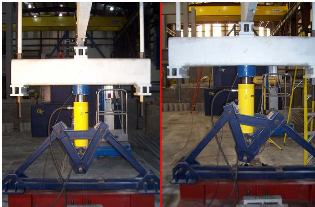
Figure 3.4 – (a) Undeformed and (b) Deflected configurations of the gravity load simulator
