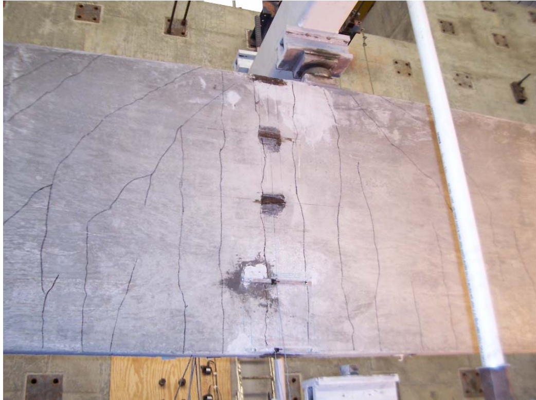
Figure 7.4 –Vertical cracks on the convex face of B44-2 at midspan after buckling
