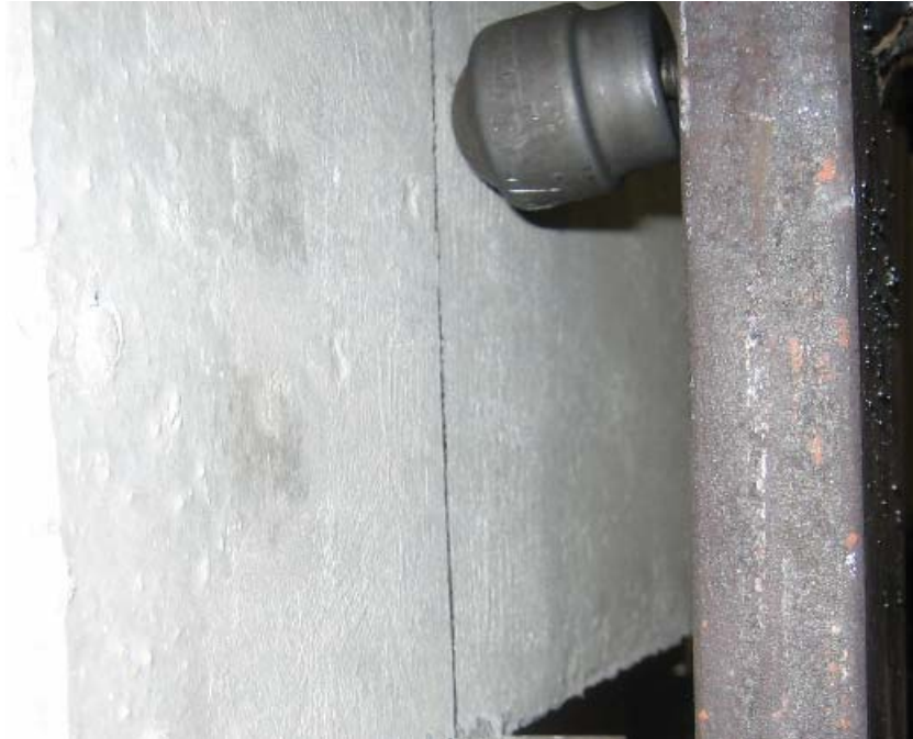
Figure 3.13 – Bending of the ball roller
