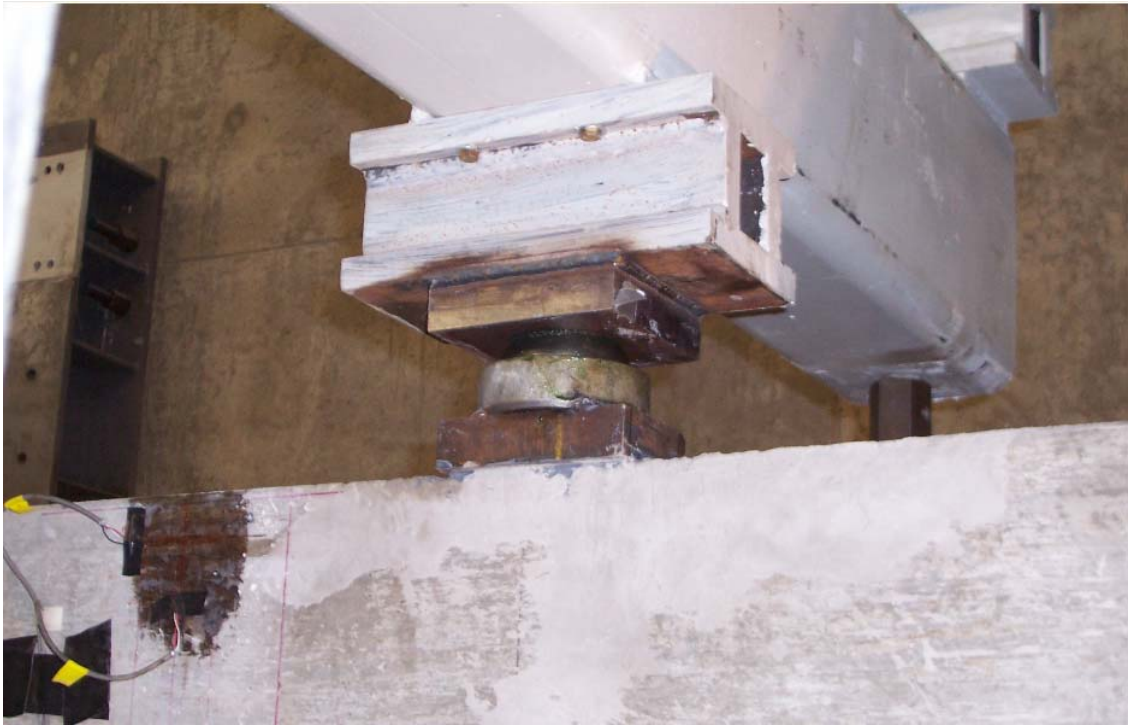
Figure 3.5 – Ball-and-socket joint
