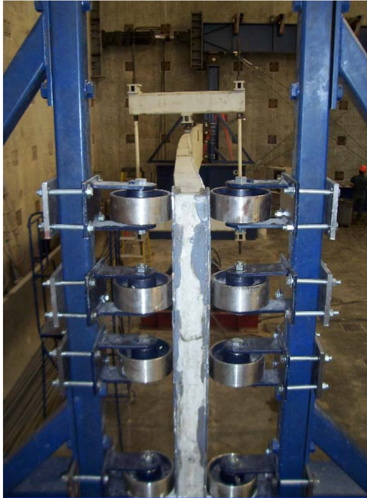
Figure 3.8 – Lateral deformations and torsional rotations restrained at the supports
