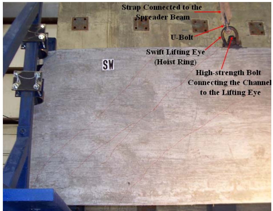
Figure G.4 – The Lifting point in the second set of beams connected to the spreader beam
