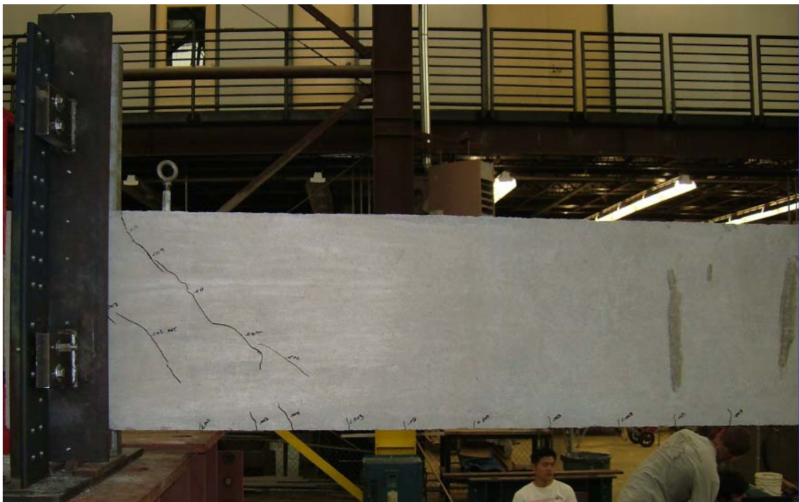
Figure 7.8 –Diagonal tension cracks on the concave face of B18-2 after buckling
