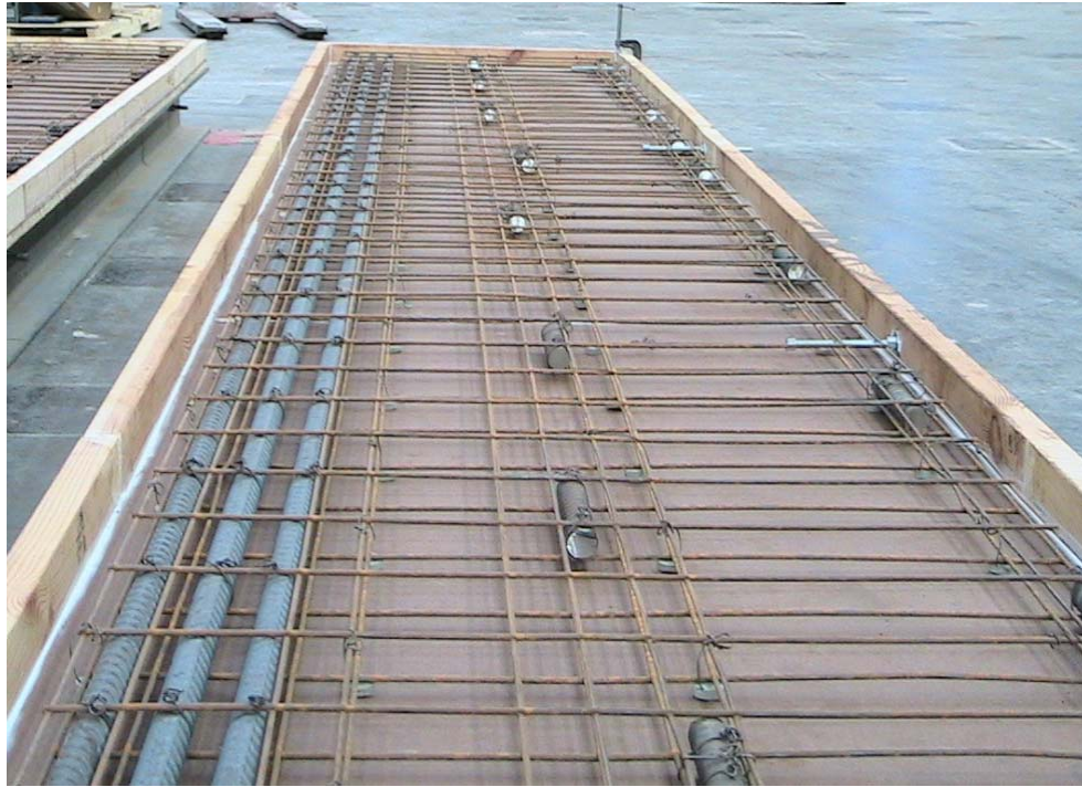
Figure G.1 – Reinforcement in Specimen B36
