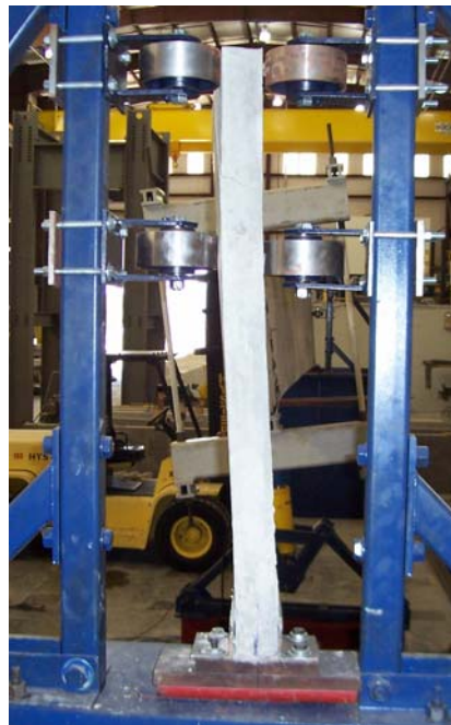
Figure 3.17 – Distortion in the cross-section at the beam end
