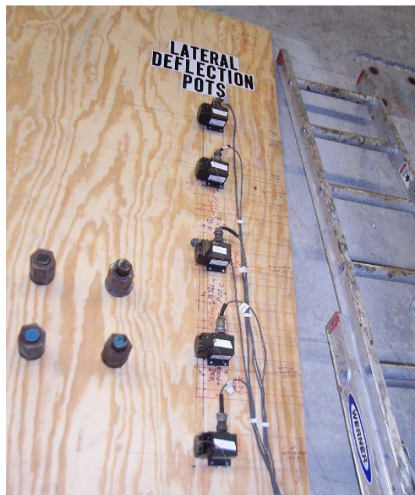
Figure 3.22 – Lateral deflection potentiometers in the second set of experiments
