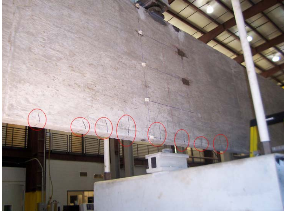
Figure 7.3 – Flexural cracks on the concave face of B44-3 at midspan before buckling
