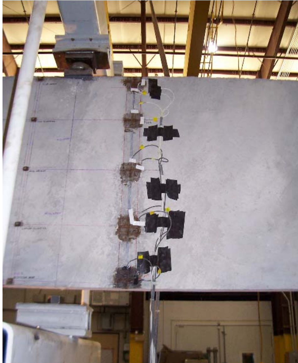
Figure 3.24 – Strain measurement through electrical resistance strain gauges in the second set of tests
