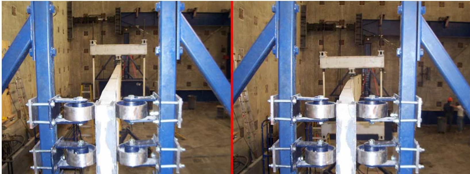
Figure 3.6 –The vertical orientation of the loading cage (a) before the test; (b) after buckling
