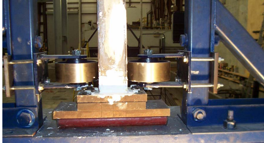
Figure 3.10 – Roller supports at the beam ends in the second set of experiments
