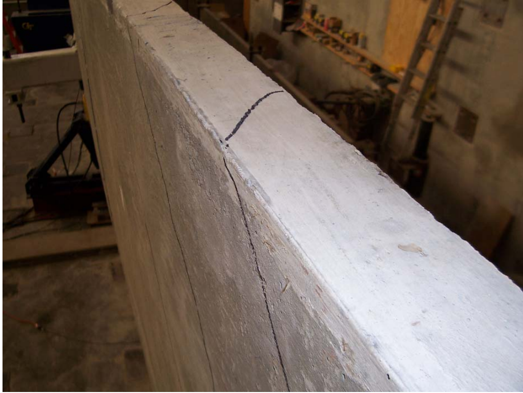
Figure 7.9 –Diagonal tension cracks continuing on the top surface of B44-2 after buckling
