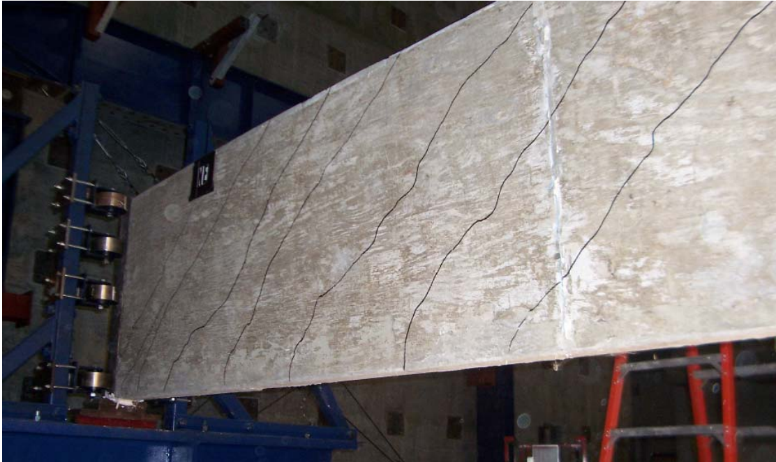
Figure 7.7 –Diagonal tension cracks on the convex face of B36L-1 after buckling
