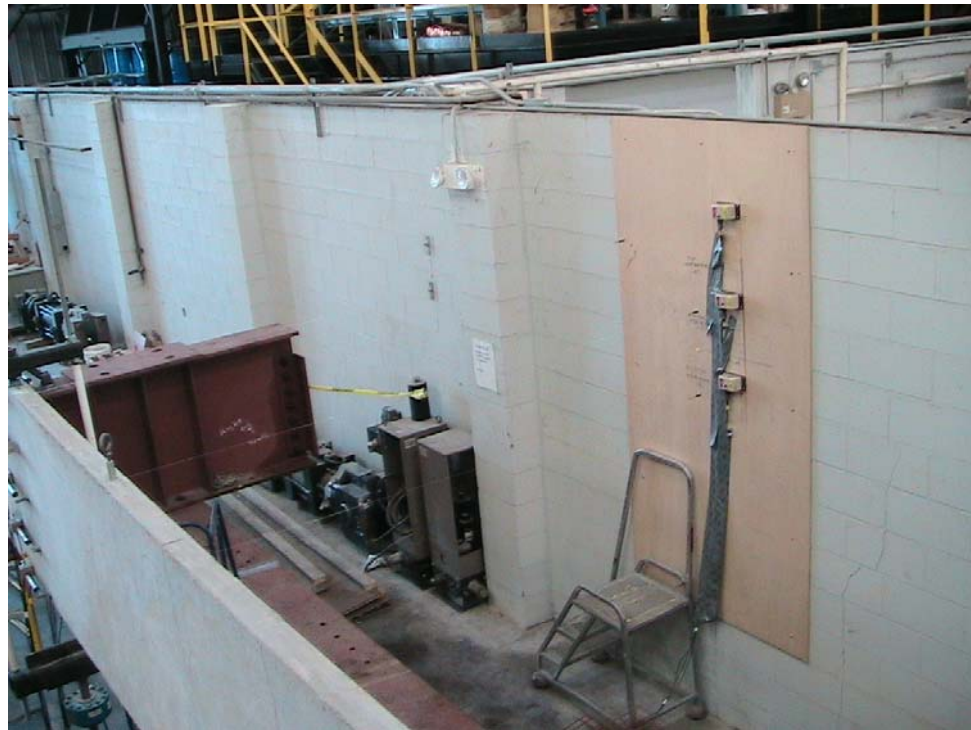
Figure 3.21 – Lateral deflection potentiometers in the first set of experiments
