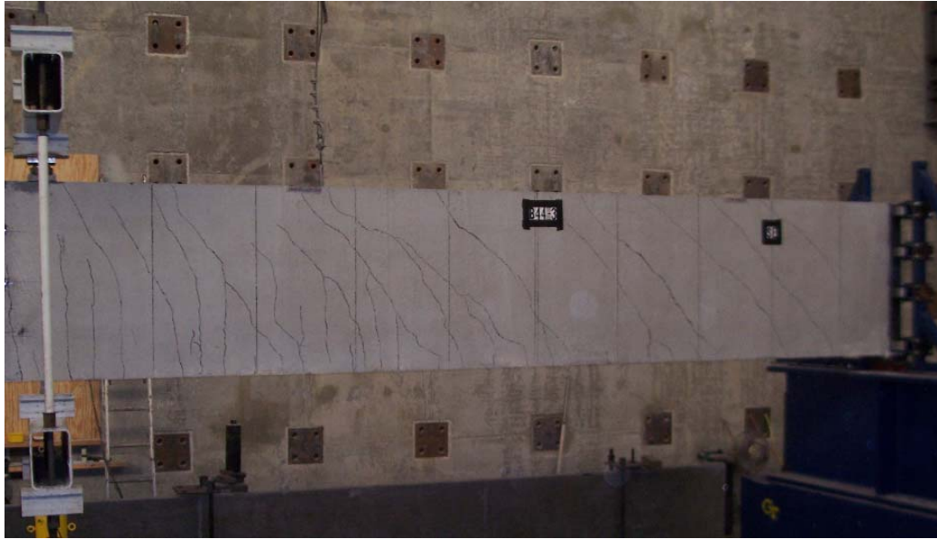
Figure 7.1 –Typical crack pattern on the convex faces of the specimens after buckling
