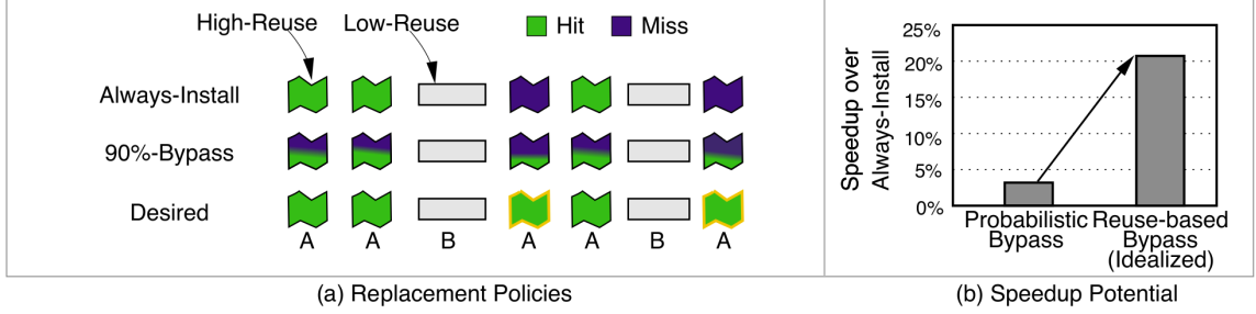
Figure 5.1: (a) Always-Install, 90%-Bypass, and Desired replacement policies under mixed high-reuse low-reuse access pattern. (b) Potential for speedup: Probabilistic Bypass [17], and Ideal Reuse-based Bypass with no state-update cost.
