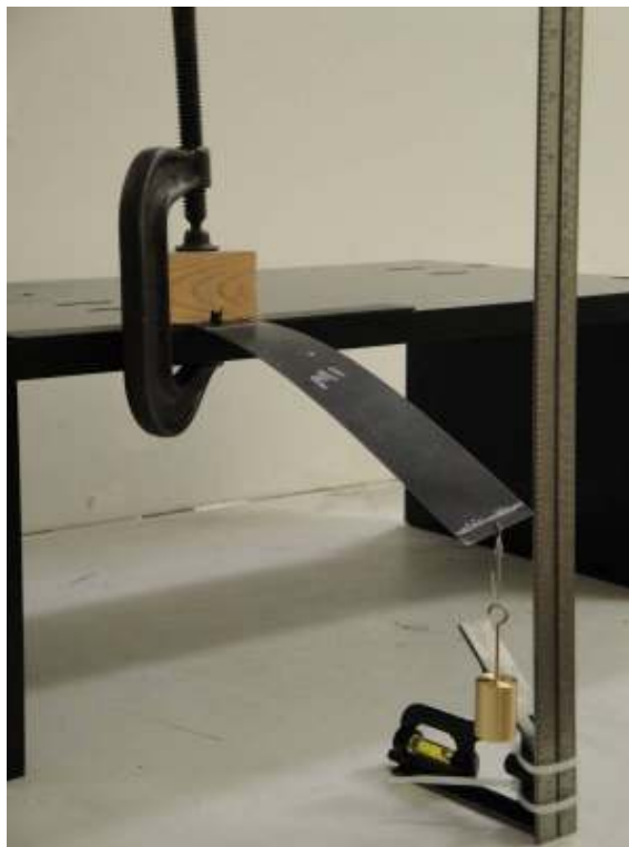
Figure 33. Specimen Undergoing Bend-twist Coupling Testing
