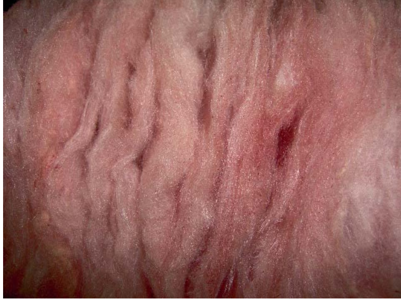
Figure 27. Photograph that illustrates the layered structure of fiberglass.
