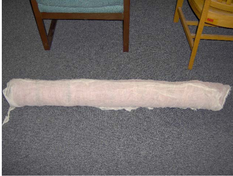
Figure 39. Wrapped cylinder of fiberglass before it is inserted into the transmission line.
