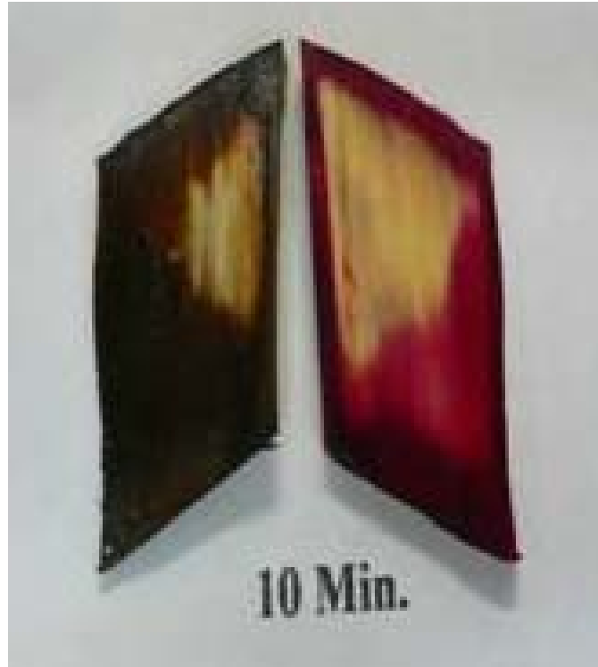
Figure 4-10 Sulfide and hydroxide diffusion into sweetgum at 10 minutes
