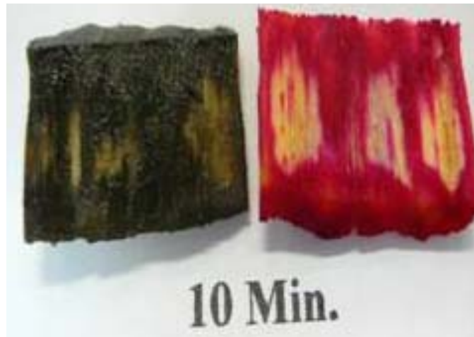
Figure 4-14 Sulfide and hydroxide diffusion into pine at 10 minutes
