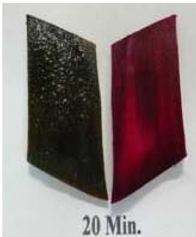
Figure 4-12 Sulfide and hydroxide diffusion into sweetgum at 20 minutes
