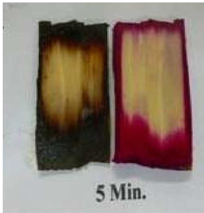
Figure 4-9 Sulfide and hydroxide diffusion into sweetgum at 5 minutes
