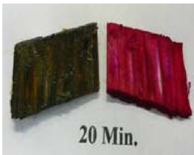
Figure 4-16 Sulfide and hydroxide diffusion into pine at 20 minutes
