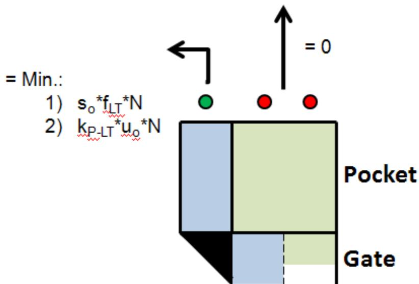
Figure 20 - Pocket Region Left Turning Vehicle Outflow Constraints
