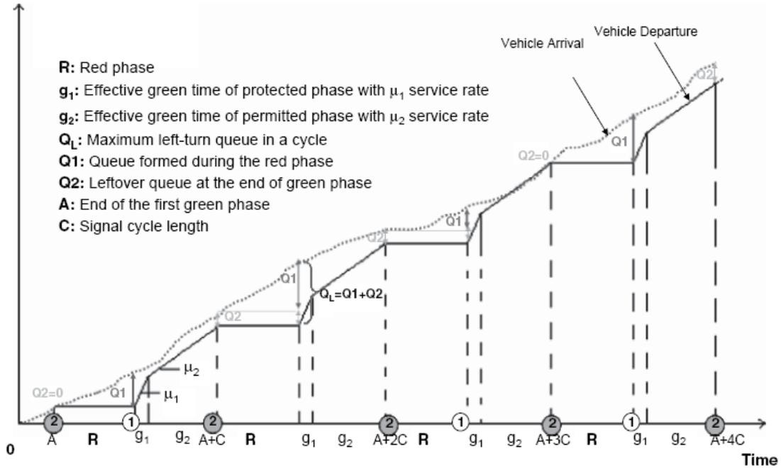
Figure 3 - Cumulative vehicle arrival and departure curve (Qi et al., 2007)
