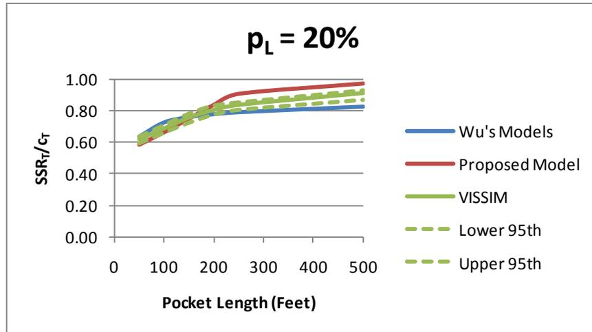
Figure 49 - Model Comparison (Through SSR with two approach lanes)
