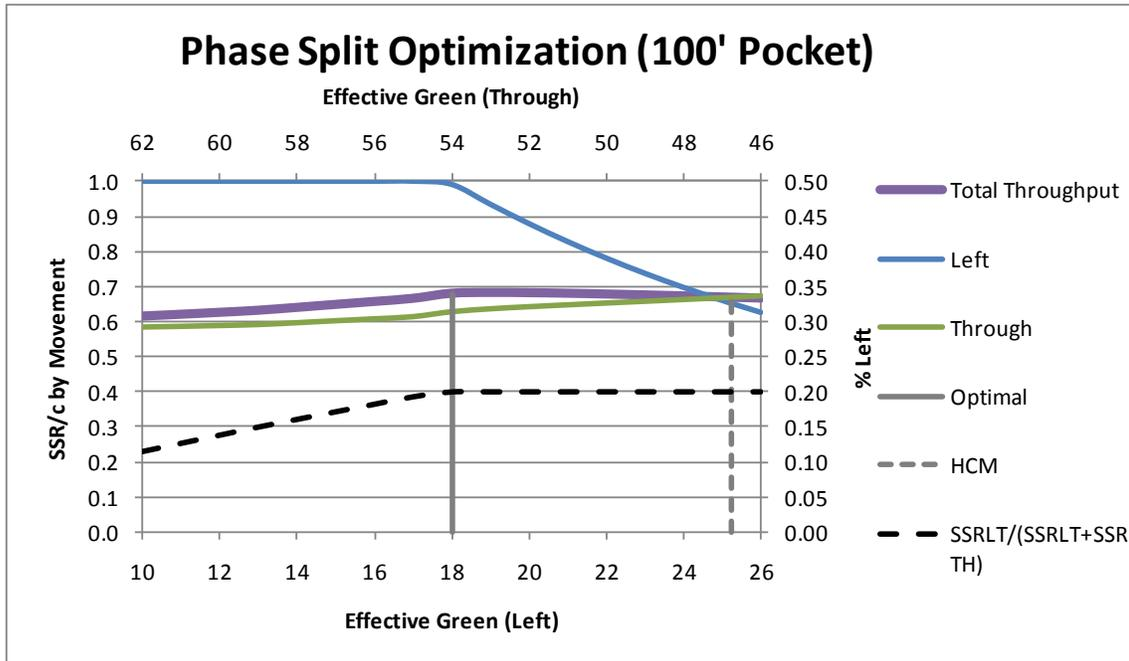
Figure 42 - Phase Split Optimization Procedure - 100' Pocket (SSR/c)
