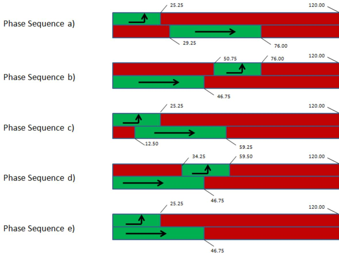
Figure 29 - Phase Sequence Input Example
