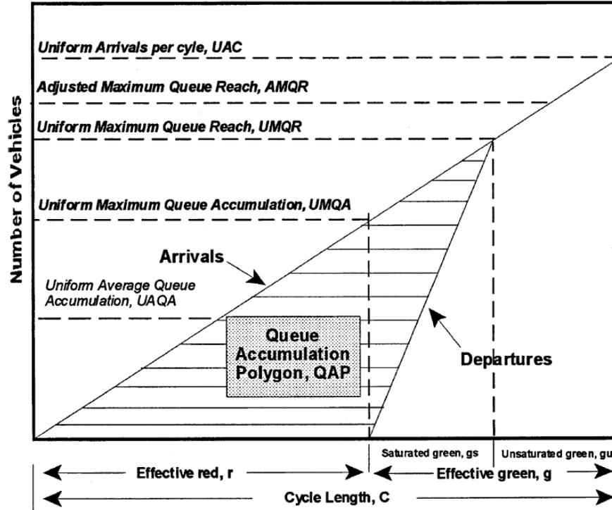
Figure 1 - Queue Accumulation and Discharge (Viloria *et al*, 2000)
