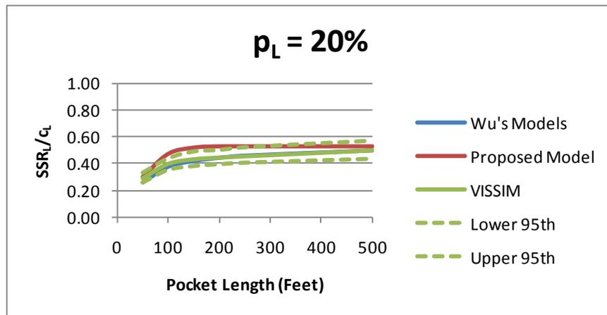
Figure 46 - Model Comparison (Left SSR with single approach lane)
