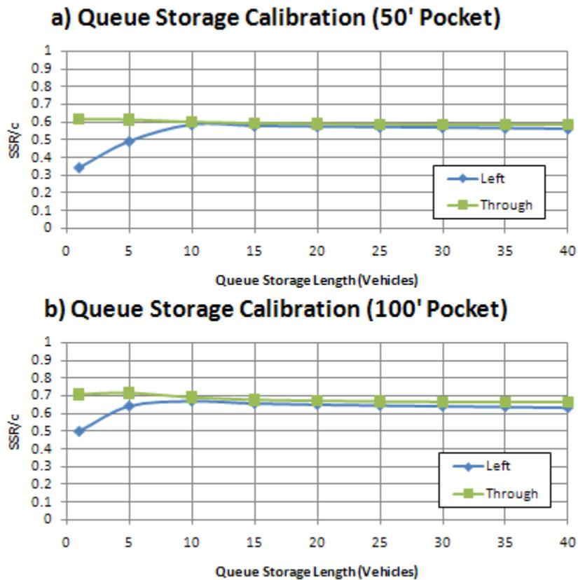
Figure 32 - Queue Storage Region Calibration for a 50' & 100' Pocket
