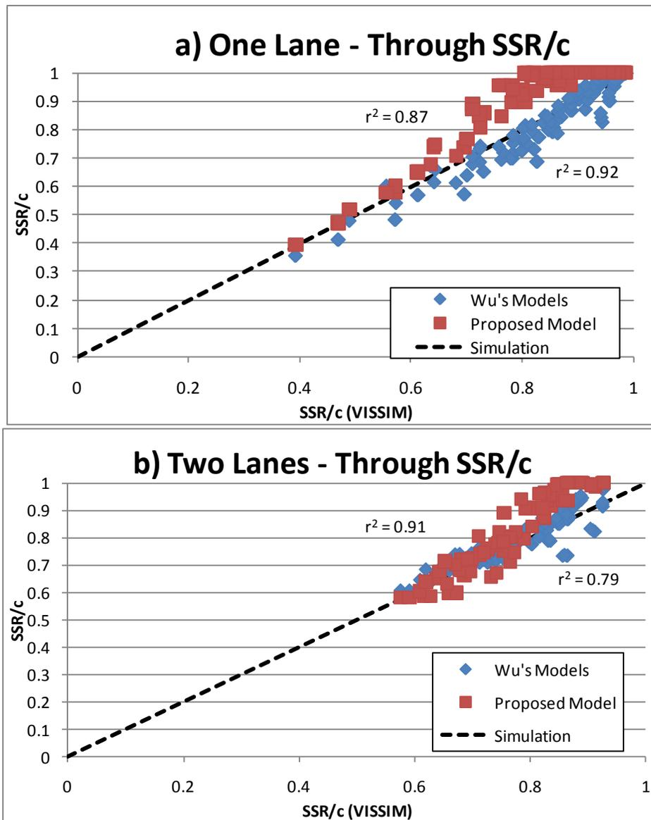
Figure 51 - SSR/c Model Comparison (Through)
