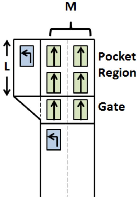
Figure 15 - Pocket Blockage:  $M \cdot n + M$  Through Vehicles
