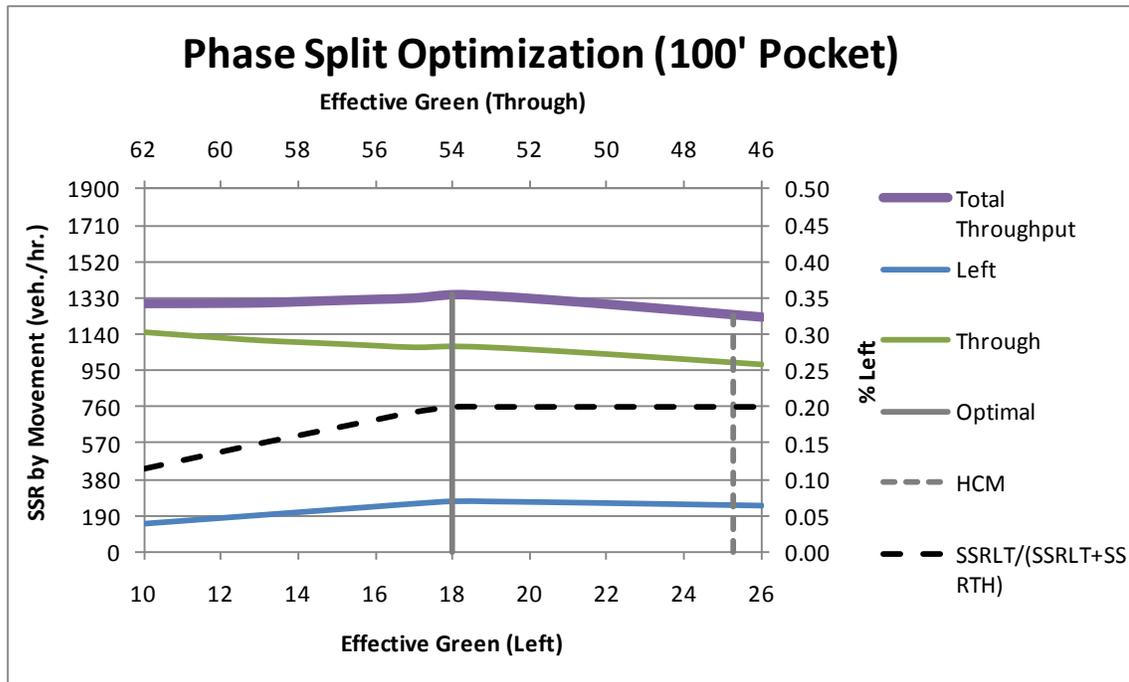
Figure 41 - Phase Split Optimization Procedure - 100' Pocket (SSR by Movement)
