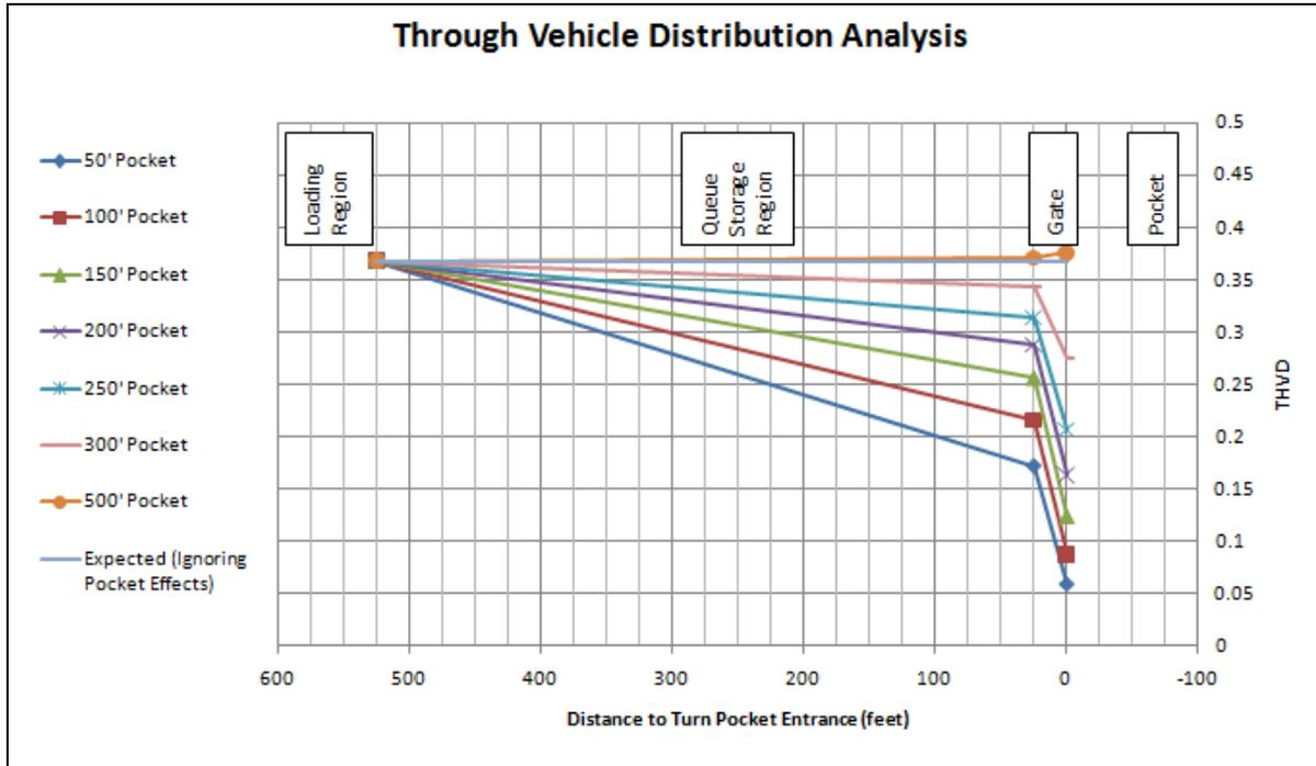
Figure 40 - Through Vehicle Lane Distribution by Distance
