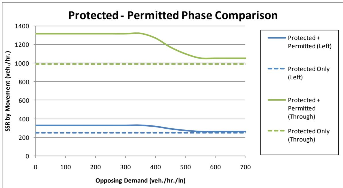
Figure 39 - Protected Only vs. Protected-Permitted Phase Sensitivity
