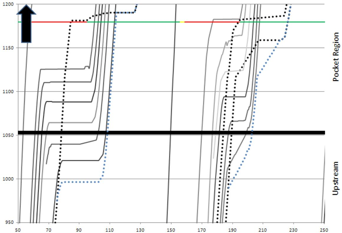
Figure 10 - Estimated Trajectories of Blocked Left-Turning Vehicles
