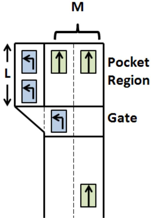
Figure 16 - Pocket Spillback:  $n+1$  Turning Vehicles
