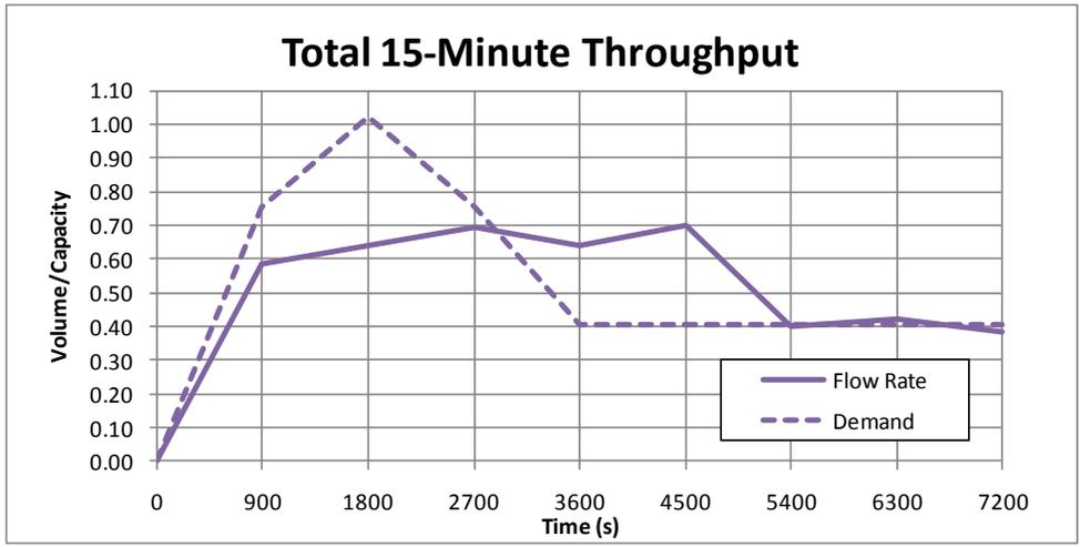
Figure 44 - Total Output with Time-Varying Demand (100' Pocket)
