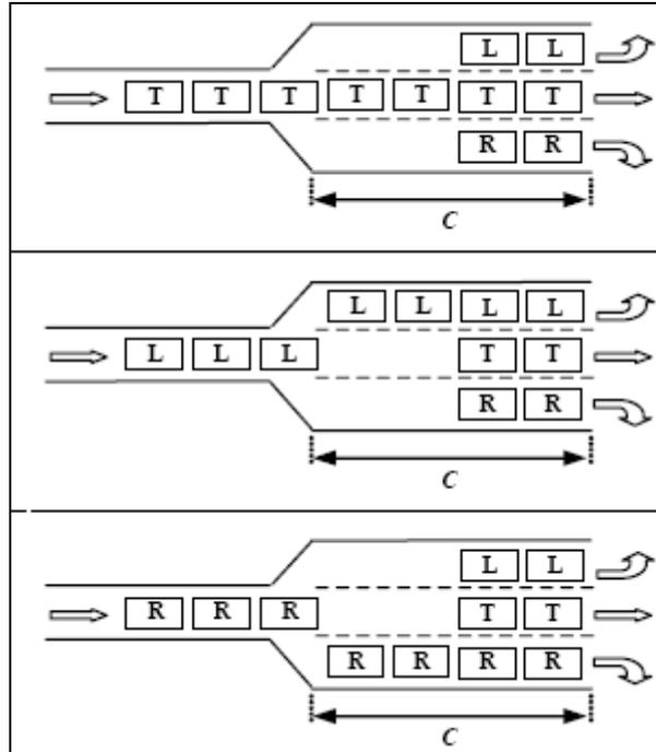
Figure 2 - Three-Branch Fork Example (Kikuchi, Kronprasert and Kii, 2007)
