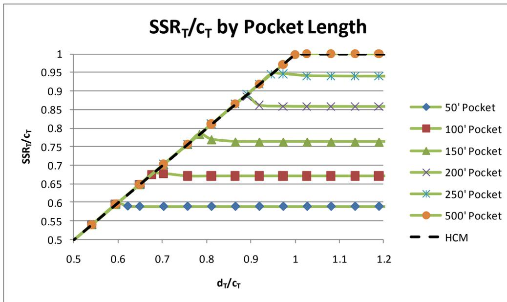
Figure 36 - Through Vehicle Throughput Demand Sensitivity
