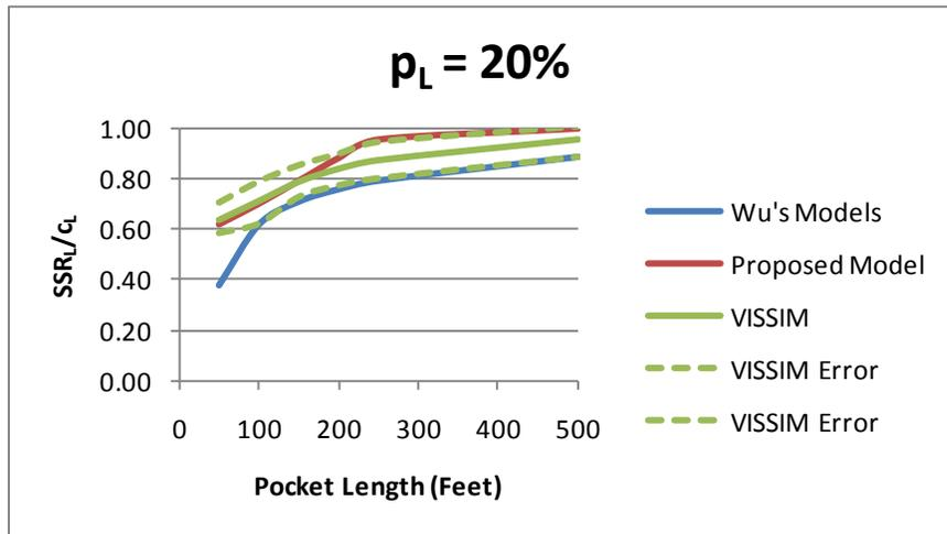
Figure 48 - Model Comparison (Left SSR with two approach lanes)
