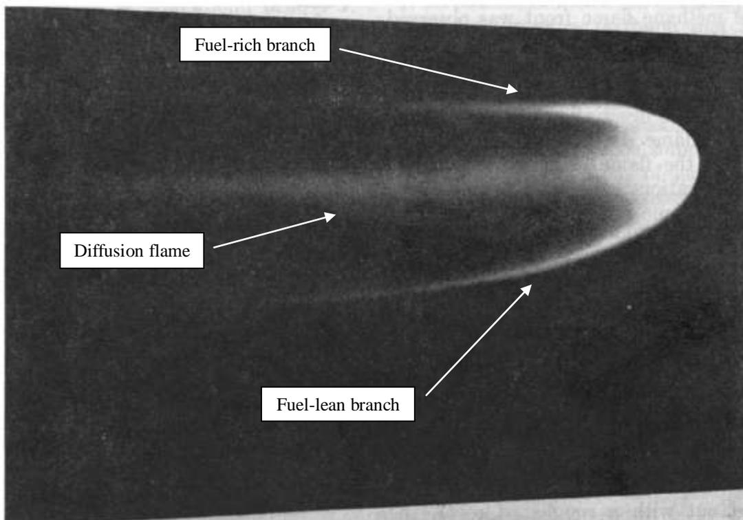
Figure 1.3 Image of a triple flame structure at the base of a lifted, laminar methane flame (Phillips, 1965).
