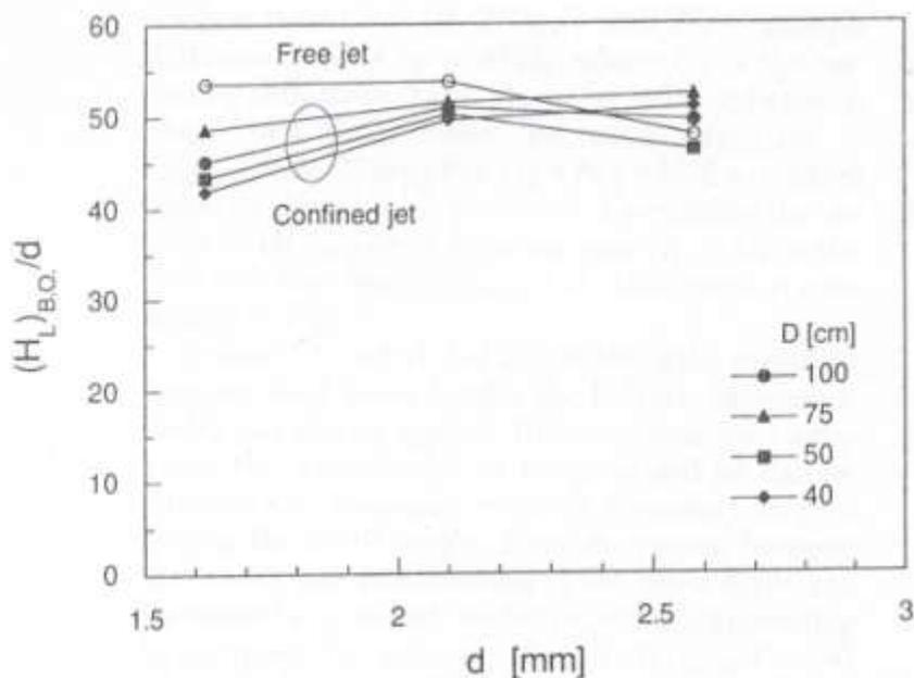
Figure 6.2 Lifted height at blowout,  $(H_L)_{B.O.}$ , nondimensionalized with the nozzle diameter,  $d$ , for free and confined jets (Cha and Chung, 1996).
