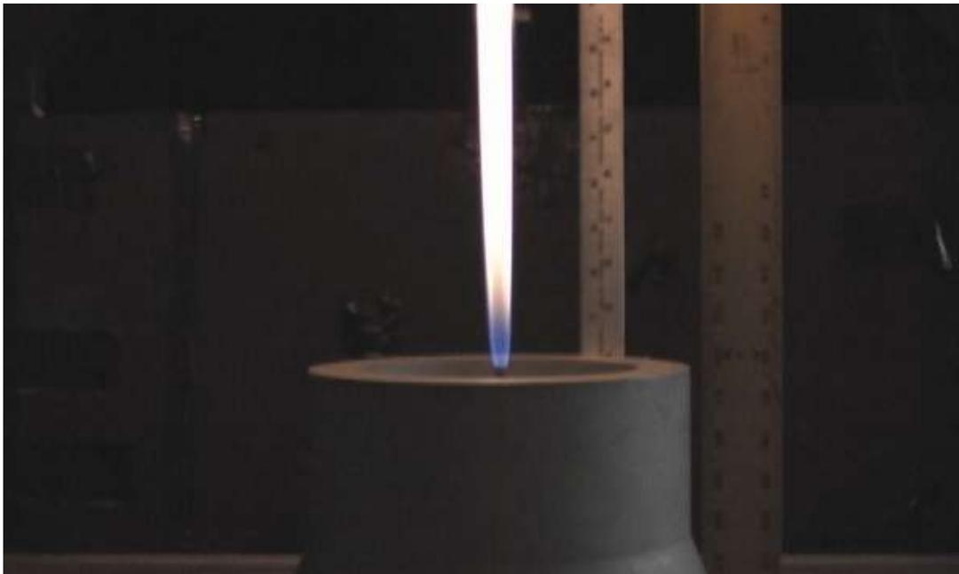
Figure 1.1 Image of a laminar methane flame.
