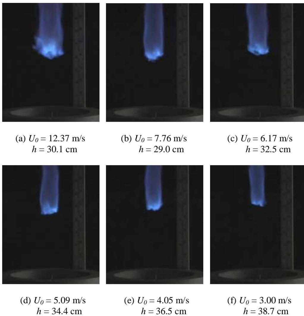
Figure 2.4 Sequence of images of a methane flame with co-flow velocity constant at 0.7 m/s.
