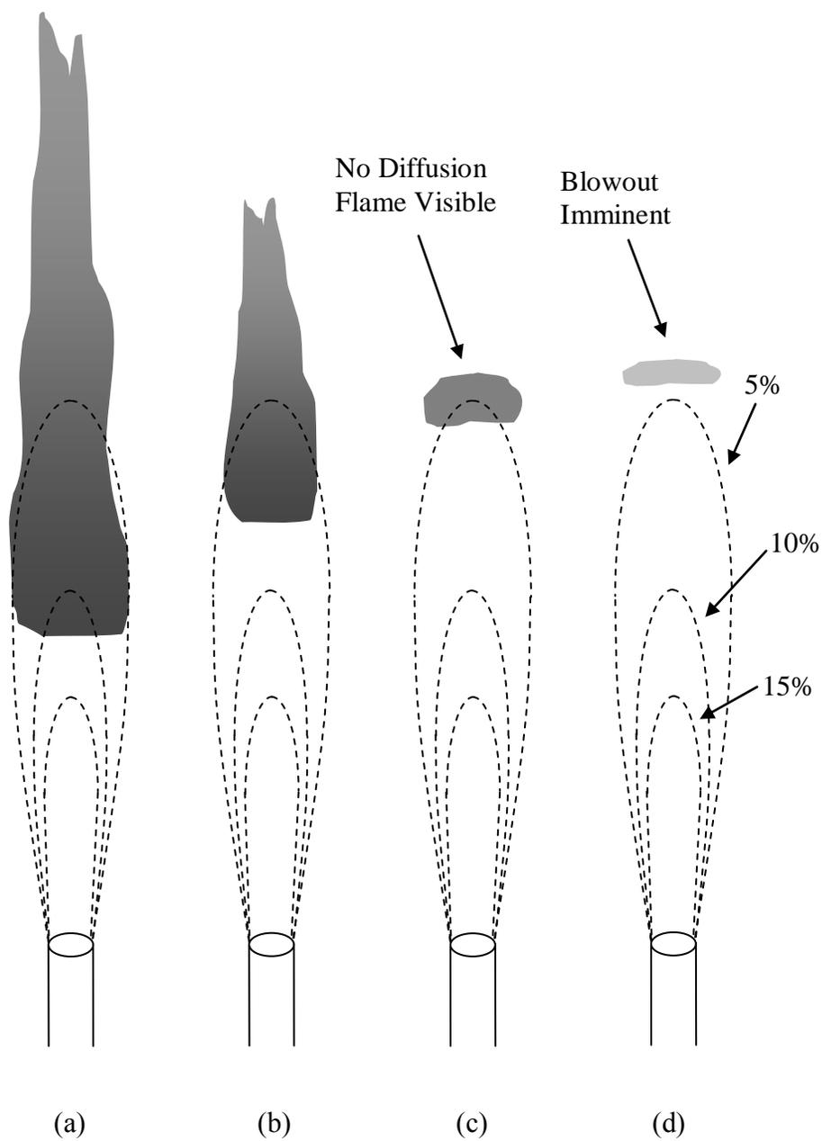
Figure 4.4 Schematic of the blowout mechanism relative to the flammability limits of methane. (a) A stable lifted flame. (b) The unstable flame has recessed downstream and the diffusion flame has shortened. (c) The diffusion flame has disappeared. (d) Blowout occurs.
