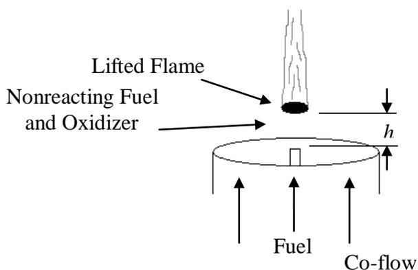
Figure 2.1 Methane is delivered from the pipe that is surrounded by co-flowing air.  $h$  is the distance from the pipe exit to the lifted flame front.
