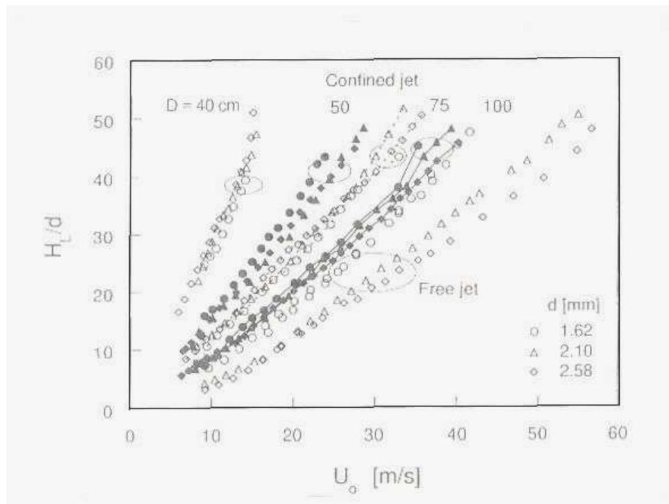
Figure 6.1. Lift-off height,  $H_L$ , nondimensionalized by the nozzle diameter,  $d$ , versus fuel velocity. The linear dependence with the free jet is not evident in the confined jets of various cylinder diameters (Cha and Chung, 1996).
