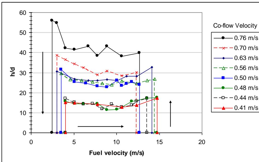
Figure 2.2 Flame position for various co-flow velocities. As indicated by the arrows, the fuel velocity was increased until the flame lifted and then incrementally decreased until reattachment. In each case, a change in the direction of movement of the flame is observed even though the fuel velocity is being decreased.
