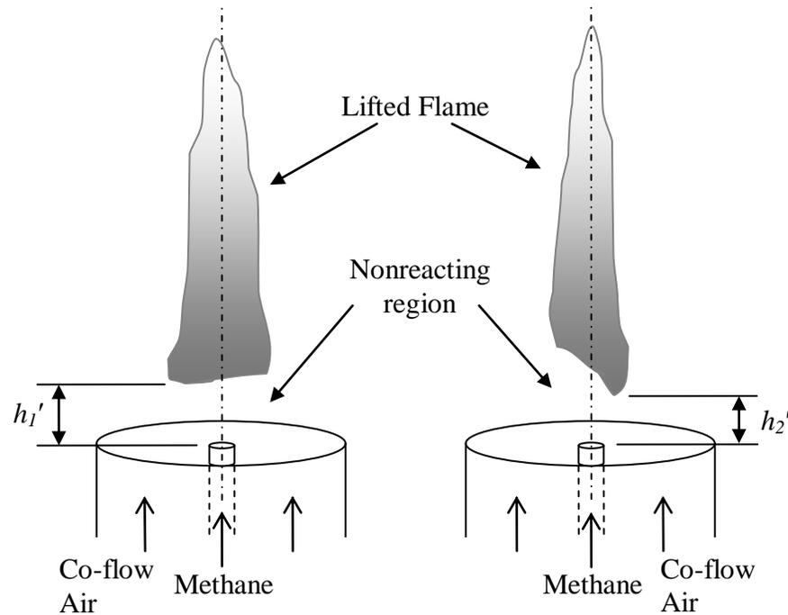
Figure 3.1 Two examples of a lifted methane flame. The fuel is delivered from a pipe that is surrounded by co-flowing air.  $h'$  is the instantaneous axial distance from the fuel exit to the lifted flame base.
