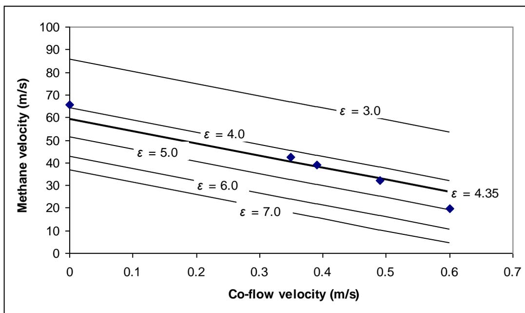
Figure 5.4 Velocities required for blowout shown with  $\varepsilon$  contours.
