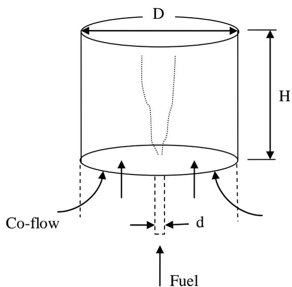
Figure 6.3 Schematic of Confining Cylinder.  $d$  is the fuel nozzle diameter,  $D$  is the cylinder diameter, and  $H$  is the cylinder height.
