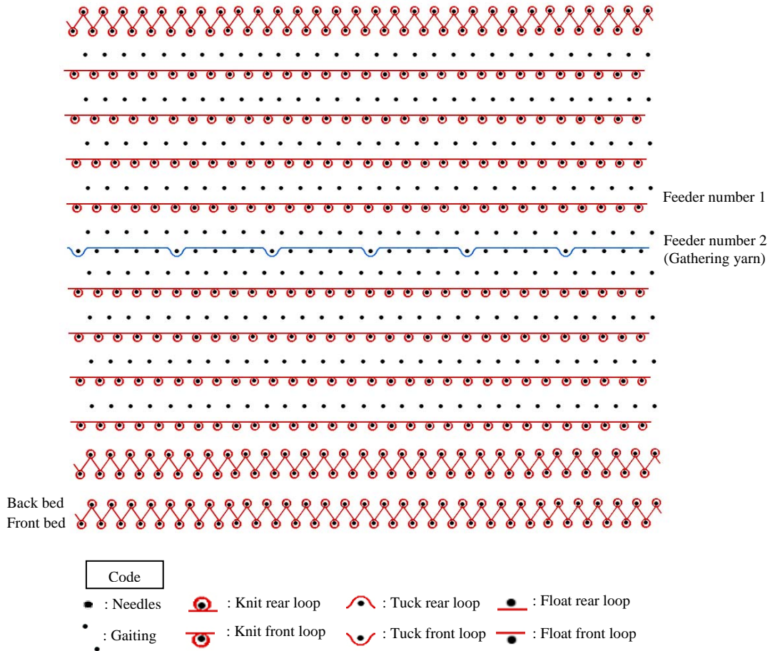
Figure 4.34 Loop notation to create pleated knit structures by the use of held loop structures.
