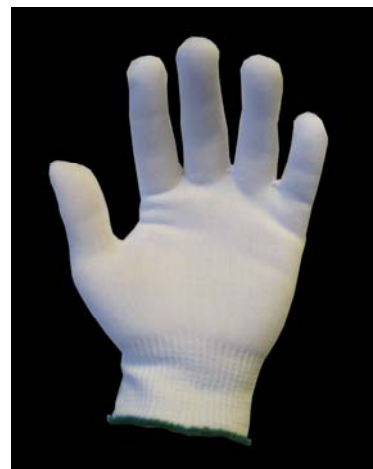
Figure 2.10 A seamless glove created on the Shima Seiki machine at Polygenex Inc. (2004).
