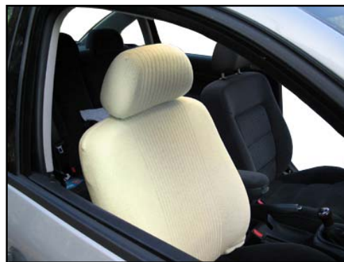
Figure 2.24 Auto seat cover knitted in a tubular form with a 2X2 rib structure on the Shima Seiki SWG-V™ machine.
