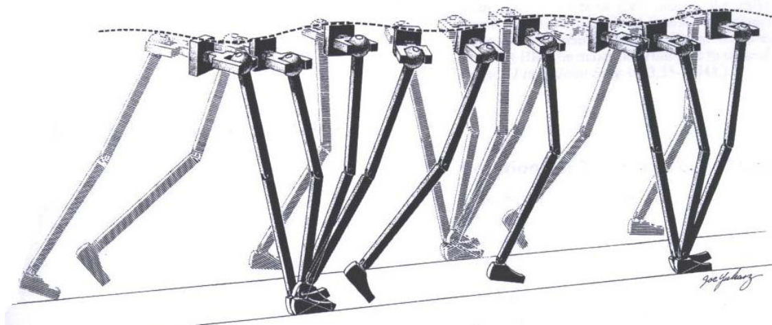
Figure 3 The sum of the effects of several determinants is a sinusoidal curve of low amplitude (Saunders 1953, Rose and Gamble 2006)
