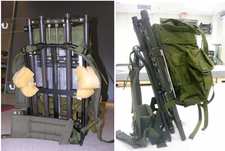
Figure 20 Left: Front view of the suspended-load backpack. Right: Side view of the suspended-load backpack.
