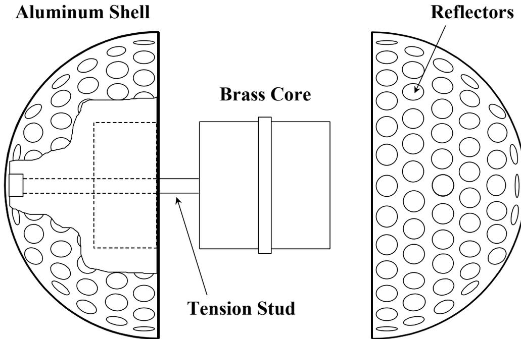
Figure 2.3 Notional schematic of the Lageos satellite structure
