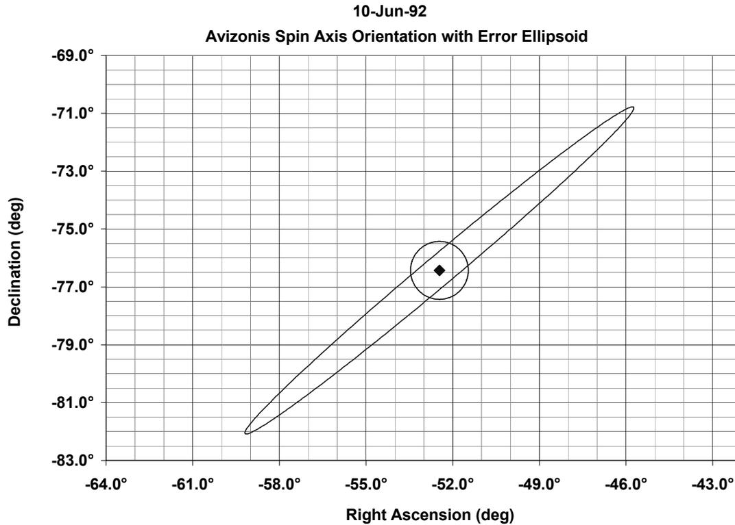
**Figure 4.1** Sample Avizonis Lageos spin axis orientation solution with corresponding error ellipsoid. The spatial orientation for the Lageos satellite spin state on June 10, 1992 is shown (centered diamond) with the corresponding  $1\sigma$  error ellipsoid superposed. The solution was determined by Avizonis from optical flash data. A unit sphere is also illustrated to provide a spatial benchmark.
