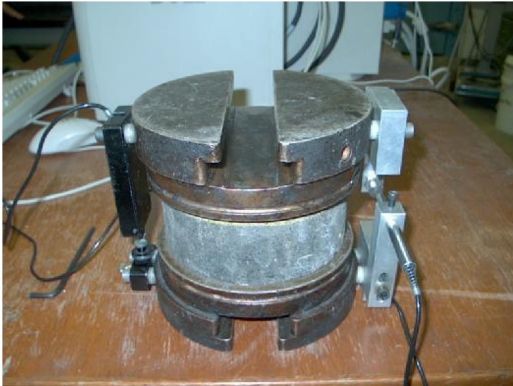
Figure 5.3 Simple Shear (FSTCH and RSTCH) Test Specimen
