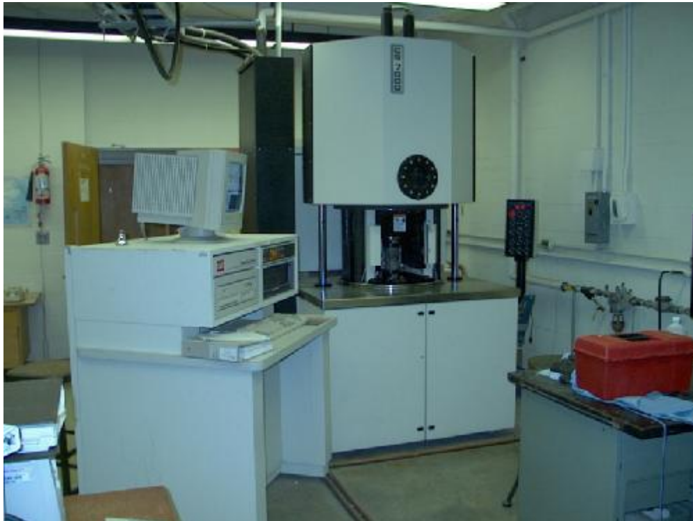
Figure 5.2 SUPERPAVE Simple Shear Tester (SST)
