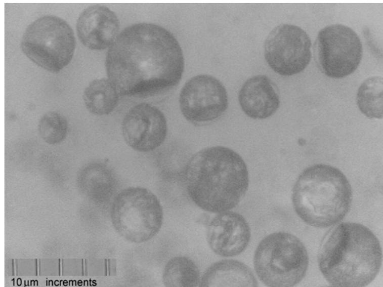
**Figure 3-2 MicroPCM slurry**
