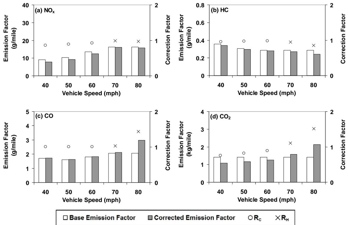
**Figure 4-5. Comparison of Base Emission Factors from MOBILE6 versus Corrected Emission Factors based on Constant and High Speed Correction Factors (R<sub>C</sub> and R<sub>H</sub>).**
