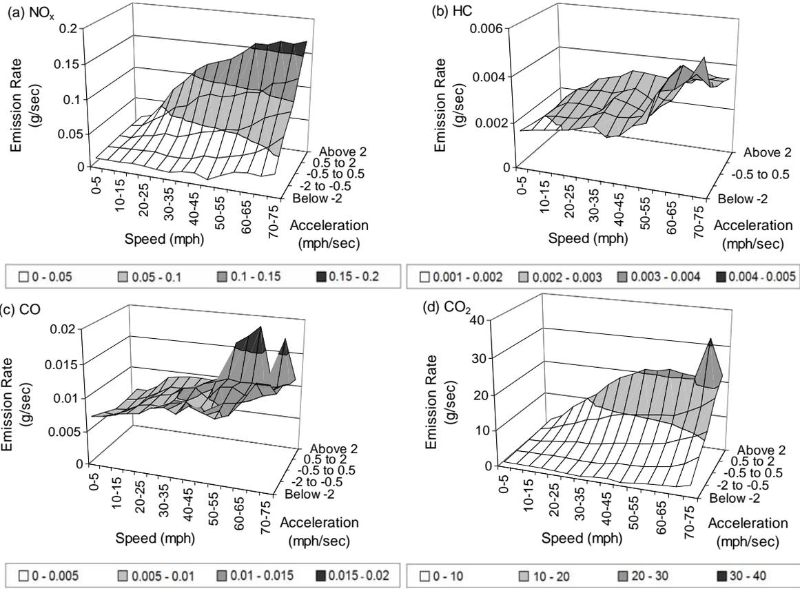
**Figure 4-2. Speed-Acceleration Matrix Profiles for Average Emission Rates based on 62,419 Seconds of Data for 5 Diesel Vehicles.**
