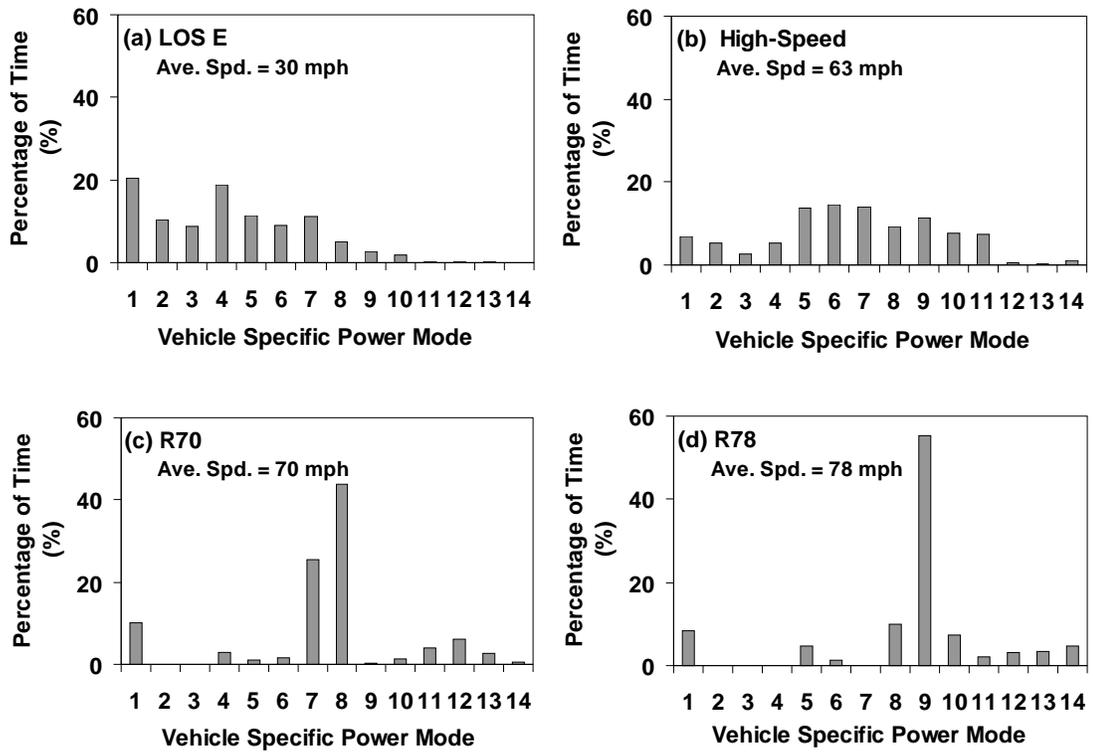
**Figure 3-2. Time Distribution of VSP Modes for LOS E, High-Speed, R70, and R78 Cycles.**
