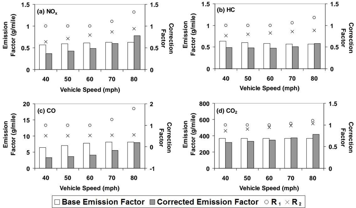
**Figure 3-6. Comparison of Base Emission Factors from MOBILE6 versus Corrected Emission Factors based on High Transient and Constant Speed Correction Factors ( $R_1$  and  $R_2$ ).**
