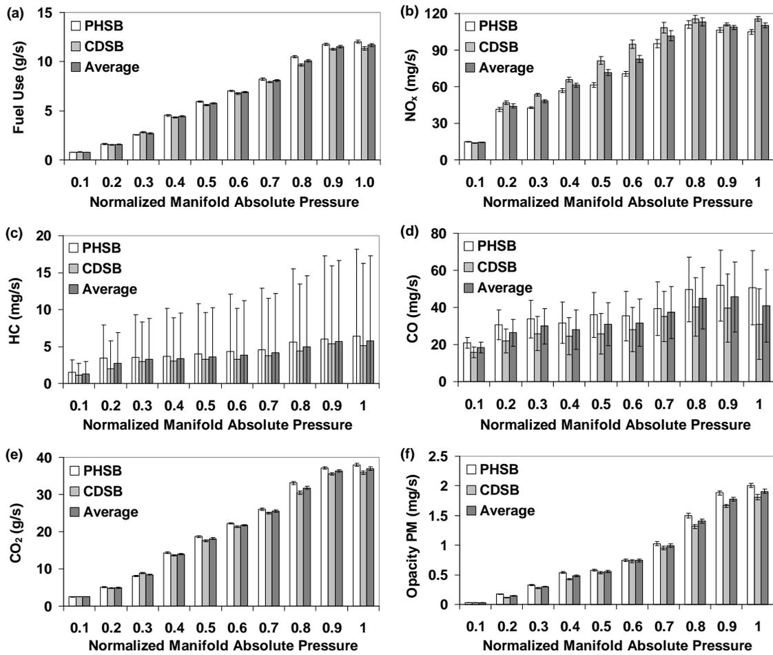
**Figure 6-1. Average fuel use rate and emission rates for each manifold absolute pressure mode for VT365 engine.** Note: PHSB = Plug-in Hybrid School Bus. CDSB = Conventional Diesel School Bus. Ranges shown are 95 percent confidential Intervals on mean values.
