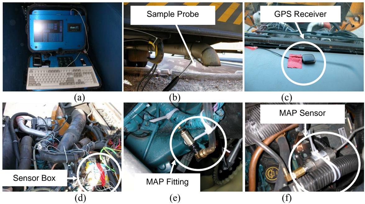
**Figure C-3. Installation of the Portable Emissions Measurement System (PEMS).** (a) the portable unit on a bus seat (front-view); (b) sampling exhaust gases using a probe secured with a hose clam; (c) GPS receiver on the dashboard; (d) sensor box; (e) Manifold Absolute Pressure (MAP) Fitting; and (f) Manifold Absolute Pressure (MAP) Sensor
