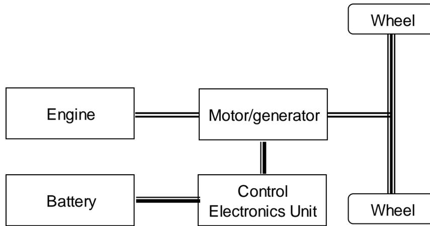
**Figure C-1. Power Flow for Parallel Plug-In Hybrid Electric Vehicle.**
