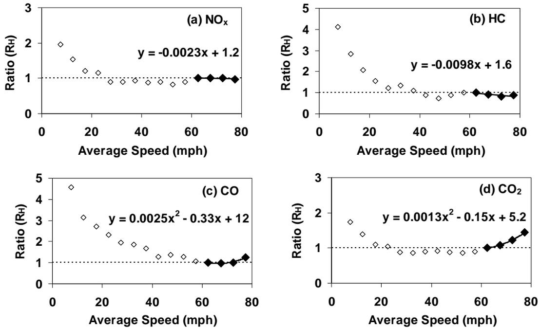
**Figure 4-4. High Constant Speed Correction Factors ( $R_H$ ) based on Ratio of Distance-based Emission Factors to Emission Factors at 63 mph during Cruise.**
