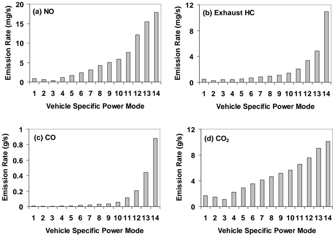
**Figure 3-1. VSP Modal Tailpipe Emission Rates for NO, Exhaust HC, CO, and CO<sub>2</sub> for Vehicles with Engine Sizes less than 3.5 Liters and Mileage Accumulation less than 50,000 Miles (Frey et al., 2002).**
