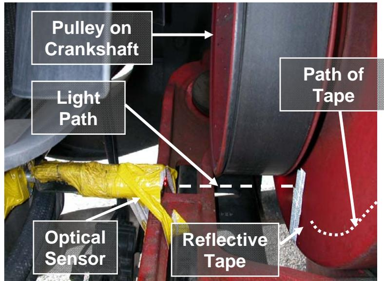
**Figure 2-2. Example Photo of Placement of Optical Engine RPM Sensor and Reflective Tape (Cummins ISX-500 Engine).**
