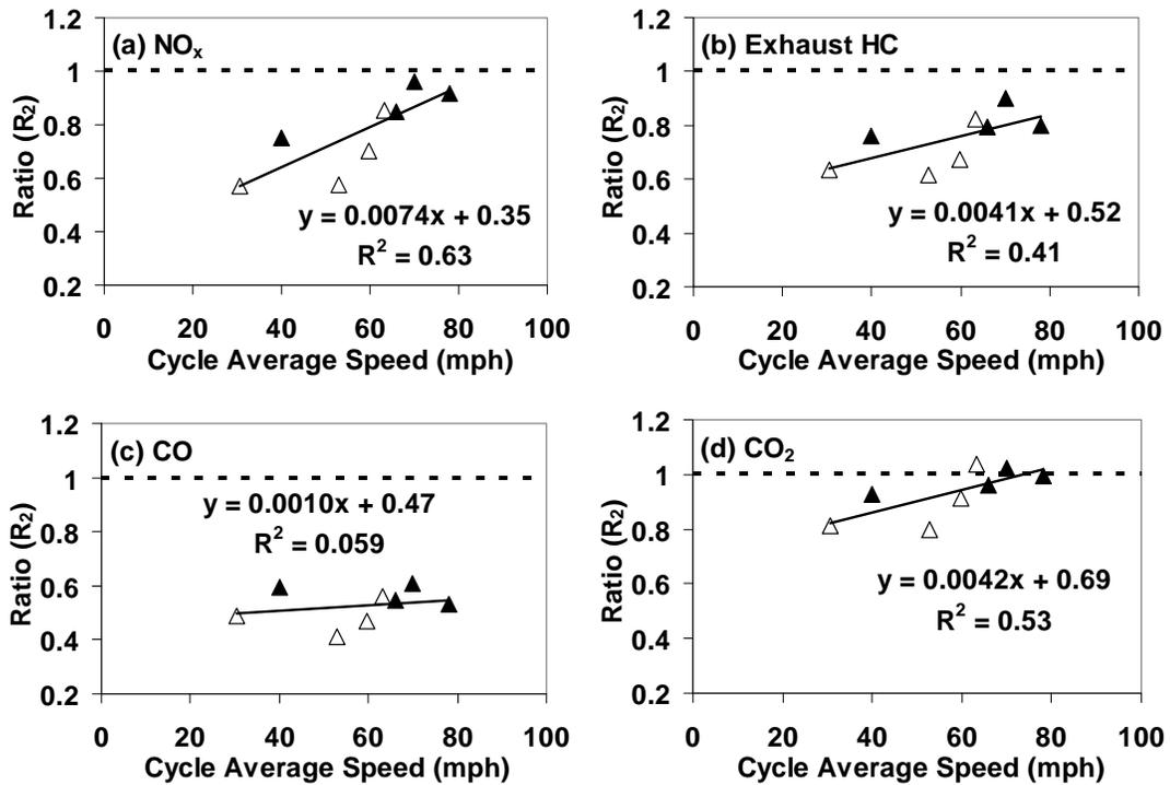
**Figure 3-5. Constant Speed Correction Factors ( $R_2$ ) based on Average Ratio of Constant Speed Emission Factors to Cycle Average Emission Factors for the Same Driving Cycle Speed using VSP-Modal Model for LDGV.** Note: Blank triangles are EPA facility-specific cycles and dark triangles are real-world cycles.
