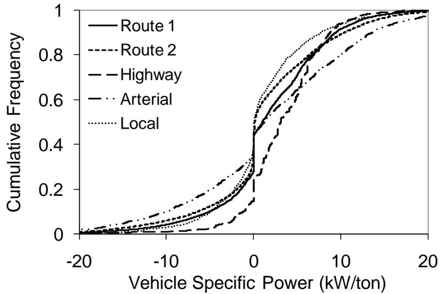
**Figure C-4. Vehicle Specific Power Distributions for each Route.** Note: Routes 1 and 2 are actual school bus routes for the hybrid bus and control bus, respectively. Highway cycle is based on the highway portion of Route 1. Arterial and Local cycles are based on the arterial and local portions of Route 2, respectively.
