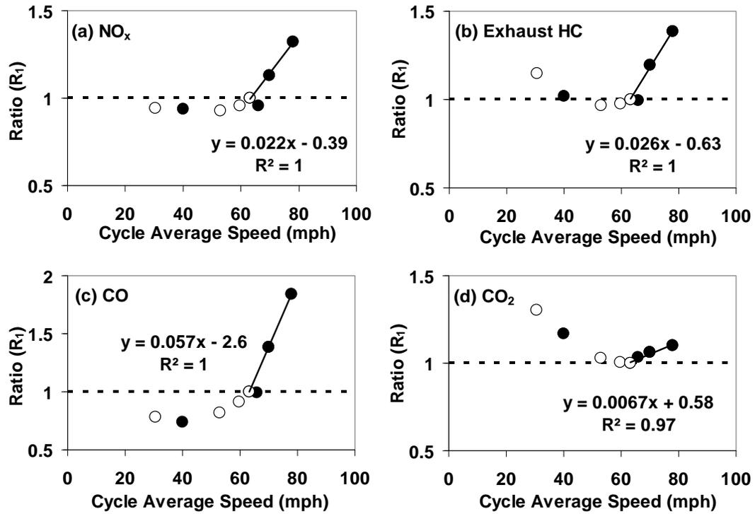
**Figure 3-4. High Speed Correction Factors ( $R_1$ ) based on Ratio of Cycle Emission Factors to High-Speed Cycle Average Emission Factors using VSP-Modal Model for Exhaust Emissions for LDGV. Note: Blank circles are EPA facility-specific cycles and dark circles are real-world cycles.**
