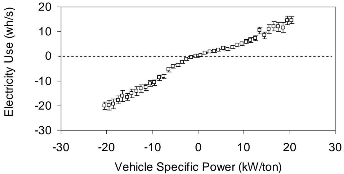
**Figure 6-3. Electricity Use Rate versus Vehicle Specific Power.** Note: Positive electricity use = discharge. Negative electricity use = recharge. Net fuel use for hybrid bus includes engine fuel use and equivalent fuel use for electricity use. Ranges shown are 95 percent confidential Intervals on mean values.
