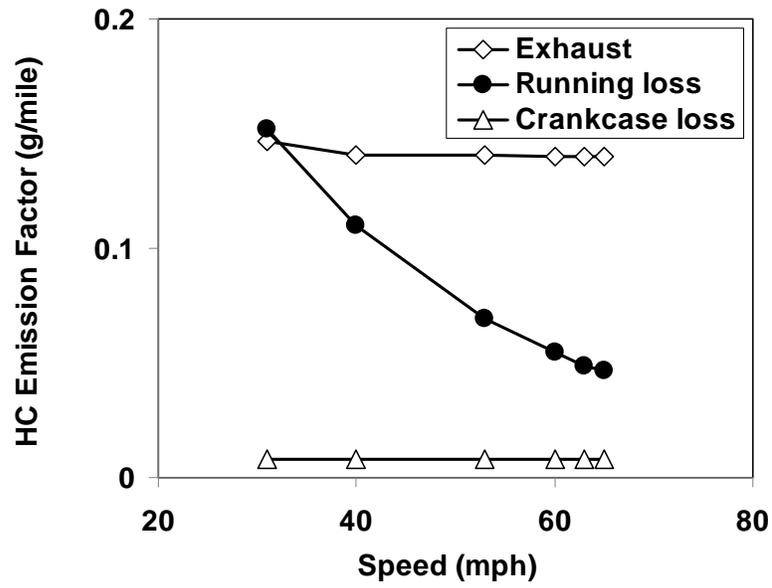
**Figure 3-3. HC Emission Factors (g/mile) for Exhaust and Non-exhaust Emissions under Base Case Conditions for Light Duty Gasoline Vehicle.** Note: The base case condition is temperature = 81°F, relative humidity = 76%, and barometric pressure = 29.6 inches Hg.
