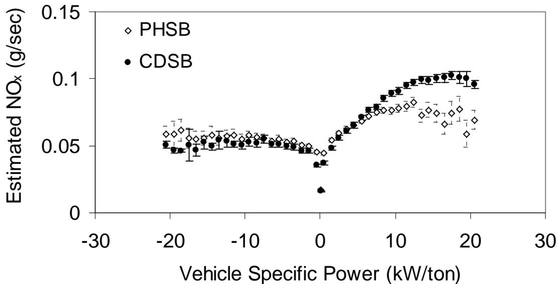
(b) NO<sub>x</sub> emission rates versus Vehicle Specific Power
