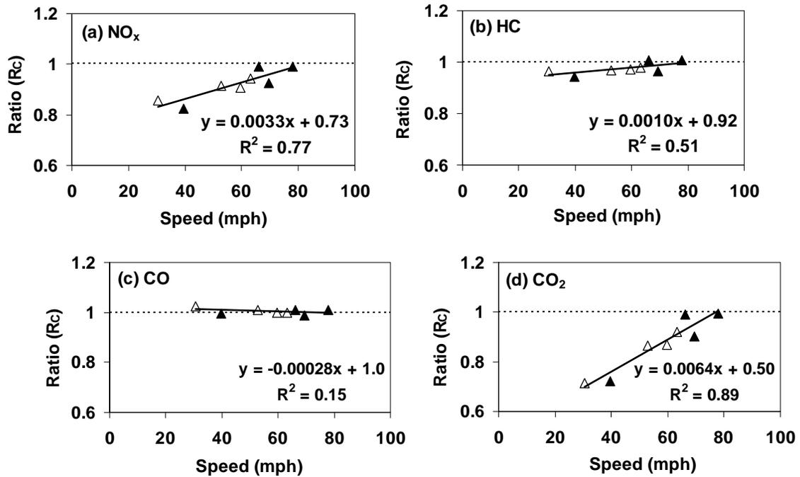
**Figure 4-3. Constant Speed Correction Factors (RC) based on Ratio of Constant Speed Emission Factor to Cycle Average Emission Factors for the Same Driving Cycle Speed on a Distance Basis.** Note: Blank triangles are EPA facility-specific driving cycles and dark triangles are real-world driving cycles.
