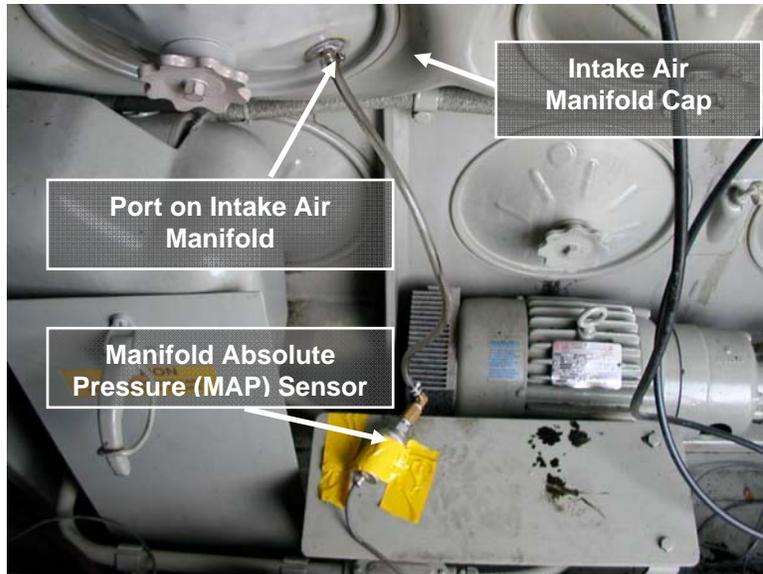
**Figure 2-1. Placement of the Manifold Absolute Pressure Sensor on the EMD 12-710G3 Engine of the F59 Locomotive (NC1755)**
