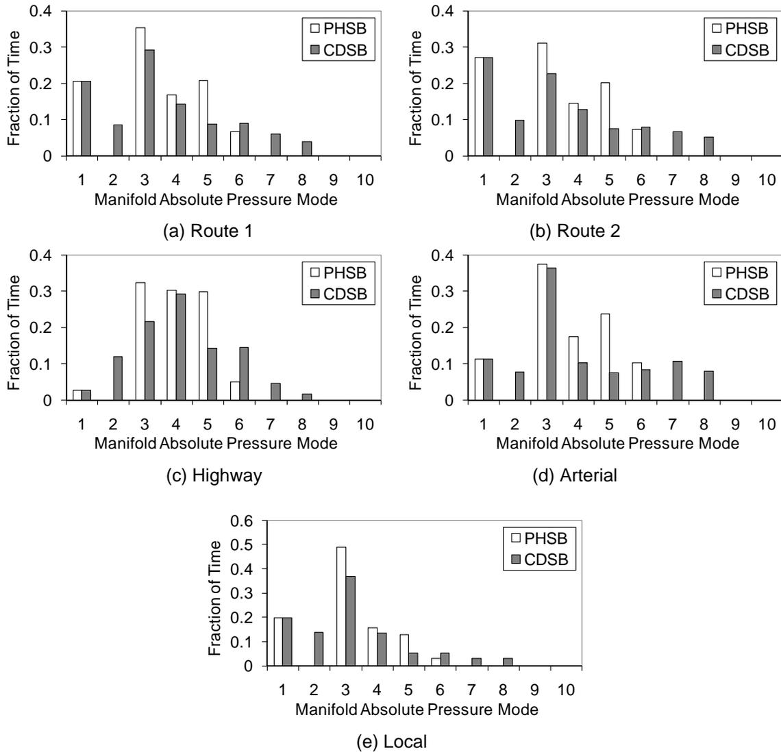
**Figure C-5. Estimated manifold absolute pressure (MAP) distributions for each route based on relationship for measured MAP versus vehicle specific power.**
