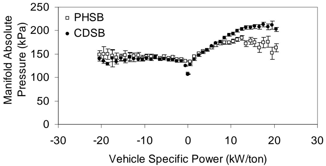
**Figure 6-2. Measured Manifold Absolute Pressure versus Vehicle Specific Power.**
