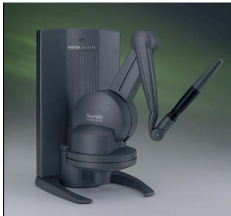
Figure 3.3. The PHANToM desktop device from SensAble Technologies, Inc.
