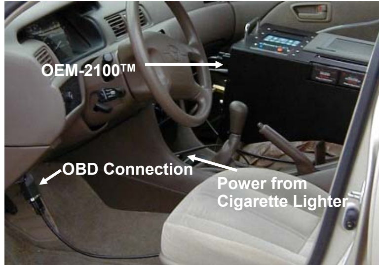
FIGURE 1. OEM-2100™ installed in a 1998 Toyota Camry
