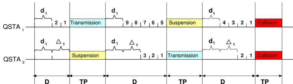
Figure 2.1: EDCA Channel States with Two stations ( $d_1 = 2, d_2 = 4$ ).
