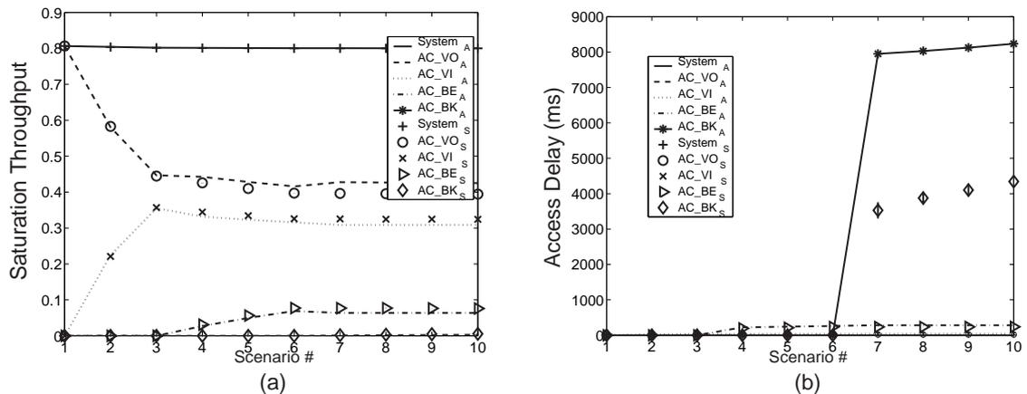
Figure 2.6: Experiment 1: Performance Using Default EDCA Parameter Set
