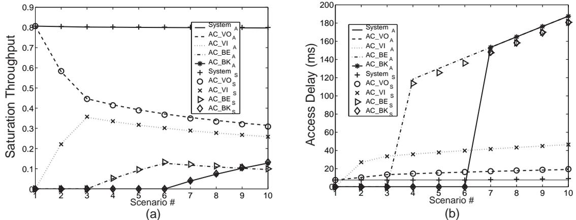
Figure 2.8: Experiment 3: Performance by Varying Only CW
