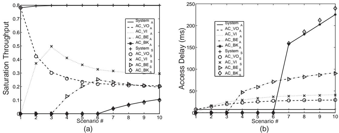
Figure 2.7: Experiment 2: Performance by Varying Only AIFS
