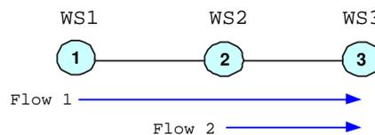
Figure 4.12: Network Model of Case Study III: an small ad-hoc Wi-Fi network.
