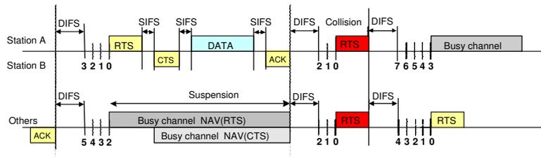
Figure 1.1: DCF Access Procedure.
