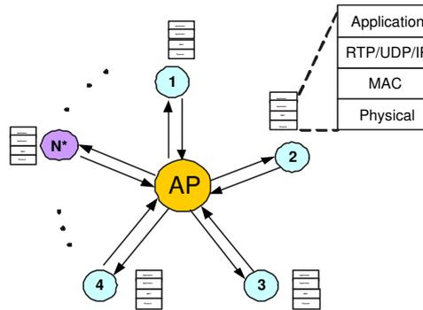
Figure 4.8: Network Model of Case Study II: an infrastructure Wi-Fi network with VoIP Traffic.
