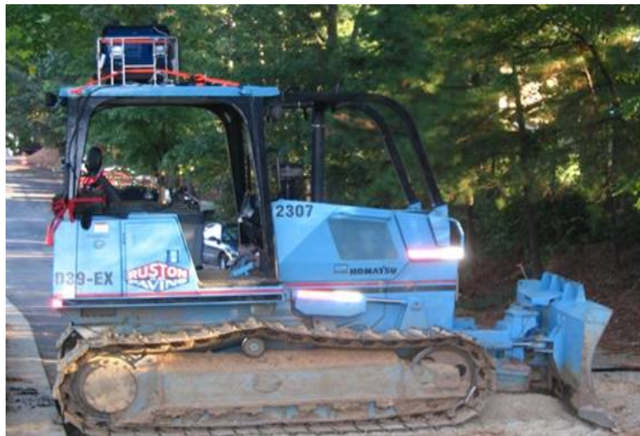
Figure 3.2 PEMS Installed on Bulldozer
