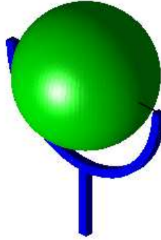
Figure 3.5: The flat double gimbal. An example of the "flat" double gimbal system is constructed by mounting a uniform, spherically symmetric body (denoted J ) to the outer gimbal. Since the ratio J_z/J_x equals 1, the mass matrix of (3.14) becomes angle independent and thus the "flat" gimbal inherits its flatness from an angle independent kinetic energy metric. The angle independent metric of the flat gimbal has the effect of decoupling the inner and outer gimbal free motions (see Figure 3.7). Since it is geometrically straight forward to analyze, the flat double gimbal gives an intuitive and simple example into not only the behavior but also the control of more difficult (meaning "non-flat" or coupled) double gimbal systems.
