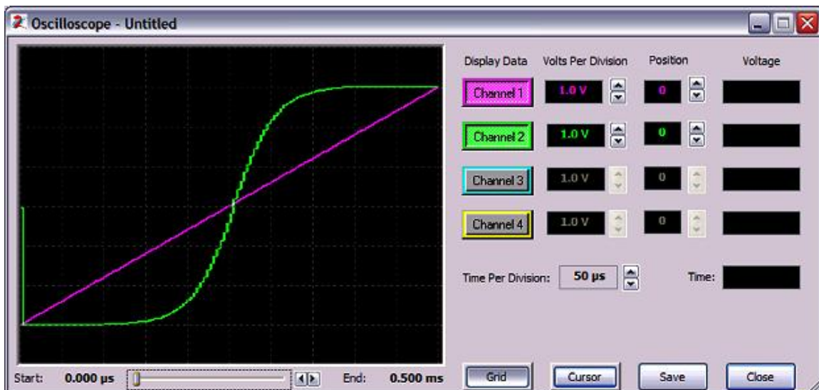
Figure 2.11. Simulation result of hyperbolic tangent transfer function.
