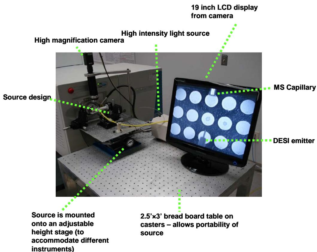
**Figure 2.5** The contemporary DESI source design used in the Muddiman laboratory. heights. The large area of the table top allows for permanent placement of the high magnification camera (Part Number KP-M1AN, Hitachi), light source (Part Number MI-150; Dolan Jenner), 19" LCD monitor (Staples Inc) and provides ample space for future modifications. The LCD monitor provides for visualization of both the position of the ESI emitter and sample spot, critical in obtaining optimal results.
