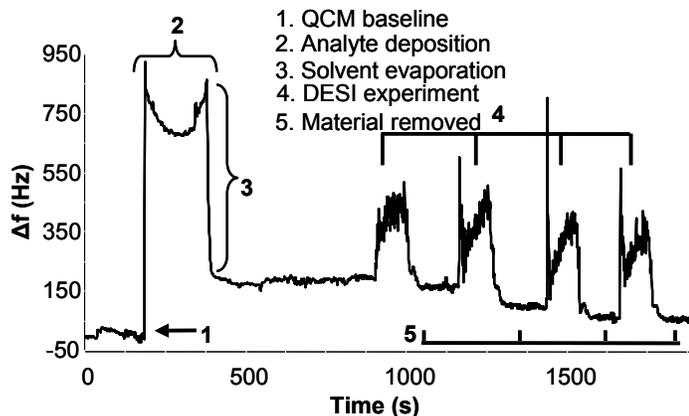
**Figure 3.8** A real time plot relating QCM response to analyte deposition and DESI-MS analysis.
