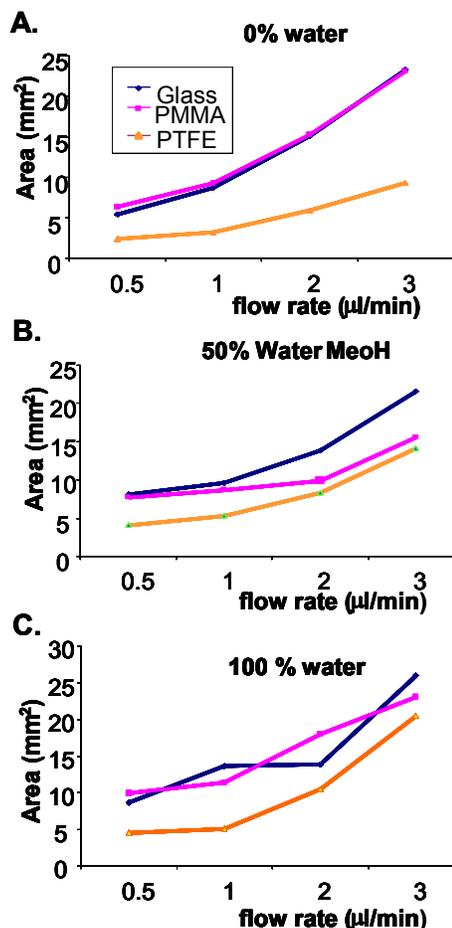
**Figure 3.2** DESI spot size as a function of flow rate, solvent composition, and surface type.
