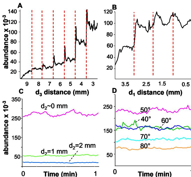
**Figure 3.3** The dependence of ion abundance on several geometric parameters.
