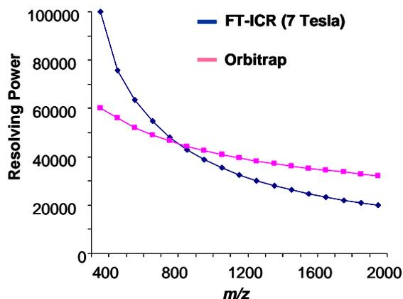
**Figure 1.3** Resolving power as a function of  $m/z$  for two different FTMS based instruments.
