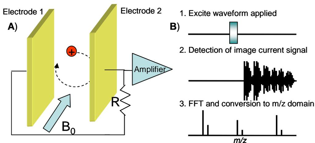
**Figure 1.1** A) Schematic of an ICR cell B) Overview of excite, detect and FFT processes.
