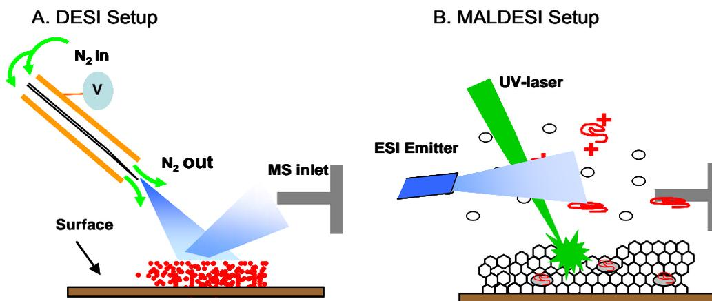
**Figure 2.1** A schematic representation of both a typical (A) DESI and (B) MALDESI setup.
