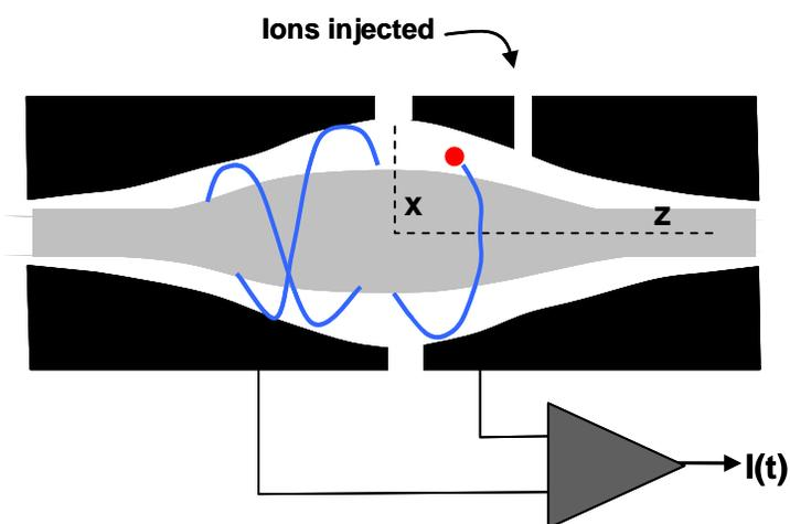
**Figure 1.2.** The static electric field created by the specially designed electrodes trap ions in a 3 dimensional space. There are three different frequencies that can be measured and used for mass analysis; however, the frequency in the z direction is the only frequency that
