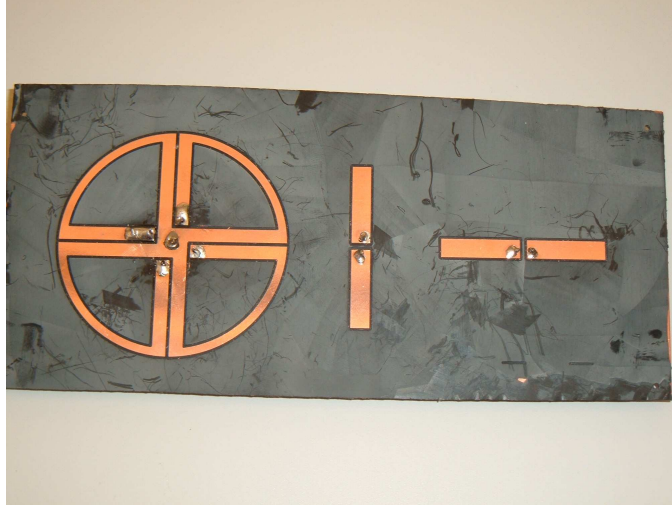
Figure 5.1: Fabricated narrow band distributed vector antenna consisting of a loop and two dipoles
