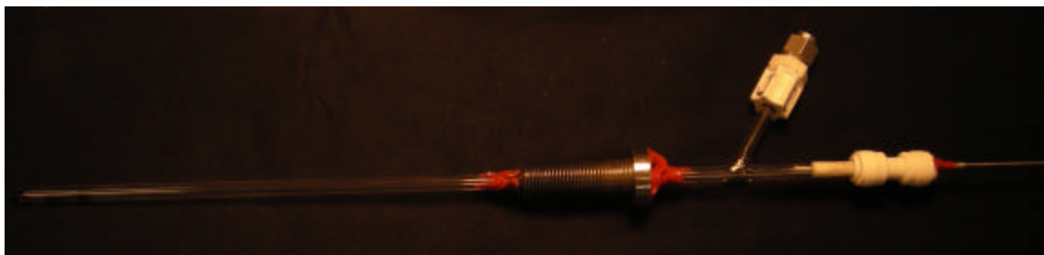
Figure 6.1: Final quartz microprobe design
