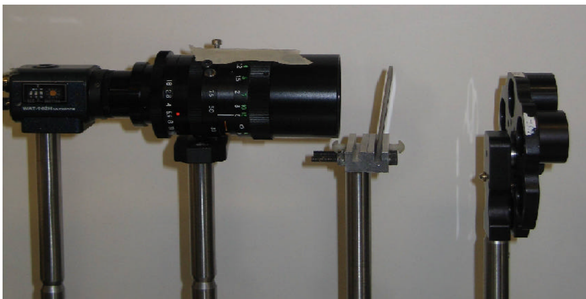
Figure 5.1:Watec 902 Ultimate monochrome CCD camera with ND filter and color filter wheel
