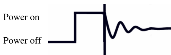
Figure 16. Simple one pulse NMR experiment followed by FID acquisition. The section to the left of the vertical line indicates the period during which the radiofrequency pulse is applied; and the section to the right indicates the oscillating signal detected from the sample during acquisition. The vertical line indicates the point at which the radiofrequency pulse is shut off, and the coil switches modes from transmitter to receiver.
