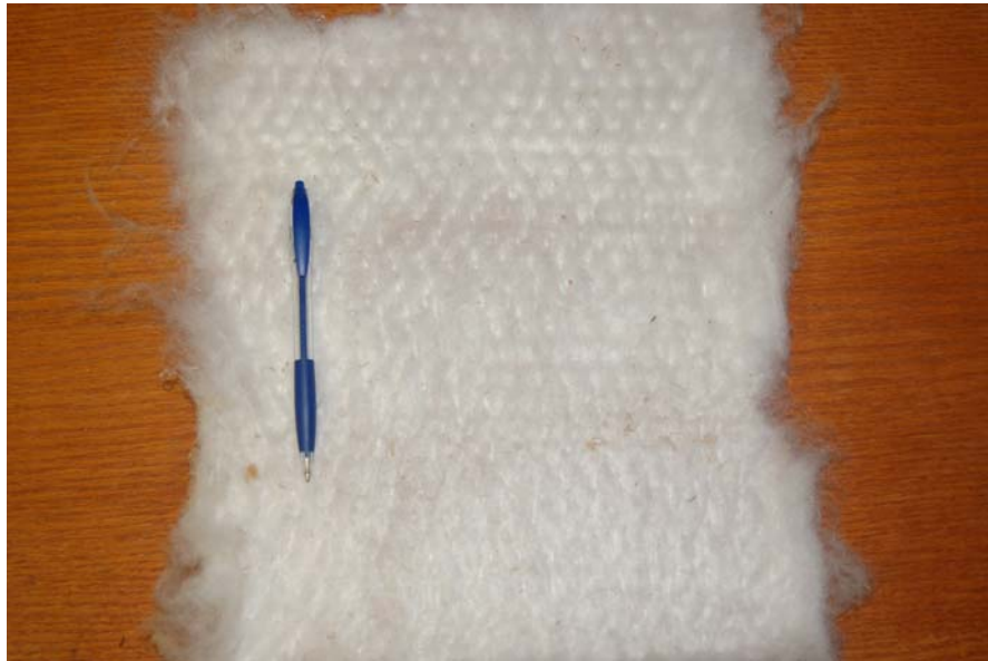
Figure 1.10: Wood-polyester fiber panels manufactured during initial phases of the project.
