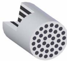
Figure 1.5c: Islands-in-the-sea bicomponent fiber
