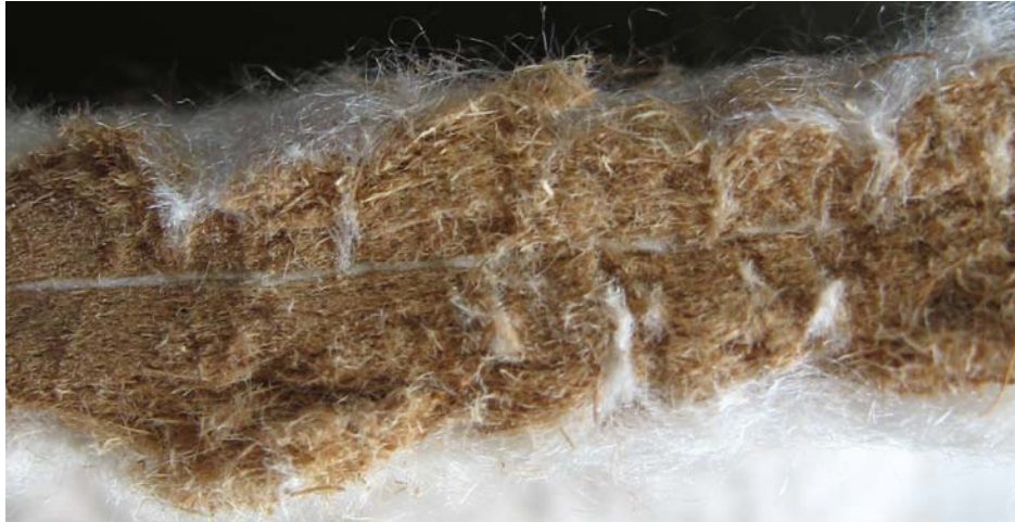
Figure 1.14a: Unconsolidated 4.3 mm half punched wood-bicomponent fiber panel.
