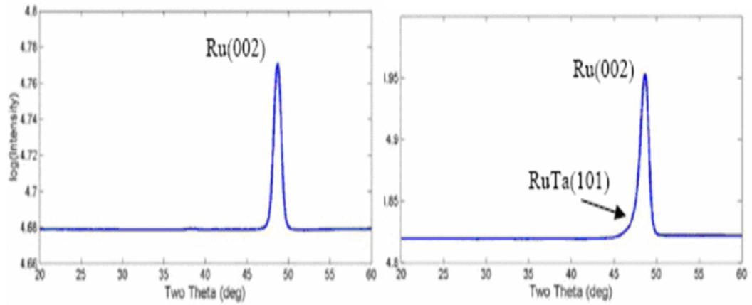
Figure 4. 14 The in-situ XRD data of 500A Ru / 100A Ta / SiO<sub>2</sub> (a) As-deposited (b) after 1100°C anneal
