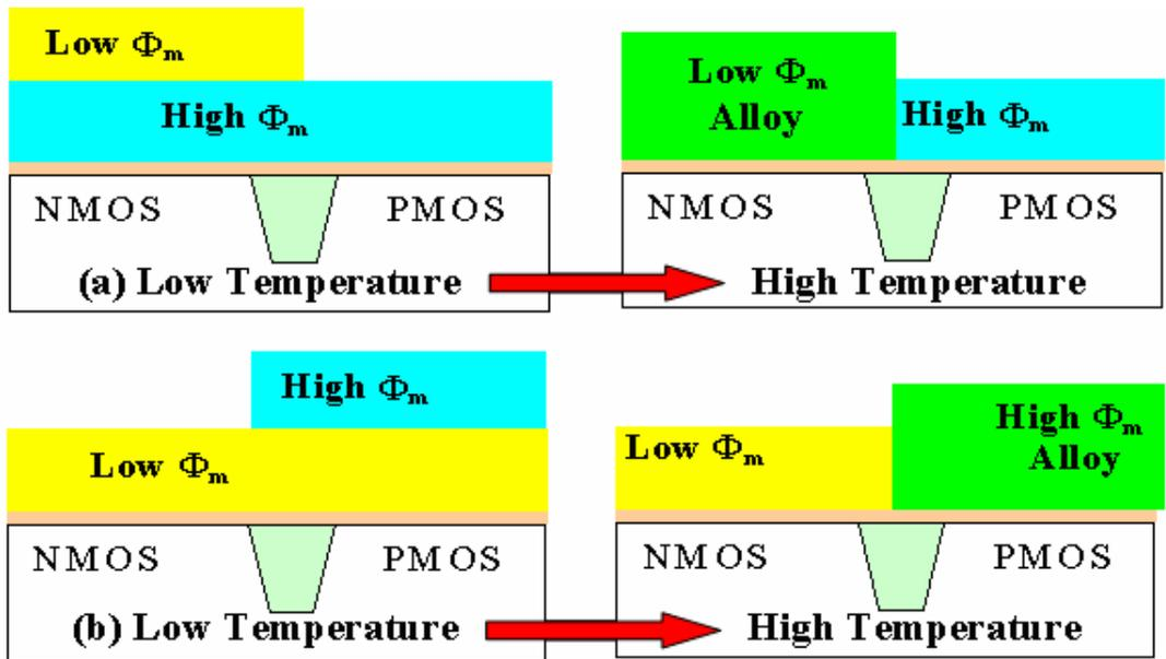
Figure 4. 1 Integration approach for dual metal gate CMOS
