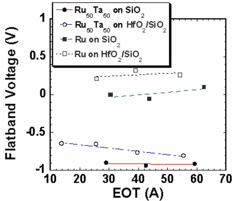
Figure 2. 15 V<sub>FB</sub> vs. EOT for Ru and Ru-Ta alloy on SiO<sub>2</sub> and HfO<sub>2</sub>/SiO<sub>2</sub>. The stacks have varying SiO<sub>2</sub> with fixed HfO<sub>2</sub> thickness. Since similar separation is observed this indicates that Fermi Level pinning is not occurring.
