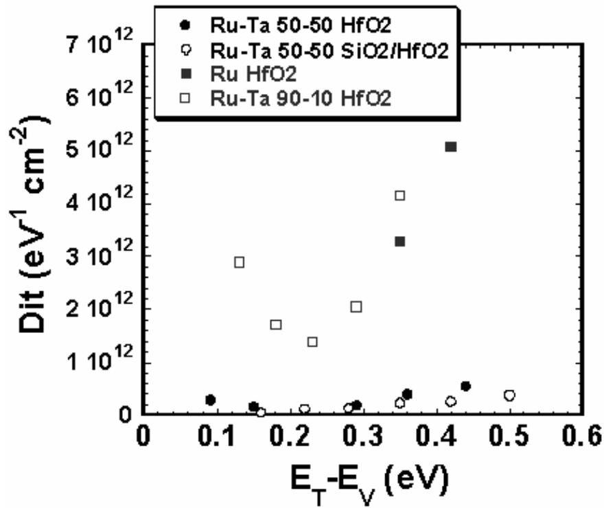
Figure 2. 10 Interface State Densities of HfO<sub>2</sub> via conductance method for selected gate electrodes.
