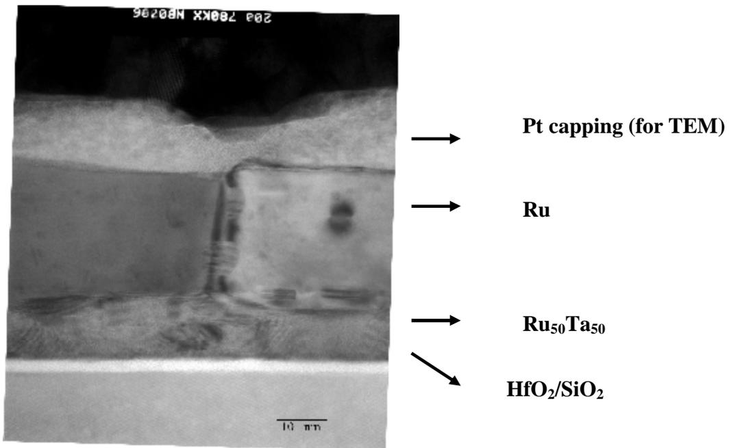
Figure 5. 9 TEM image of Ru 500A gates with underlayer of Ru<sub>50</sub>Ta<sub>50</sub> 100A on HfO<sub>2</sub>/SiO<sub>2</sub> after annealing at 800°C in 10min.
