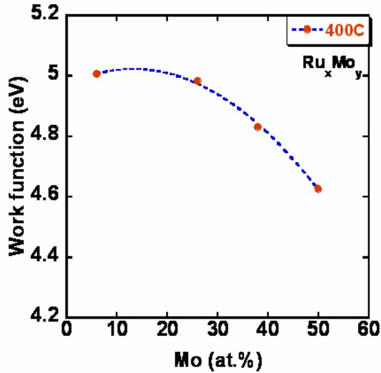
Figure A.5 2<sup>nd</sup> exp. Work functions of as Ru-Mo on varying SiO<sub>2</sub> and HfO<sub>2</sub> after 400°C FGA
