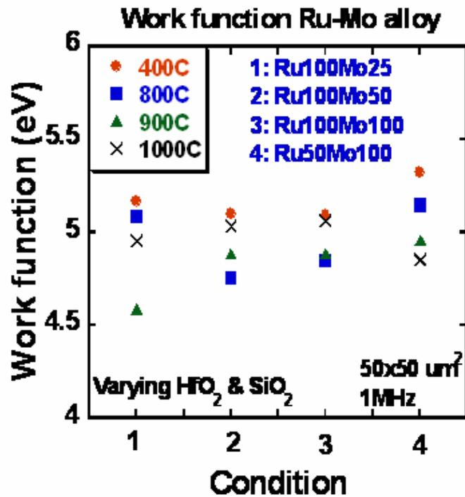
Figure A.4 1<sup>st</sup> exp. Work functions of as Ru-Mo on varying  $SiO_2$  and  $HfO_2$  after different temperature anneal
