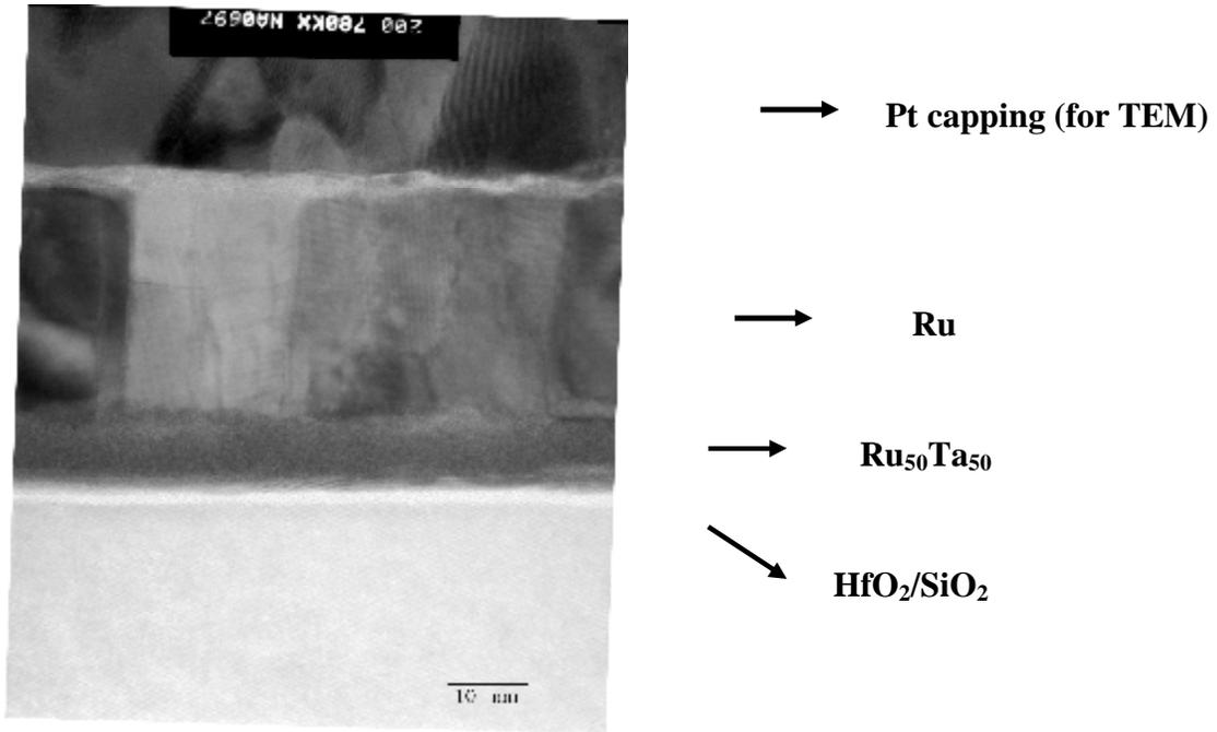
Figure 5. 8 TEM image of Ru 500A gates with underlayer of Ru<sub>50</sub>Ta<sub>50</sub> 100A on HfO<sub>2</sub>/SiO<sub>2</sub> after annealing at 400°C
