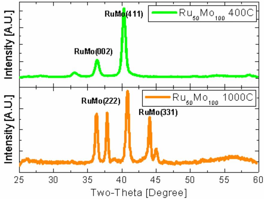
Figure 2.25 XRD analysis (a) 400°C (b) 1000°C of RuMo/SiO<sub>2</sub>
