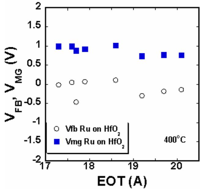
Figure 2. 12  $V_{FB}$  vs. EOT and  $V_{MG}$  EOT curves of Ru based metal electrodes on  $HfO_2$  gate Dielectrics.  $V_{FB}$  data is more scattered due to high  $D_{it}$
