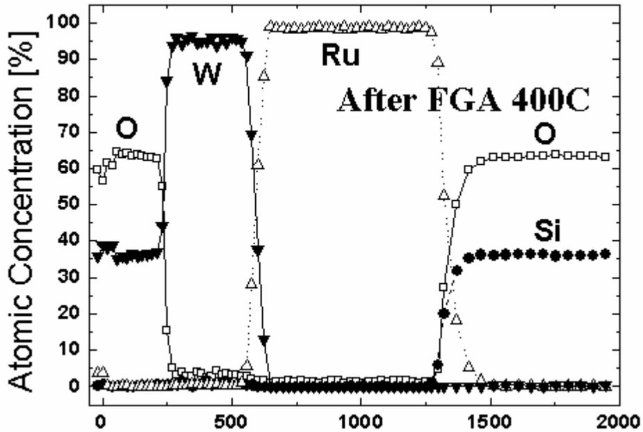
Figure 3. 11 AES Depth profile of Ru 700A with W 600A films on SiO<sub>2</sub> forming gas annealed at 400°C
