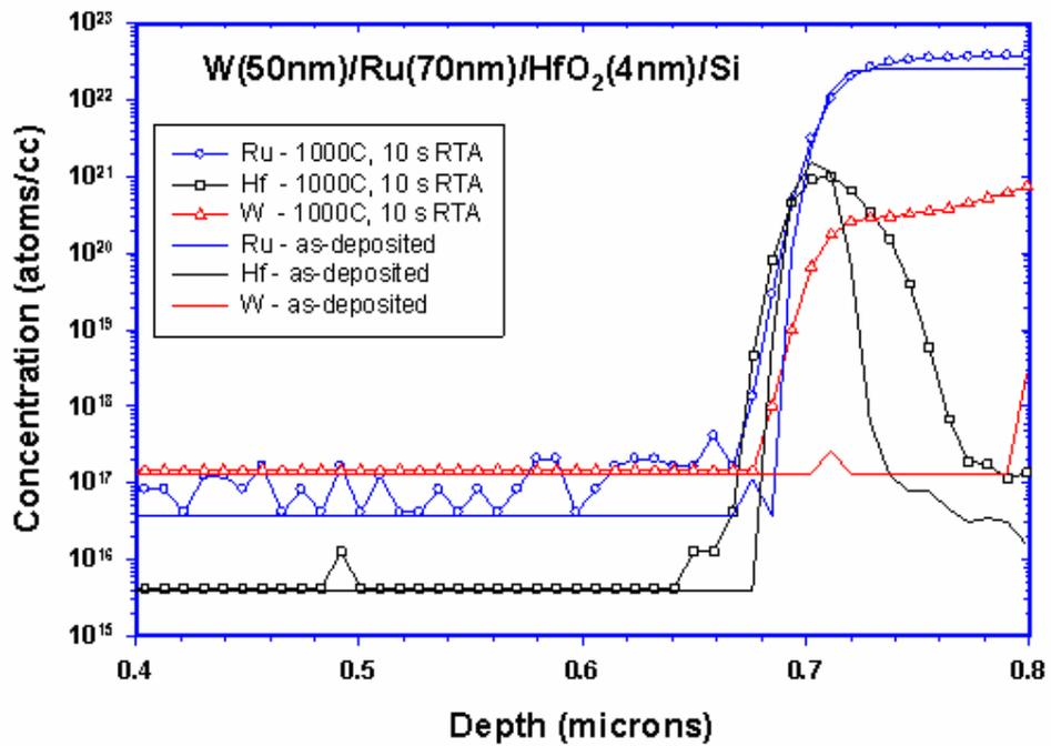
Figure 2. 27 Back side SIMS profile analysis (a) as-deposited (b) 1000°C anneal of W/Ru/HfO<sub>2</sub>
