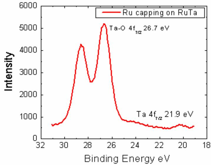
Figure 5. 10 XPS results of Ru 500A/RuTa 100A stacked metal gates after annealing at 800°C
