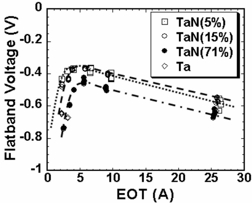
Figure 2. 17  $V_{FB}$  vs. EOT for TaN on varying thicknesses of  $SiO_2$ . The rollover of  $V_{FB}$  is attributed to N diffusion into the  $SiO_2$ .
