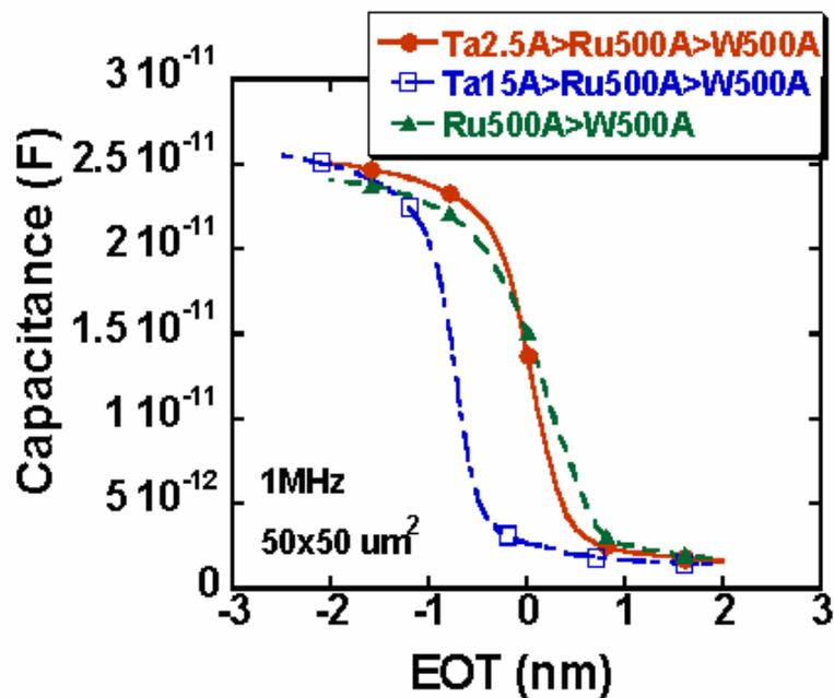
Figure 4. 27 C-V curves for Ta with Ru overlayer with W capping layer gate stacks forming gas annealed at 400°C
