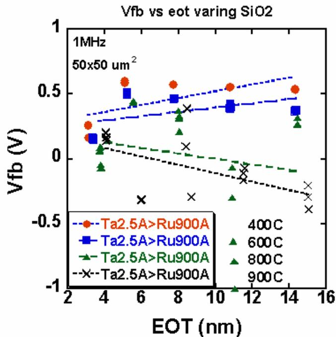
Figure 4. 30 Vfb vs. EOT curves for Ta monolayer with Ru overlayer gate stacks forming gas annealed at various temperatures.
