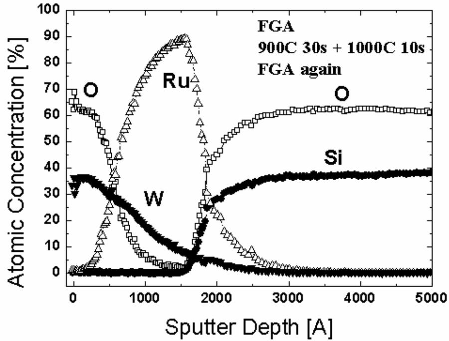
Figure 3. 12 AES Depth profile of Ru 700A with W 600A films on SiO<sub>2</sub> with pre-FGA at 400°C and subsequent 900°C and 1000°C anneal in Ar followed by FGA at 400°C
