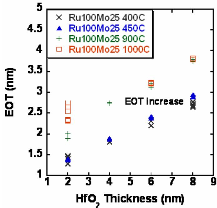
Figure A. 8 EOT change of as Ru 100W Mo 25W on varying HfO<sub>2</sub>/SiO<sub>2</sub> after different anneal
