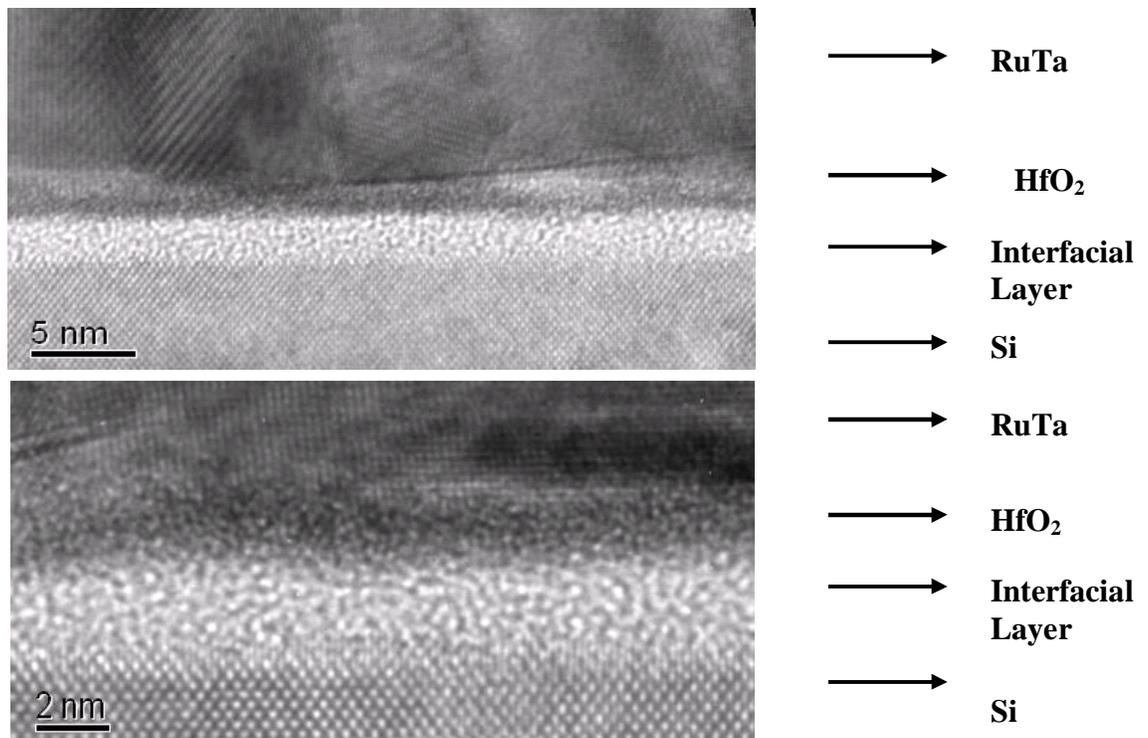
Figure 2. 28 TEM picture at 400°C of RuTa on HfO<sub>2</sub>
