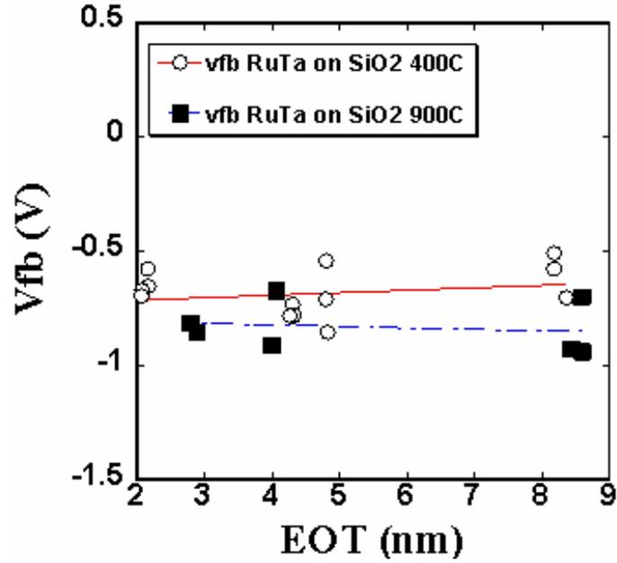
Figure 2. 21  $V_{FB}$  vs. EOT for  $Ru_{50}Ta_{50}$  on  $SiO_2$  as a function of anneal temperature showing the improvement and charge. The difference in intercepts at 400°C and 900°C for both gates is  $\sim 0.05V$
