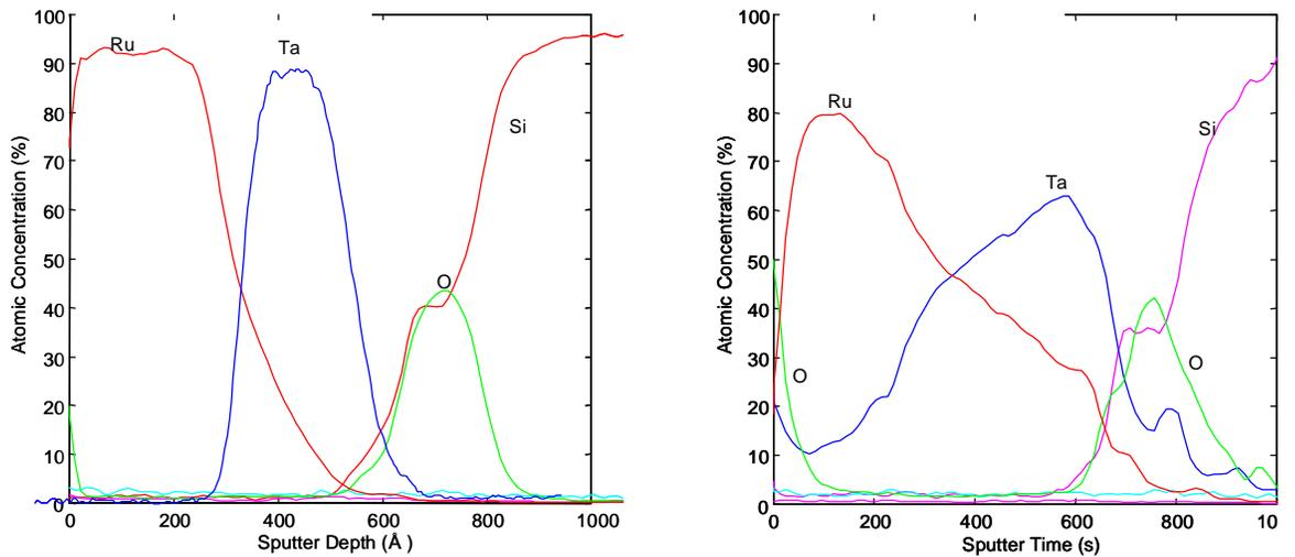
Figure 4. 13 Auger Depth Profile after annealing of Si/SiO<sub>2</sub>/Ru 100Å/Ta 200Å/W 500Å
