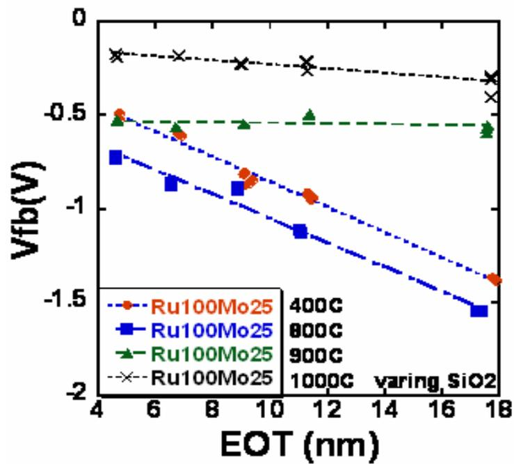
Figure A.6 V<sub>FB</sub> vs. EOT of as Ru-Mo on varying SiO<sub>2</sub> with fixed HfO<sub>2</sub> after different temperature anneal
