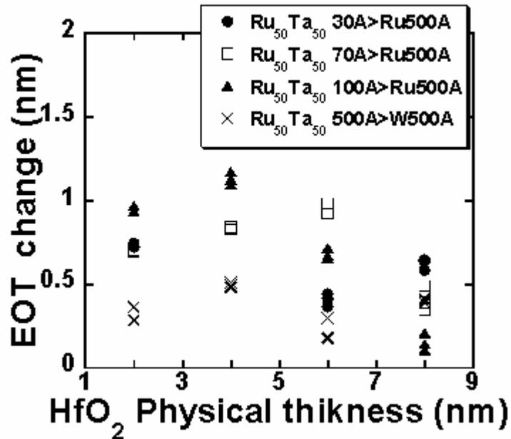
Figure 5. 7 EOT change vs.  $HfO_2$  physical thickness curve of stacked metal gates on  $HfO_2/SiO_2$  after annealing at  $400^\circ C$
