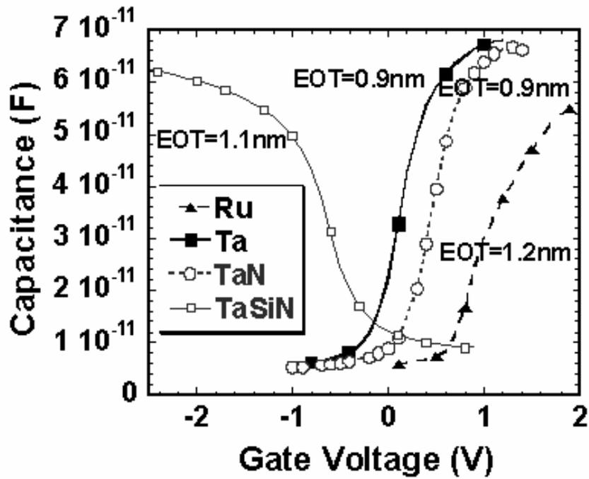
Figure 2. 9 1MHz C-V curves of Ru, Ta, TaN and TaSiN on  $HfO_2$  indicating low EOT values on both n and p substrates.
