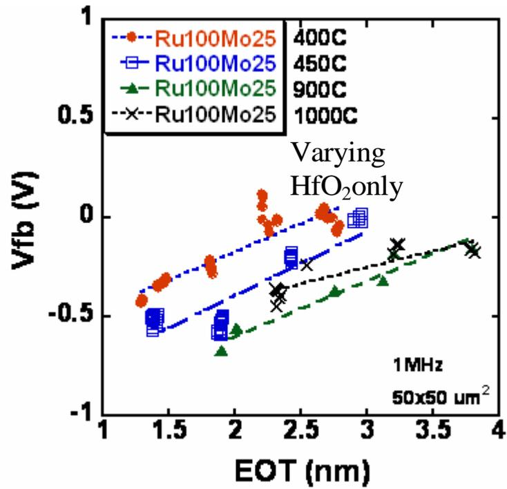
Figure A. 7  $V_{FB}$  vs. EOT of as Ru-Mo on varying HfO<sub>2</sub> after different anneal
