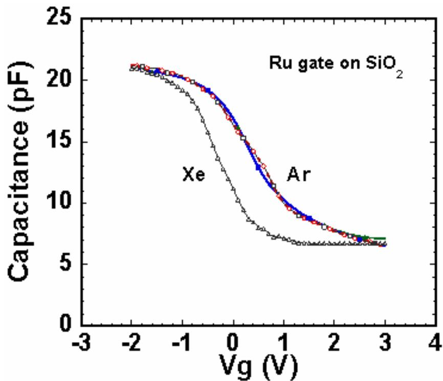
Figure 2. 11 C-V curves Ru gates sputtered in Ar v. Xe on SiO<sub>2</sub>
