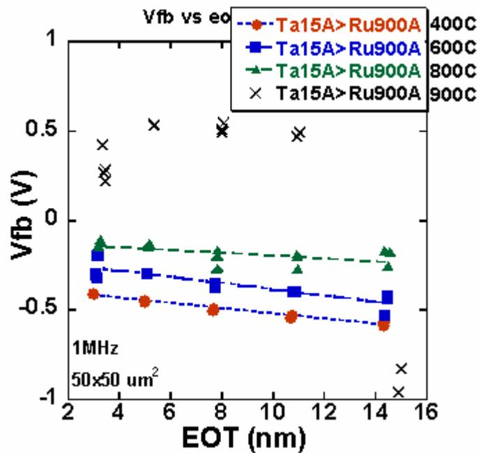
Figure 4.31 Vfb vs. EOT curves for Ta monolayers with Ru overlayer gate stacks forming gas annealed at various temperatures.
