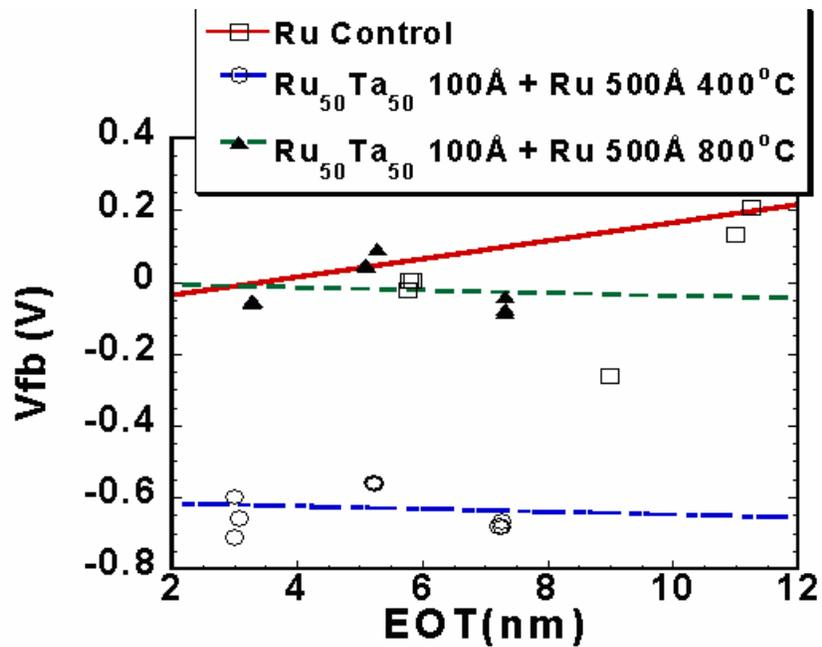
Figure 4. 20 Vfb vs. EOT for Ru<sub>50</sub>Ta<sub>50</sub>/Ru stacks annealed at 800°C for 10min.
