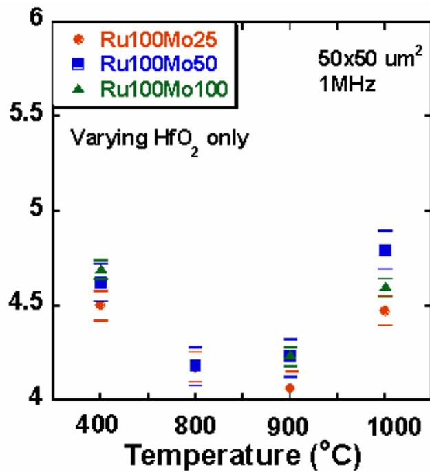
Figure A. 11 Work functions of as Ru-Mo on varying HfO<sub>2</sub> after different temperature anneal
