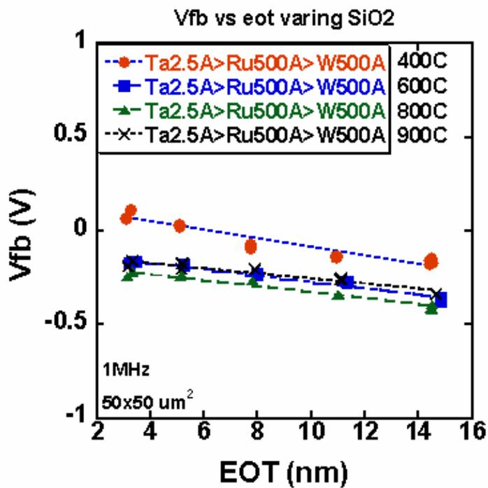
Figure 4. 28 Vfb vs. EOT curves for Ta monolayer with Ru overlayer with W capping layer gate stacks forming gas annealed at various temperatures.
