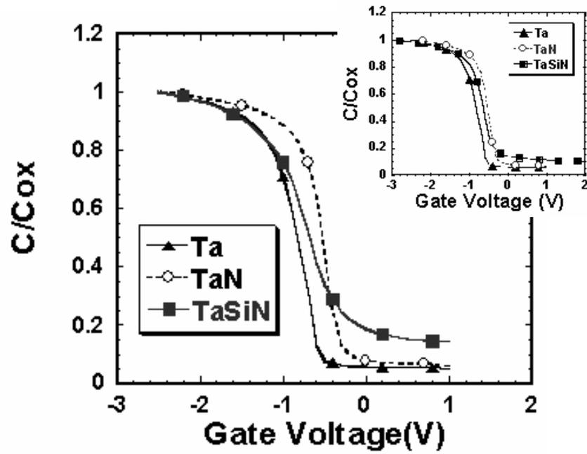
Figure 2. 8 1 MHz C-V curves of Ta based metal electrodes on  $HfO_2$  gate Dielectrics. EOT down to  $11\text{\AA}$  have been obtained. Inset shows the same electrodes on  $SiO_2$ . Similar shifts between the gates are observed on  $HfO_2$  and  $SiO_2$ .
