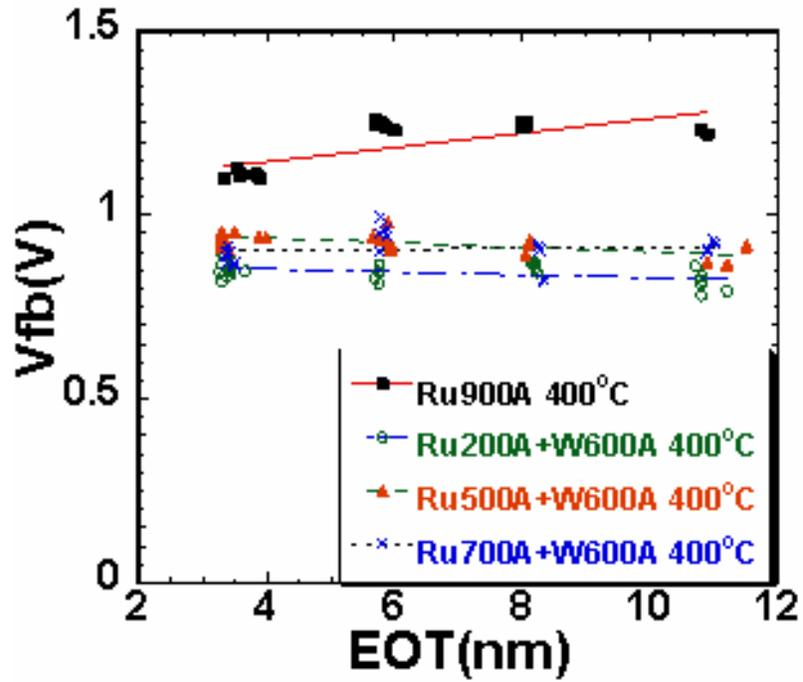
Figure 3.3  $V_{fb}$  vs. EOT for various metal stack conditions FGA at 400°C
