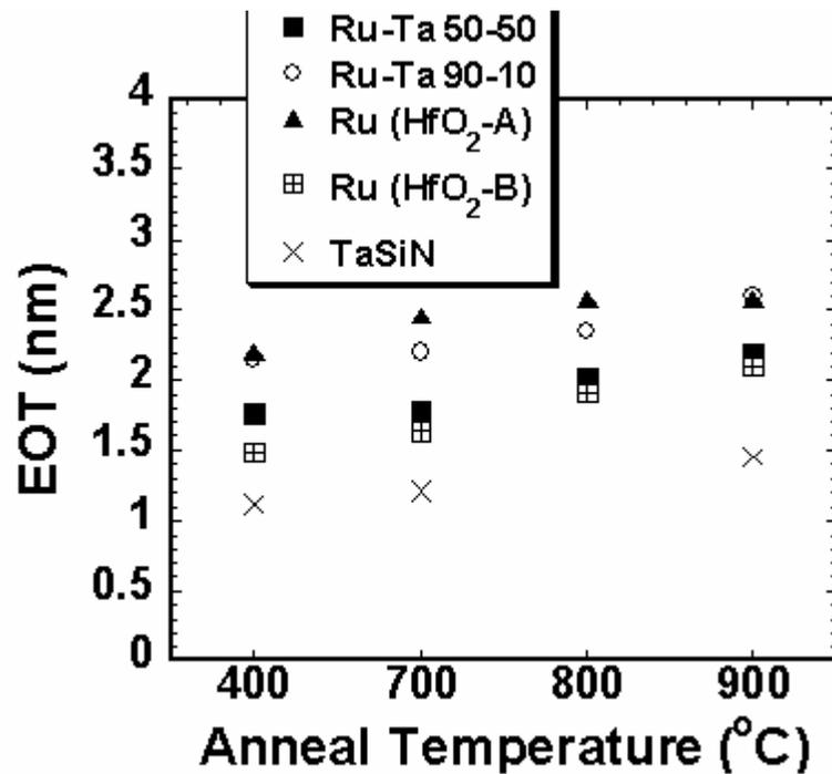
Figure 2. 18 EOT vs. anneal temperature for all gates as a function of anneal temperature. Ru was investigated on two thicknesses of  $HfO_2$ .
