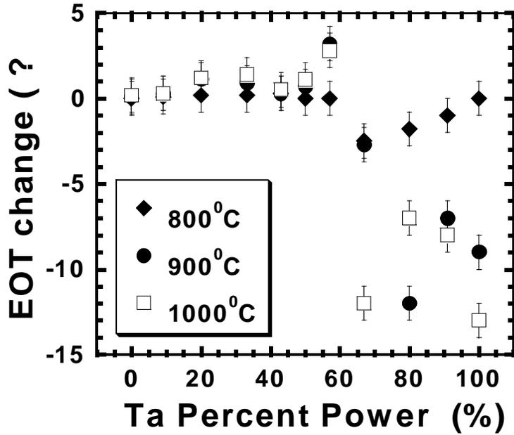
Figure 2. 2 EOT change under high temperature annealing for Ru-Ta alloys with various Ta percent power conditions on 25Å SiO<sub>2</sub> gate dielectrics [3]
