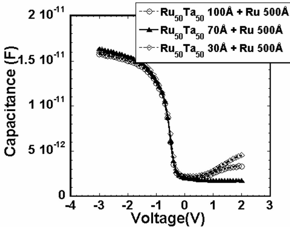
Figure 4. 18 C- V curves of Ru<sub>50</sub>Ta<sub>50</sub>/Ru stacks annealed at 400°C for 30min.
