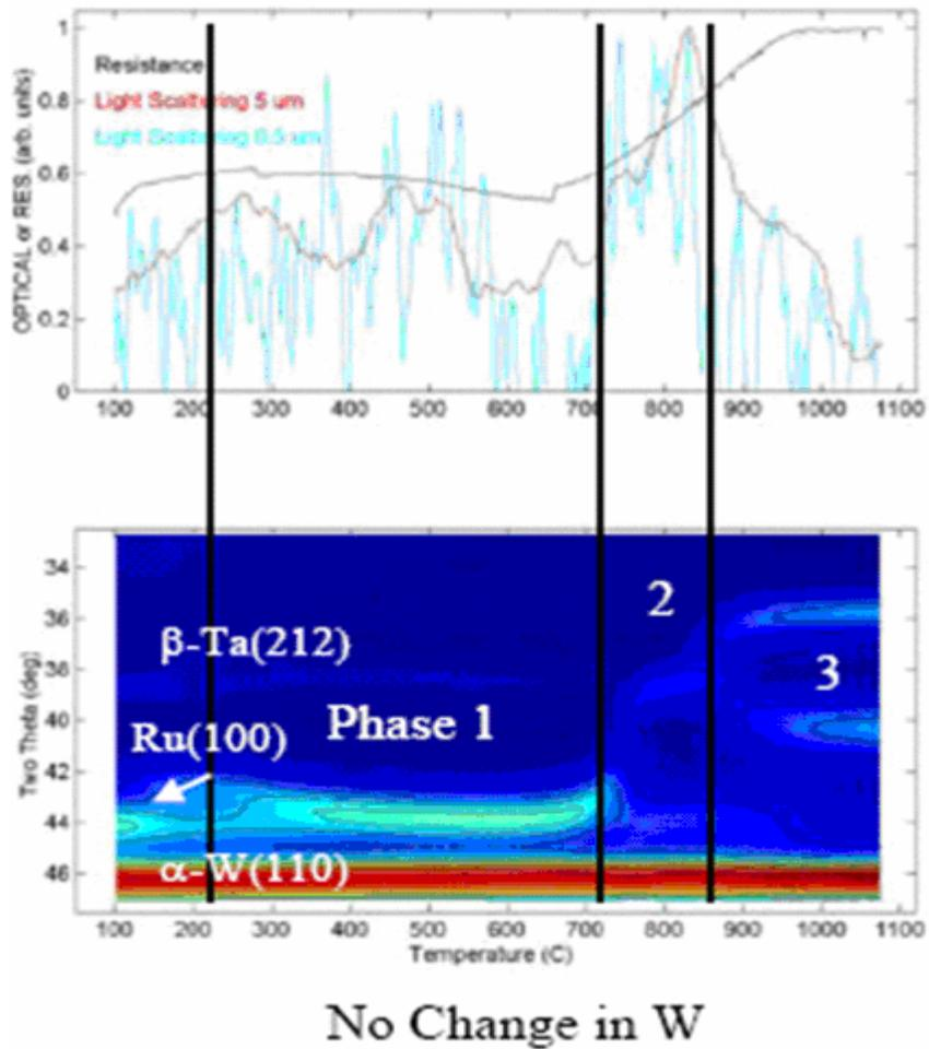
Figure 4. 17 In-situ XRD data of 500Å W / 200Å Ta / 100Å Ru on SiO<sub>2</sub> annealed from 100°C to 1100°C
