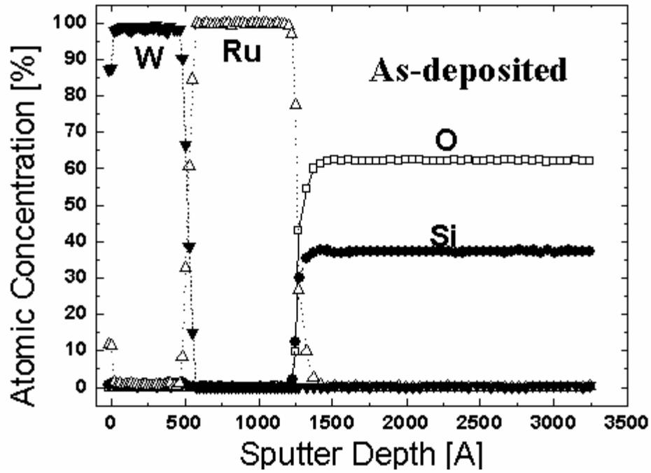
Figure 3. 10 AES Depth profile of as-deposited Ru 700A with W 600A films on SiO<sub>2</sub>
