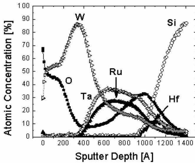
Figure 5. 15 AES depth analysis of Ru<sub>50</sub>Ta<sub>50</sub> 500A with capping layer 500A W on HfO<sub>2</sub>/SiO<sub>2</sub> after annealing at 800°C for 10min.
