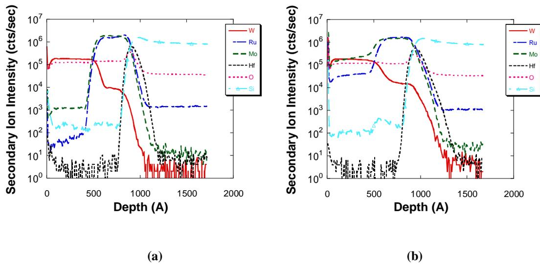
Figure 2.26 SIMS profile analysis (a) as-deposited (b) 900°C anneal of W/RuMo/SiO<sub>2</sub>
