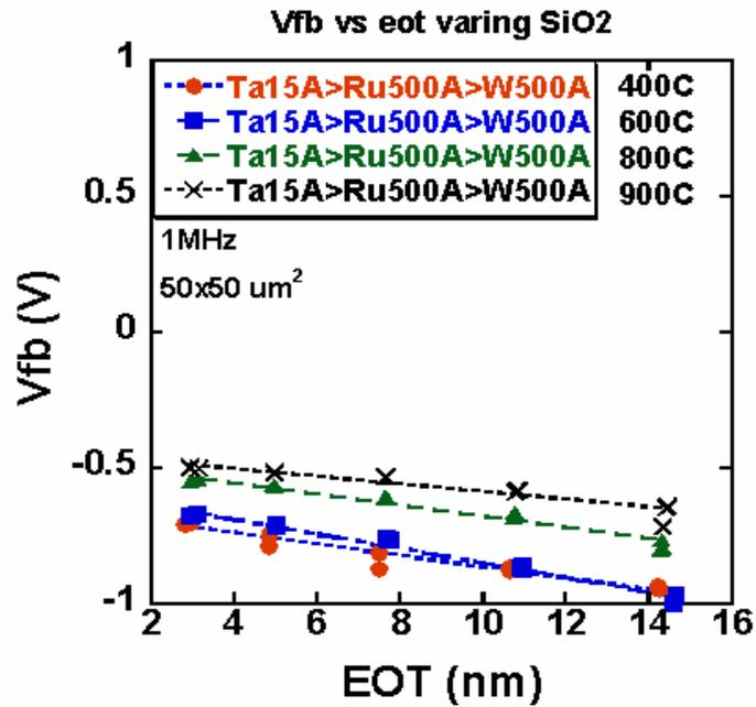
Figure 4. 29 Vfb vs. EOT curves for Ta monolayers with Ru overlayer with W capping layer gate stacks forming gas annealed at various temperatures.
