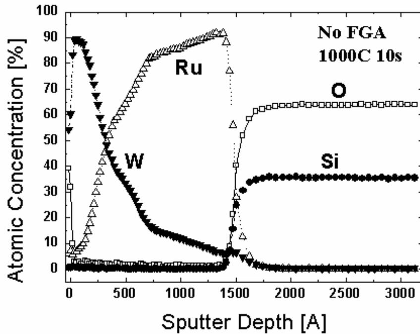
Figure 3. 13 AES Depth profile of Ru 700A with W 600A films on SiO<sub>2</sub> without pre-FGA and subsequent 900°C and 1000°C anneal in Ar.
