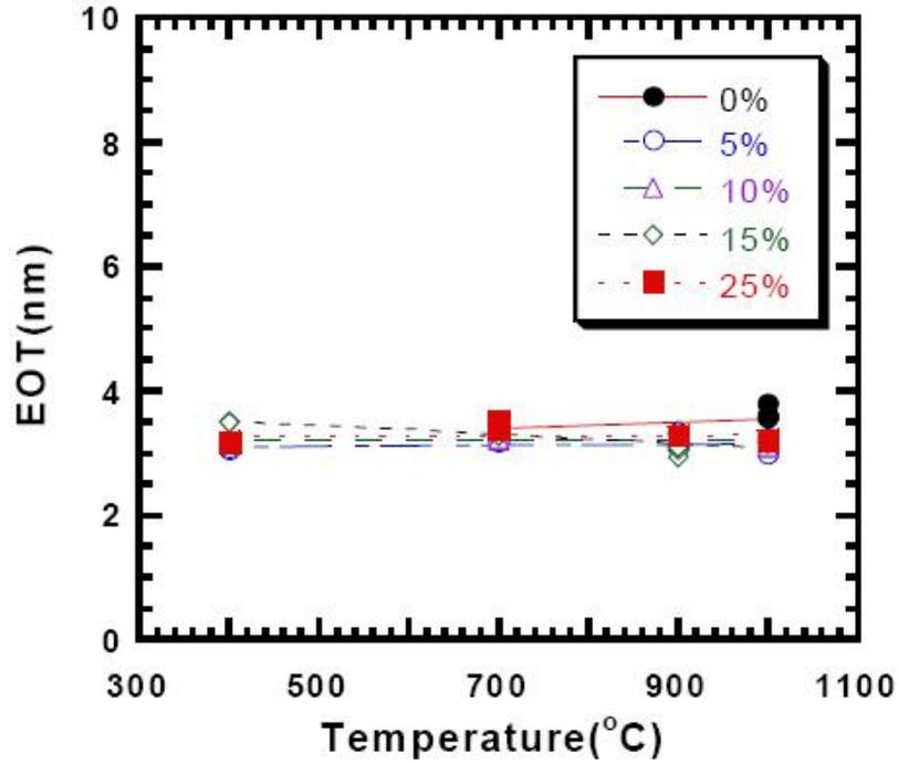
Figure 2. 5 EOT vs. annealing conditions at the various TaSixNy electrodes [8].
