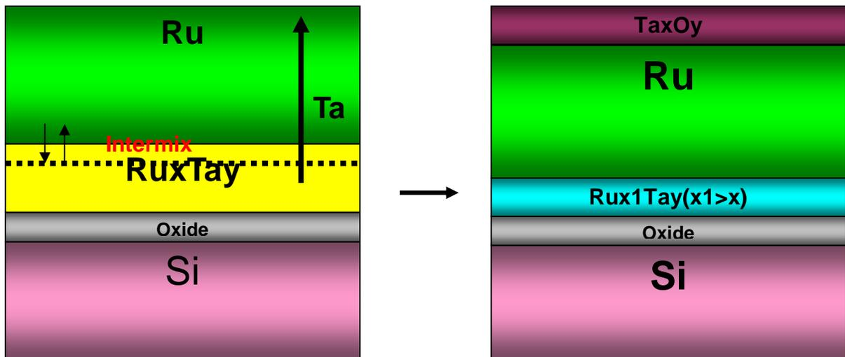
Figure 5.18 Schematic of Ru 500A with the underlayer of Ru<sub>50</sub>Ta<sub>50</sub> 100A on HfO<sub>2</sub>/SiO<sub>2</sub> after annealing at 800°C for 10min
