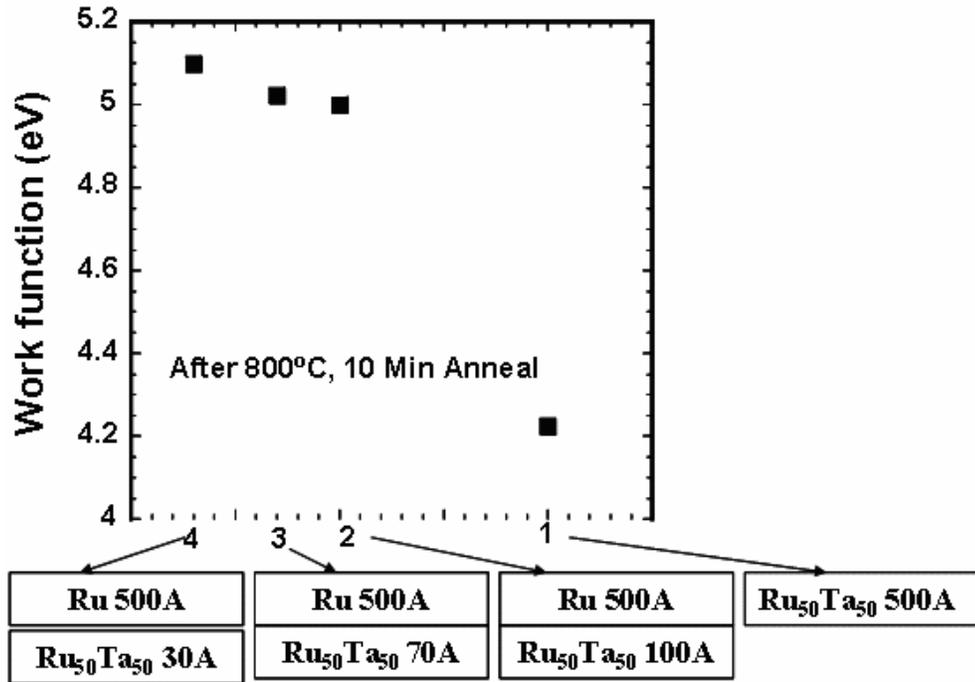
Figure 4. 21 Work function vs. sample condition: Ru<sub>50</sub>Ta<sub>50</sub>/Ru stacks annealed at 800°C for 10min.
