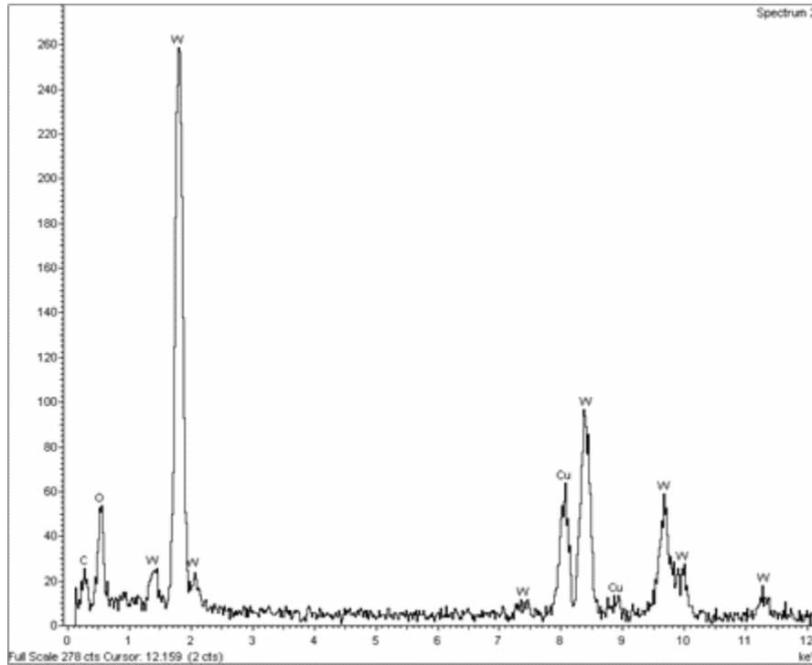
Figure 5. 17 EDX analysis of surface of Ru<sub>50</sub>Ta<sub>50</sub> 500A with capping layer W 500A on HfO<sub>2</sub>/SiO<sub>2</sub> after annealing at 800°C for 10min.
