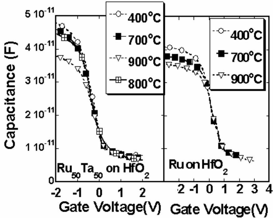
Figure 2. 19 1MHz C - V curves for metals on  $\text{HfO}_2$  as a function of anneal temperature.
