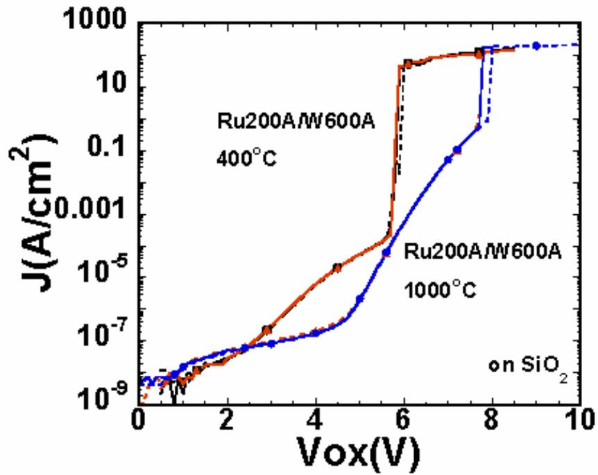
Figure 3.8 I-V curves of Ru 200A with W 600A films on SiO<sub>2</sub> annealed at 400°C and at 1000°C
