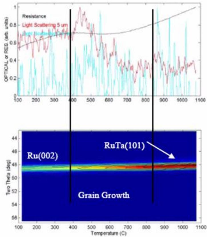
Figure 4. 25 The in-situ XRD data of 500A Ru / 30A RuTa / SiO2 annealed from 100°C to 1100°C
