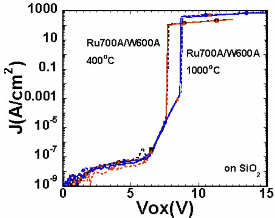
Figure 3.9 I-V curves for Ru 700A with W 600A films on SiO<sub>2</sub> with FGA at 400°C and 1000°C anneal in Ar.
