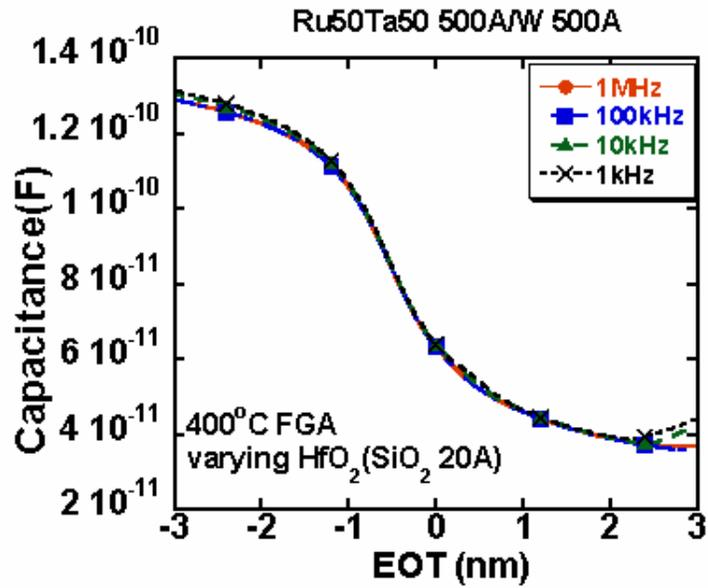
Figure 5. 4 C-V curve frequency dispersion of RuTa500A/W500A with overlayer Ru 500A stacked metal gate on HfO<sub>2</sub>/SiO<sub>2</sub> after annealing at 400°C
