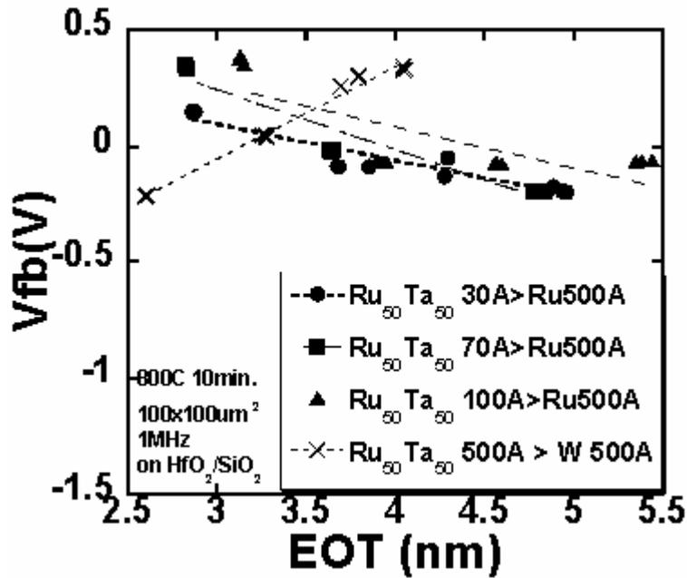
Figure 5. 6  $V_{fb}$  vs. EOT curves of stacked metal gates on  $HfO_2/SiO_2$  after annealing at  $800^\circ C$
