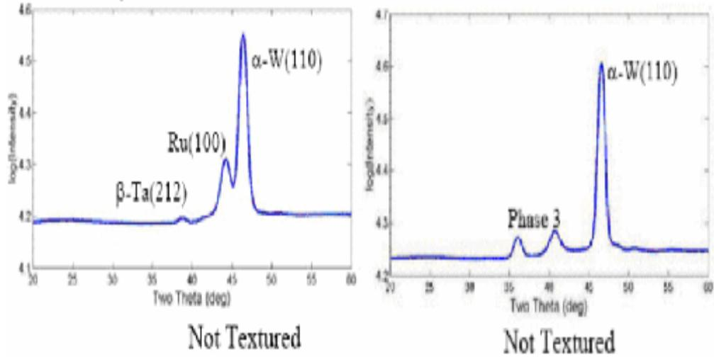
Figure 4. 16 The in-situ XRD data of 500Å W / 200Å Ta / Ru 100Å /SiO<sub>2</sub> (a) As-deposited (b) after 1100°C anneal
