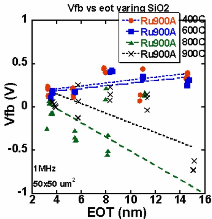
Figure 4.32 Vfb vs. EOT curves for Ru single gate stacks forming gas annealed at various temperatures.
