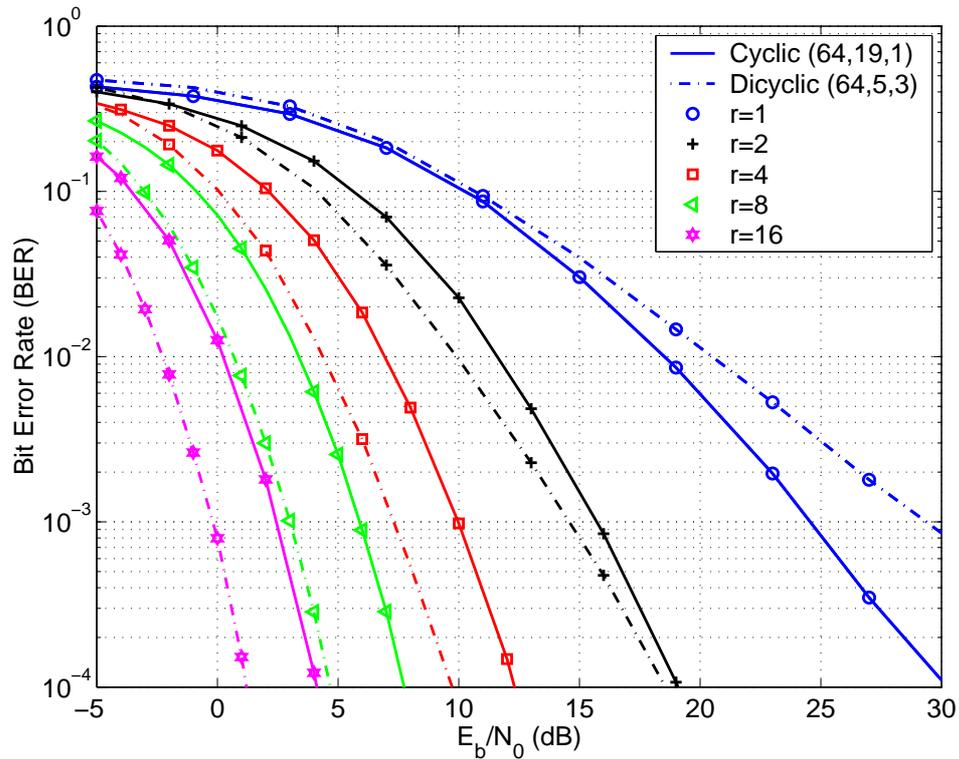
Figure 2.2: BER performance of cyclic vs dicyclic group codes for  $R = 3$  bps/Hz and  $r = 1, 2, 4, 8, 16$
