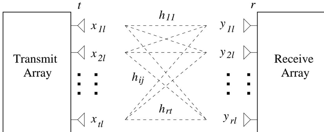
Figure 2.1: MIMO channel model
