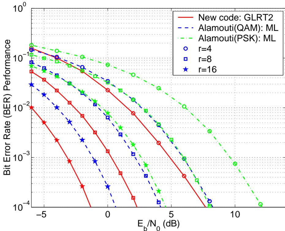
Figure 3.4: BER comparison of the new code using GLRT2 decoding with the Alamouti code with QAM and PSK respectively at  $R = 4$  bps/Hz for  $t = 2$  and  $r = 4, 8, 16$ .
