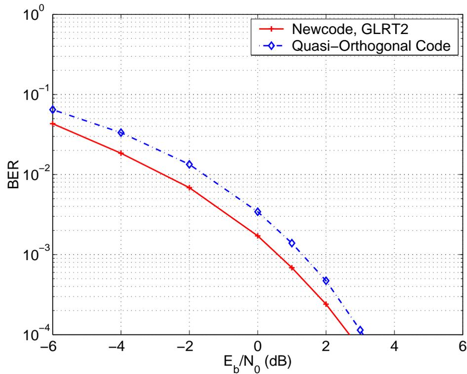
Figure 3.12: BER of new code with GLRT2 receiver and Quasi-orthogonal code for rate  $R = 3$  bps/Hz,  $t = 4$ ,  $r = 8$  receive antennas and coherent detection.
