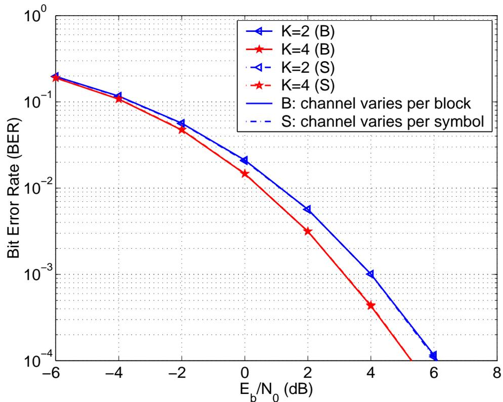
Figure 4.1: Comparison of performance of GLRT2 receiver for conventional DD ( $K=2$ ) and DFDD ( $K=4$ ), with  $R = 4$  bps/Hz,  $t = 2$  transmit antennas,  $r = 8$  receive antennas and  $f_{dt}=0.01$ .
