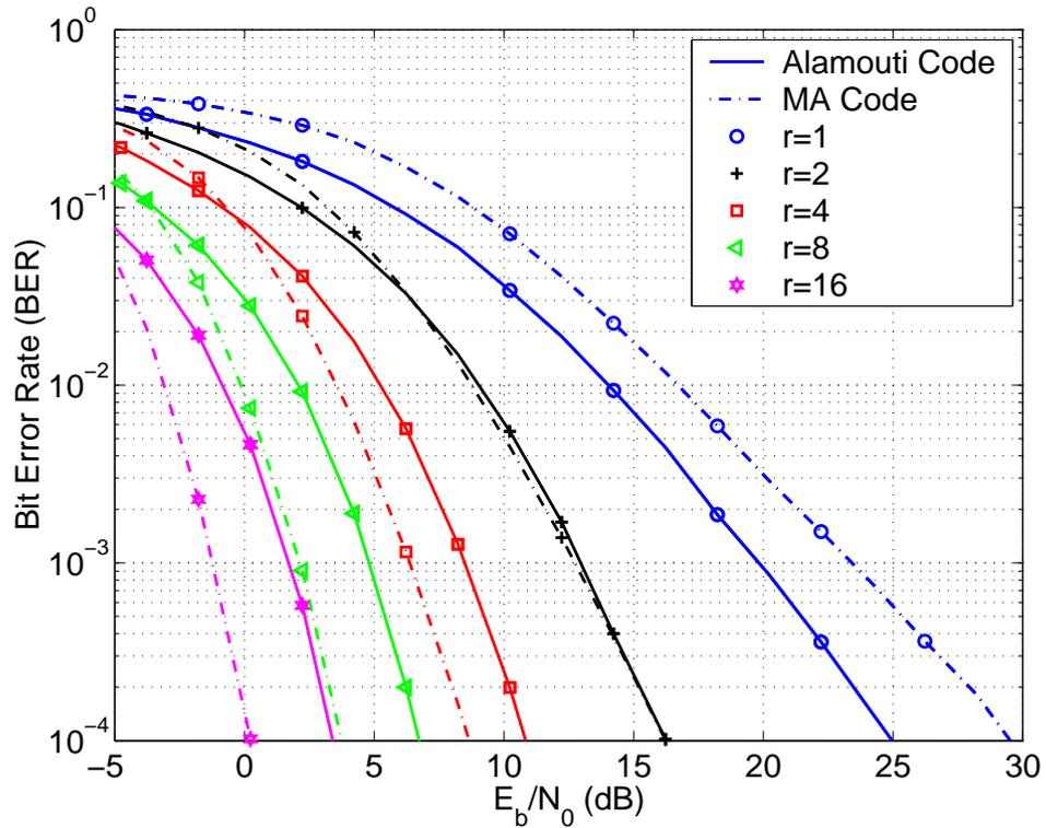
Figure 2.4: BER performance of Alamouti vs Modified Alamouti codes for  $R = 3$  bps/Hz and  $r = 1, 2, 4, 8, 16$
