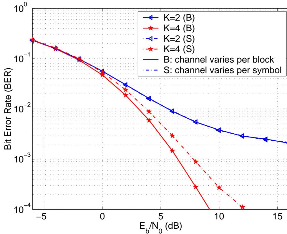
Figure 4.3: Comparison of performance of GLRT2 receiver for conventional DD ( $K=2$ ) and DFDD ( $K=4$ ), with  $R = 4$  bps/Hz,  $t = 2$  transmit antennas,  $r = 8$  receive antennas and  $f_{dt}=0.05$ .
