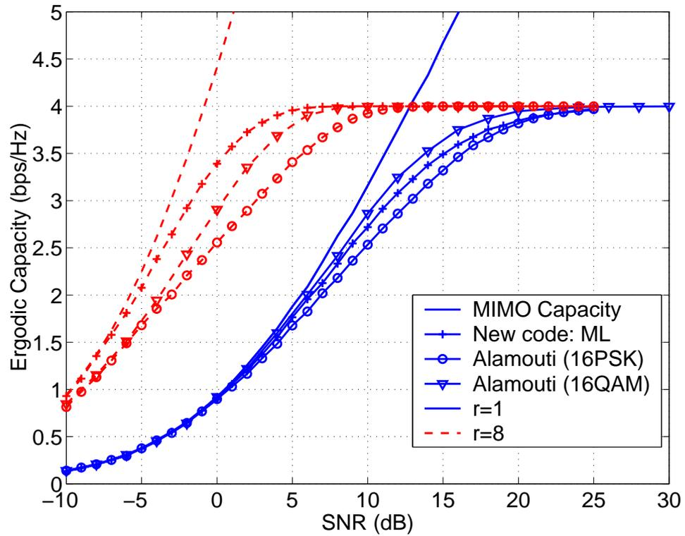
Figure 3.10: Comparison of ergodic capacity of the new code and Alamouti code at  $R = 4$  bps/Hz for  $t = 2$ ,  $r = 1$  and  $r = 8$  respectively.
