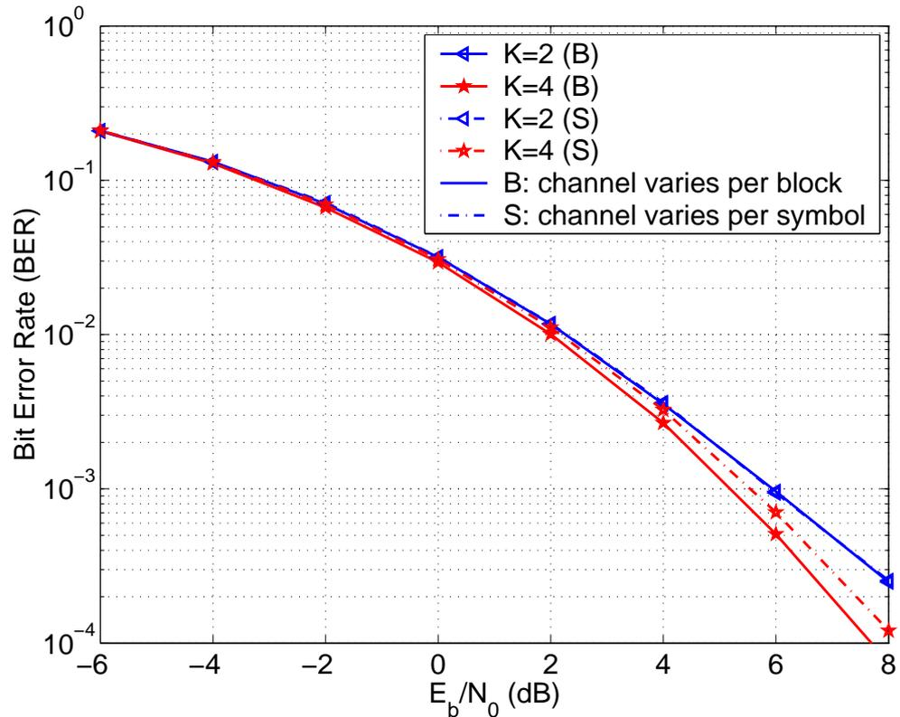
Figure 4.2: Comparison of performance of GLRT2 receiver for conventional DD ( $K=2$ ) and DFDD ( $K=4$ ), with  $R = 4$  bps/Hz,  $t = 2$  transmit antennas,  $r = 8$  receive antennas and  $\text{fdt}=0.03$ .
