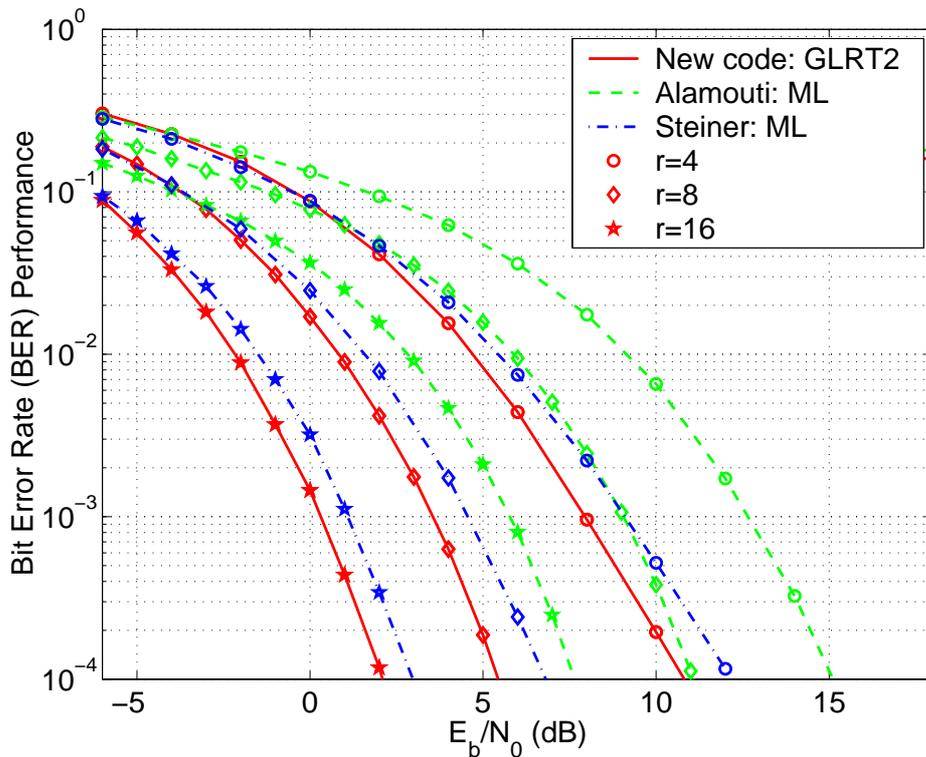
Figure 3.7: BER comparison of the new code using GLRT2 decoding with the Alamouti and Steiner codes at  $R = 4$  bps/Hz for  $t = 2$  and  $r = 4, 8, 16$  in DSTM
