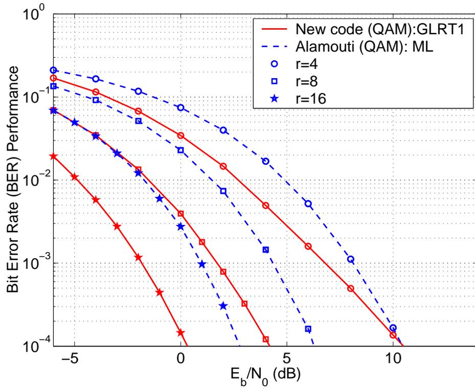
Figure 3.5: BER comparison of new code with GLRT1 decoding and Alamouti code at  $R = 5$  bps/Hz for  $t = 2$ ,  $r = 4, 8, 16$  with coherent detection.
