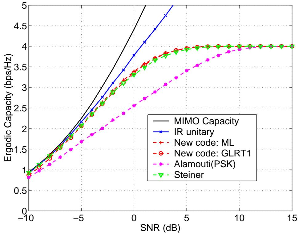
Figure 3.9: Ergodic capacity of the new code with ML and GLRT1 decoding, Alamouti code and Steiner code at  $R = 4$  bps/Hz for  $t = 2$ ,  $r = 8$ .
