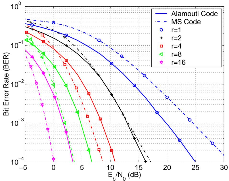
Figure 2.5: BER performance of Alamouti vs Modified Steiner codes for  $R = 3$  bps/Hz and  $r = 1, 2, 4, 8, 16$
