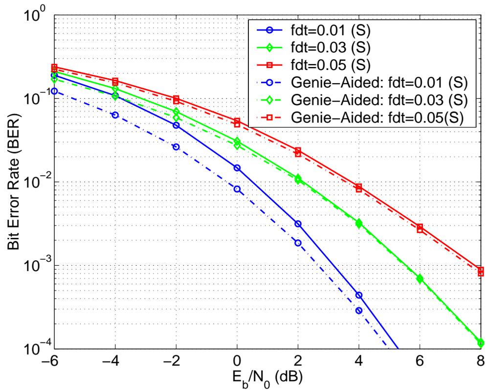
Figure 4.5: Comparison of performance of GLRT2 receiver with DFDD or Genie-Aided DFDD ( $R = 4$  bps/Hz,  $t = 2$  transmit antennas and  $r = 8$  receive antennas and  $fdt = 0.01, 0.03, 0.05$  respectively. Channel varies symbol by symbol.
