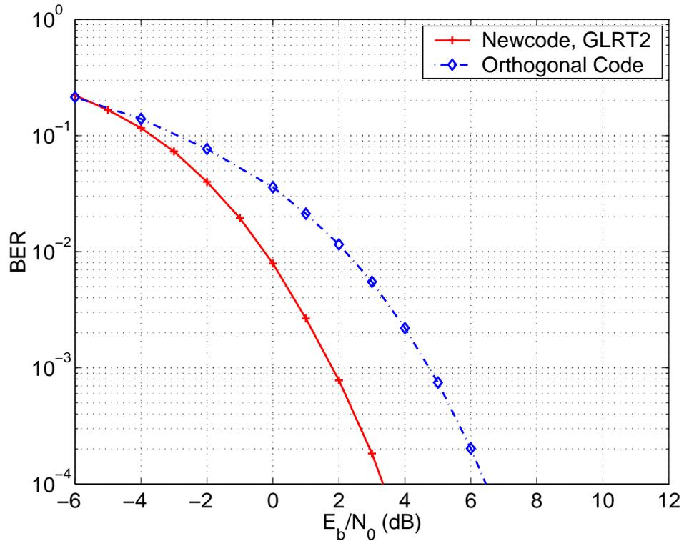
Figure 3.11: BER of new code at  $R = 2$  with GLRT2 receiver and Orthogonal code at  $R = 2.25$  for  $t = 4$ ,  $r = 8$  receive antennas and DSTM structure.
