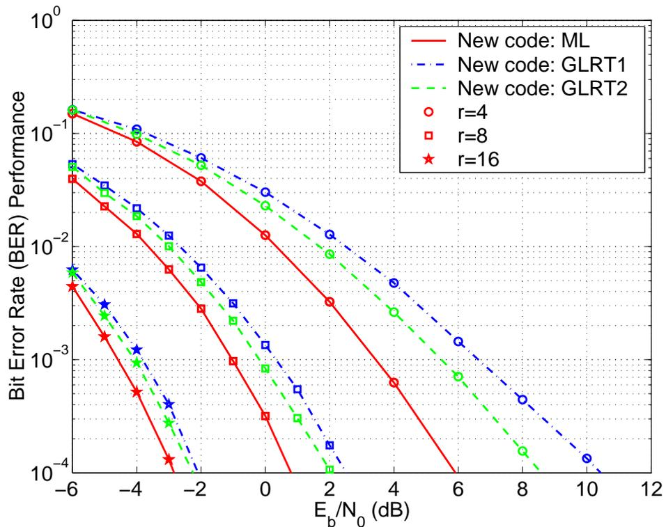
Figure 3.1: BER performance of the new code with ML, GLRT1 and GLRT2 decoding at  $R = 3$  bps/Hz for  $t = 2$  and  $r = 4, 8, 16$  with coherent detection.
