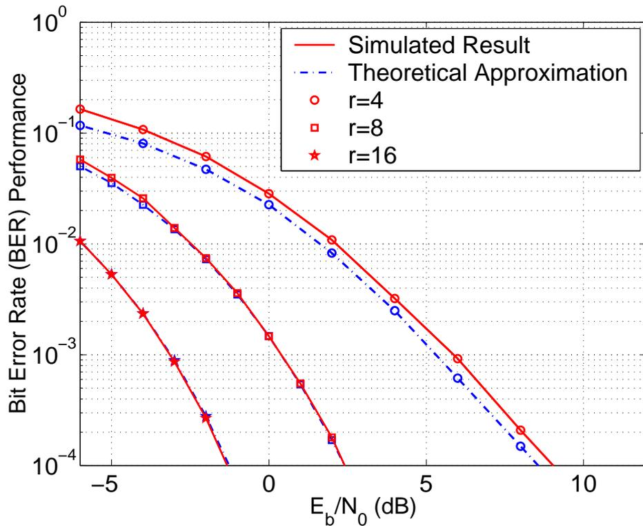
Figure 3.6: Comparison of simulated BER performance and theoretical approximation for GLRT1 decoder at  $R = 4$  bps/Hz for  $t = 2$  and 4, 8, 16
