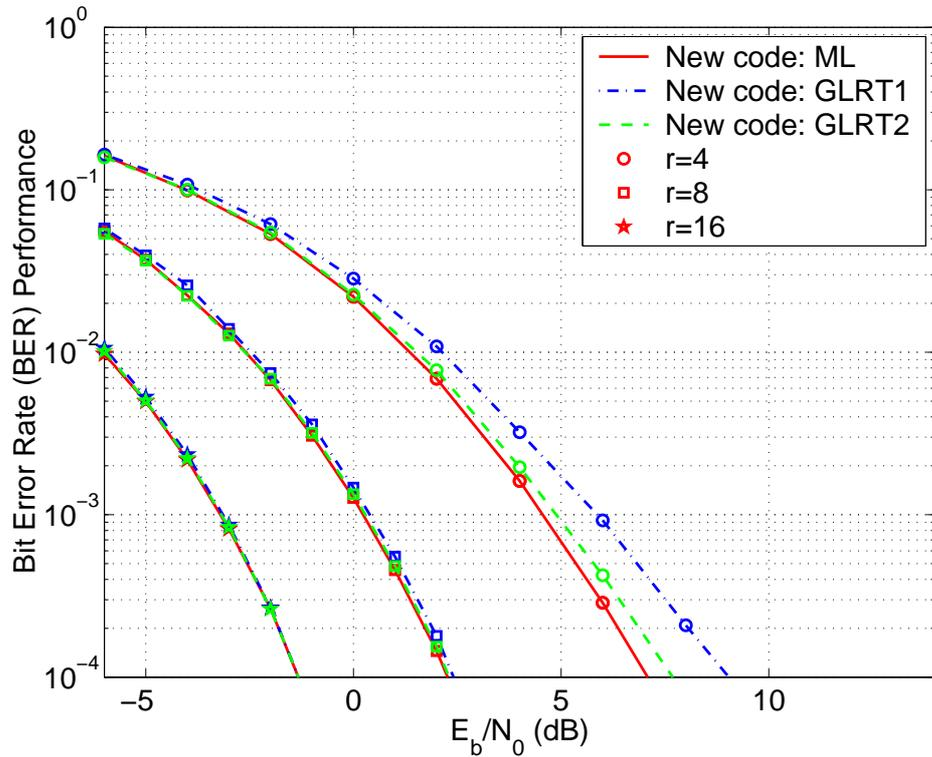
Figure 3.3: BER of new code with ML, GLRT1 and GLRT2 decoding at  $R = 4$  bps/Hz for  $t = 2$  and  $r = 4, 8, 16$  with coherent detection.
