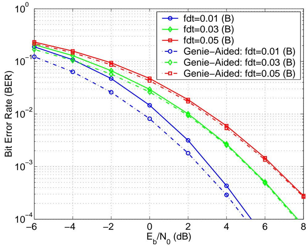
Figure 4.4: Comparison of performance of GLRT2 receiver with DFDD or Genie-Aided DFDD ( $R = 4$  bps/Hz,  $t = 2$  transmit antennas and  $r = 8$  receive antennas and  $fdt = 0.01, 0.03, 0.05$  respectively. Channel varies block by block.
