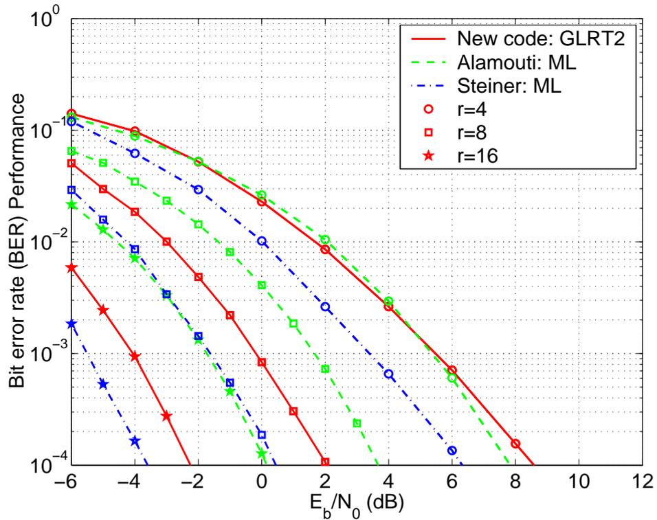
Figure 3.2: BER comparison of the new code using GLRT2 decoding with the Alamouti and Steiner codes using ML decoding at  $R = 3$  bps/Hz for  $t = 2$  and  $r = 4, 8, 16$  with coherent detection.
