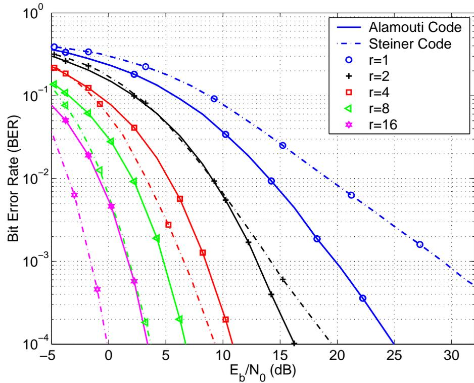
Figure 2.3: BER performance of Alamouti vs Steiner codes for  $R = 3$  bps/Hz and  $r = 1, 2, 4, 8, 16$
