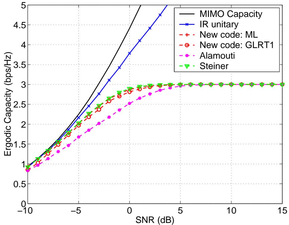
Figure 3.8: Ergodic capacity of the new code with ML and GLRT1 decoding, Alamouti code and Steiner code at  $R = 3$  bps/Hz for  $t = 2$ ,  $r = 8$ .
