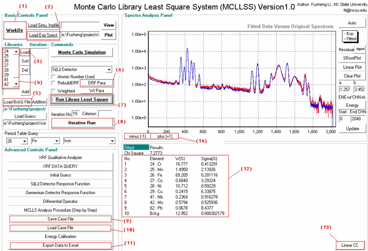
Figure 5.1 Main-page of X-ray Fluorescence Quantitative Analyzer
