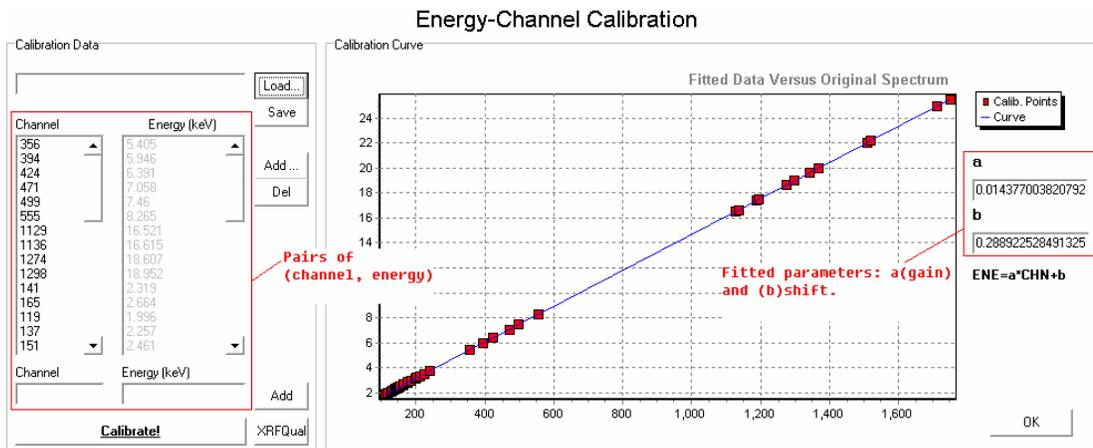
Figure 5.4 Module of energy calibration
