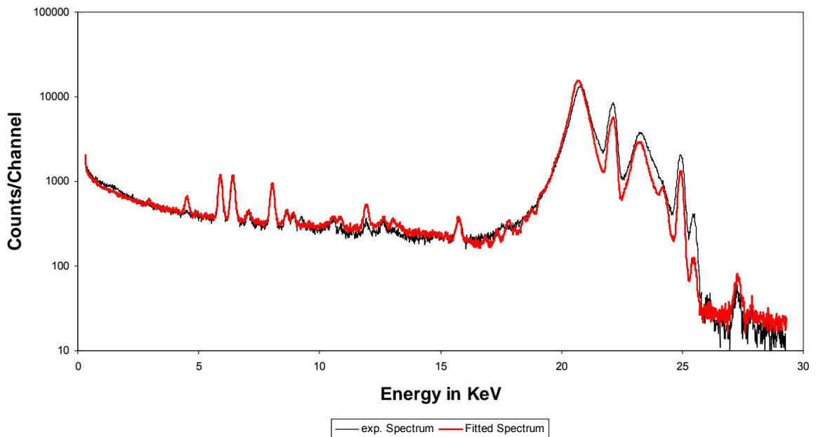
Figure 6.8 Experimental spectrum and fitted spectrum for AA3004
