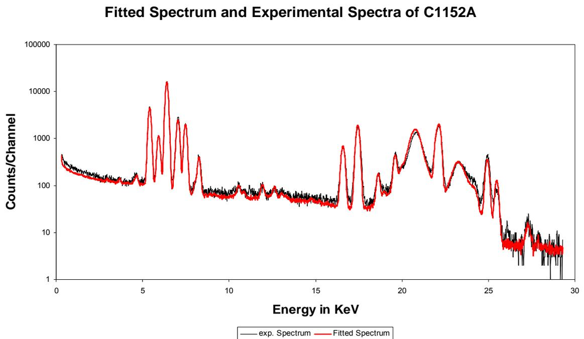
Figure 6.6 Experimental and fitted spectra for C1152A
