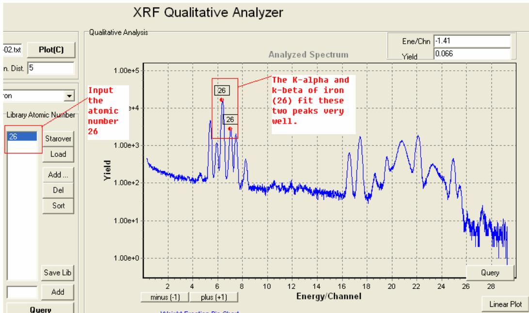
Figure 5.8 Detection of element (iron) in XRF Qualitative Analyzer
