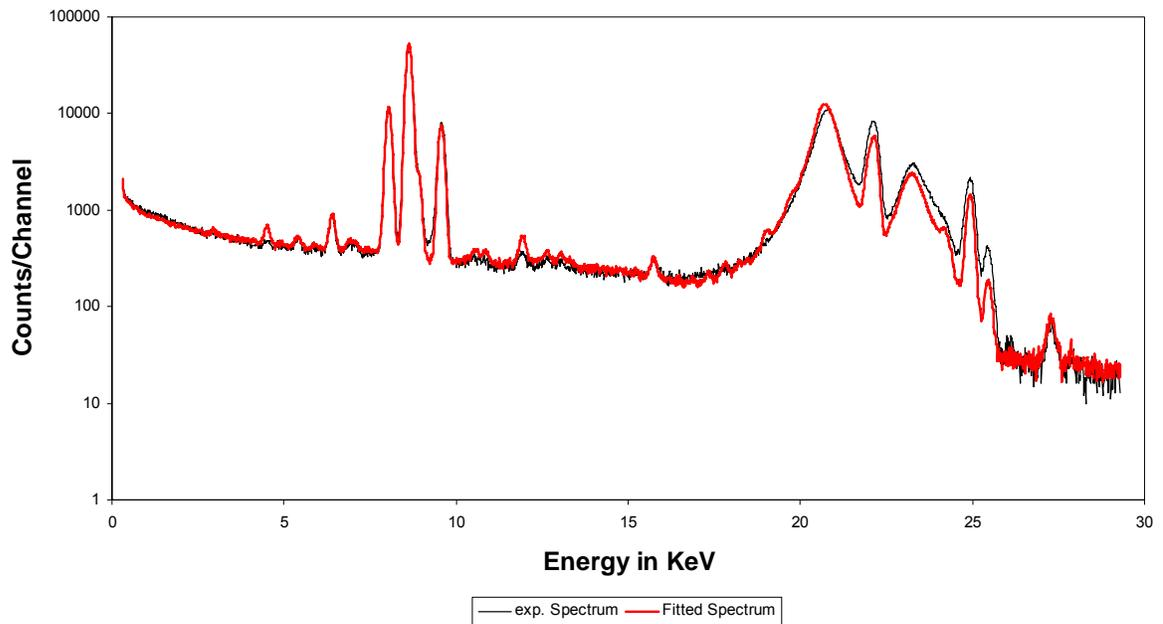
Figure 6.9 Experimental spectrum and fitted spectrum for AA7178
