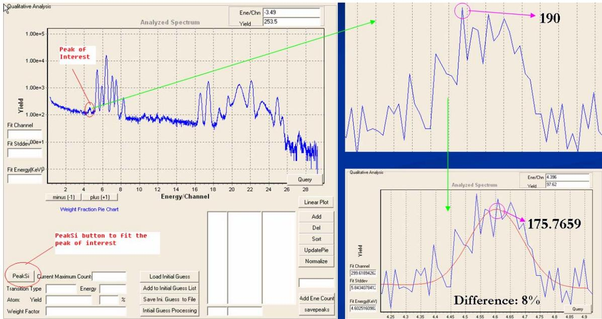
Figure 7.5 PeakSi analysis on peak with poor statistics
