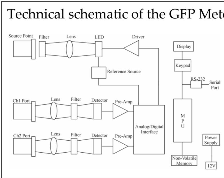
Figure 1. Technical schematic of the GFP Meter.
