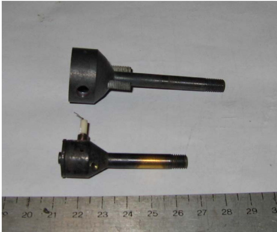
Figure 29: 5 cm and 8 cm Pulsejets
