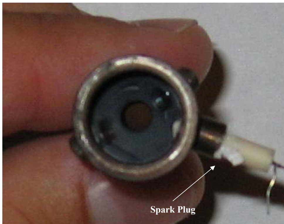
Figure 30: Frontal View of 5 cm Pulsejet
