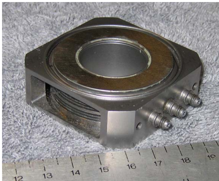
Figure 11: Kistler 3-Component Force Sensor
