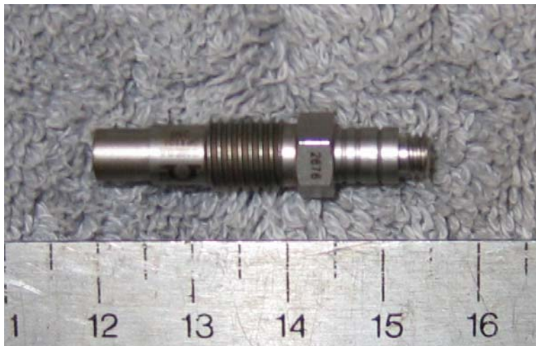
Figure 9: Omega DPX101-250 Pressure Transducer
