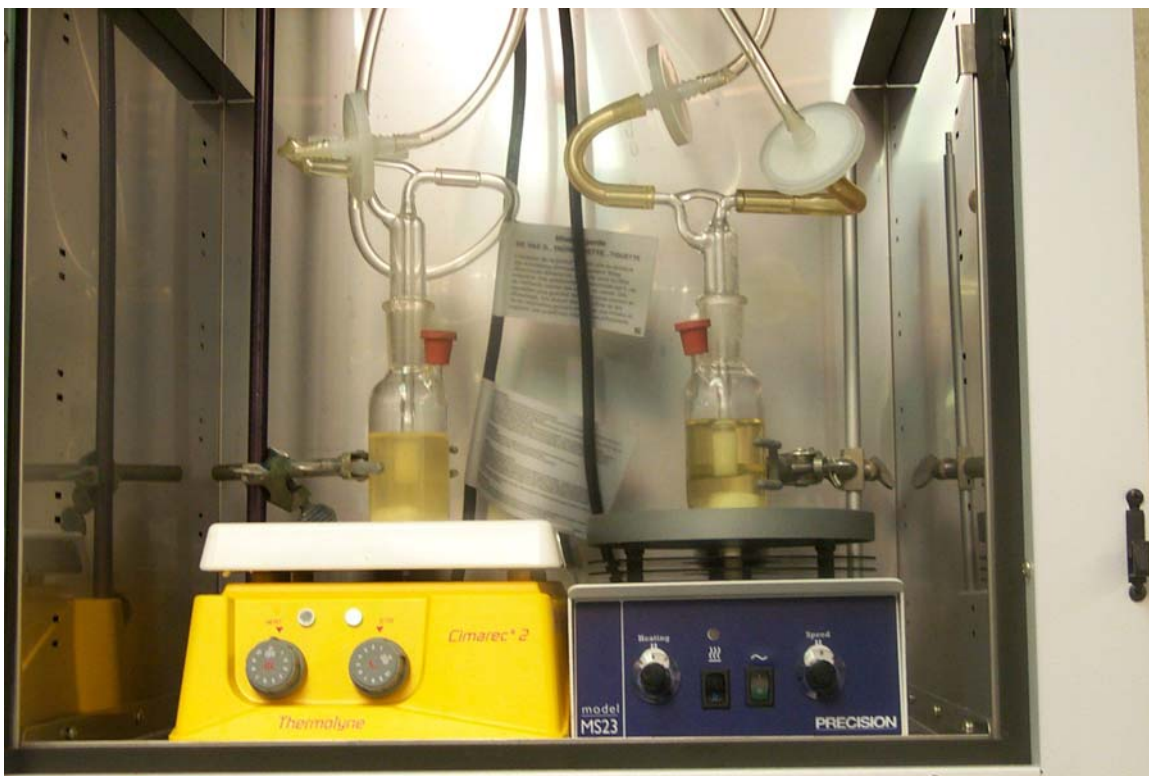
Figure 2. Experimental set-up of growth experiments used to calculate generation times. Inside the glass vessel rests a stir bar. Suspended within the device is the glass dispersion tube.
