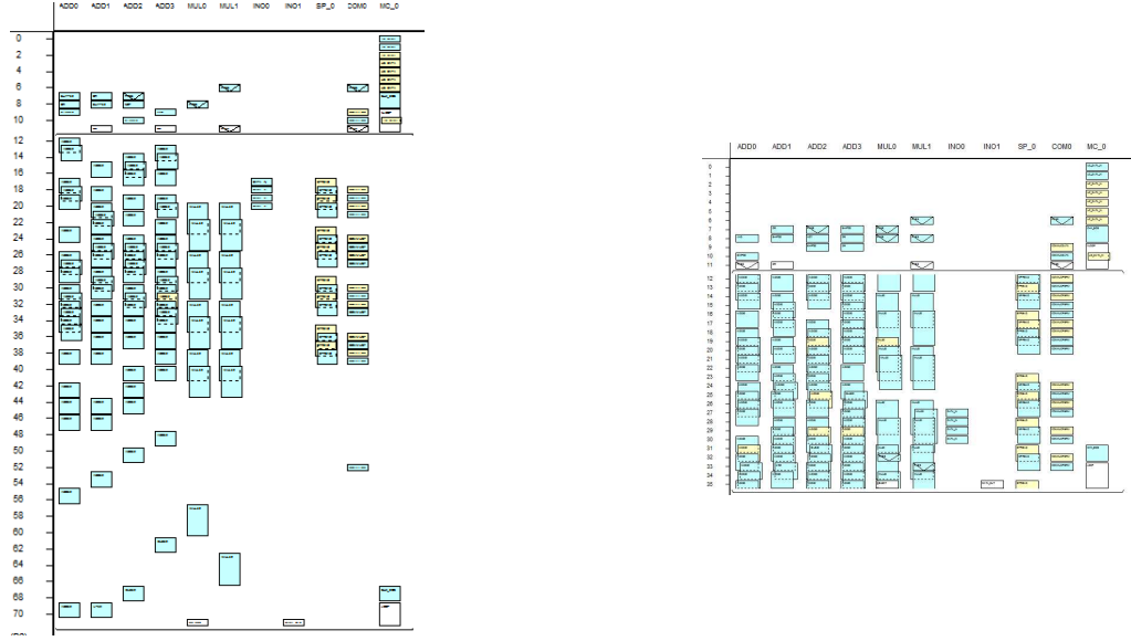
Figure 4.4: The VLIW scheduling results by IScd for the first kernel. The optimized result by using the software pipelining technique is shown in the right. For the second basic block, the total cycle is reduced by 60% and the average kernel utilization for adders is increased from 35% to 85%.
