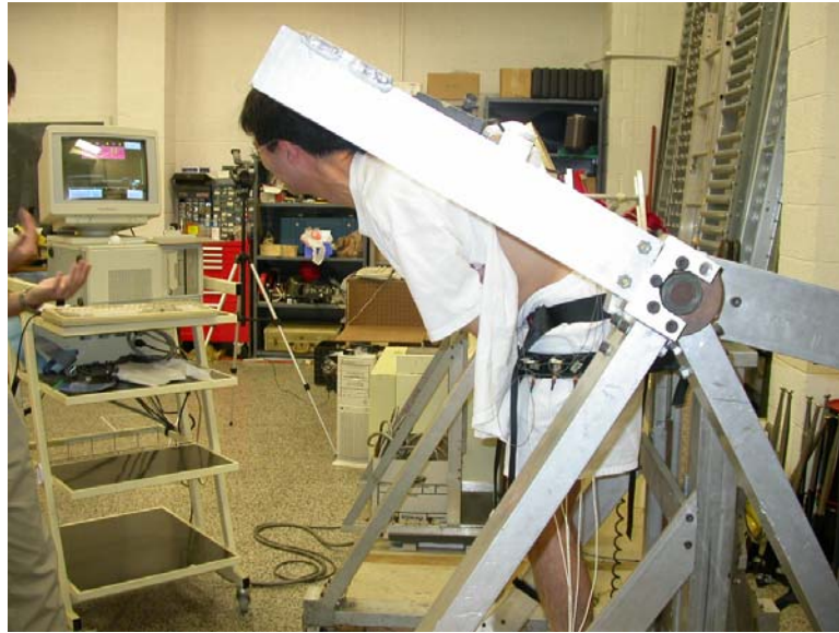
Figure 14: Dynamometer for the performance of maximum voluntary contractions for static extensions and flexions
