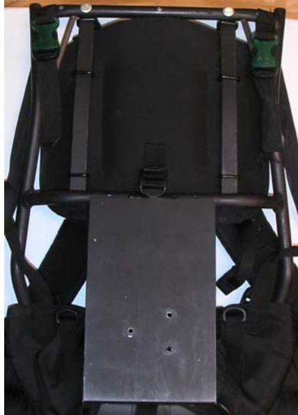
Figure 11: Aluminum plate attached to the frame of the new harness
