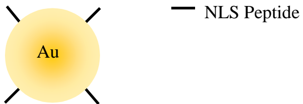
Figure 2. 20 nm gold nanoparticles with Nuclear Localization Signal (NLS) peptide attached to the gold surface via a thiol bond.
