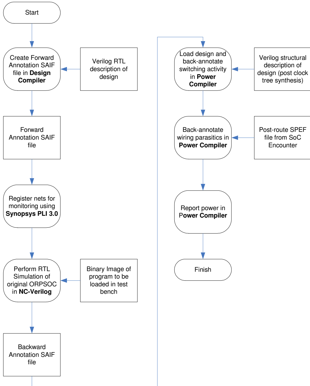
Figure 3-1: Flow for obtaining the power dissipation of the ORPSOC test case
