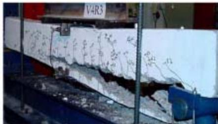
Figure 2.29. Strengthened beams after failure (Barros and Fortes, 2005)
