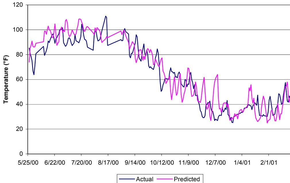
**Figure 2.4 – Actual and Predicted Bladder Outlet Water Temperatures**
