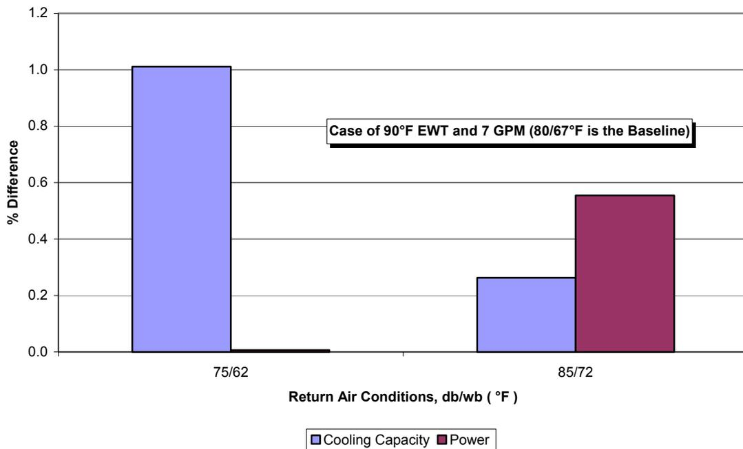
**Figure 2.1 – Correlation of Trane Performance Data Correction Factors to Bard Data**
