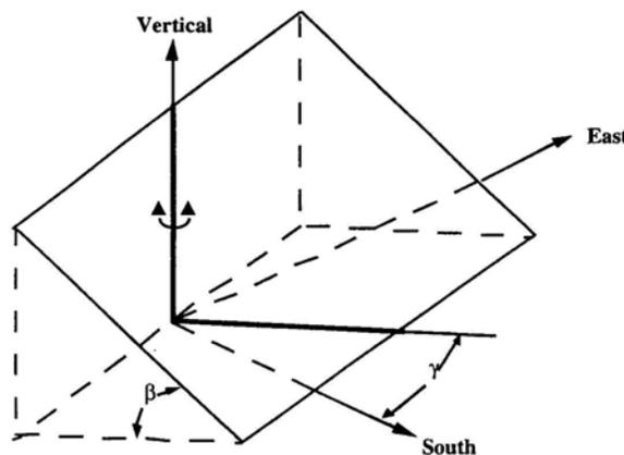
**Figure 4.8 – Surface Orientation for Solar Collectors in TRNSYS [6]**
