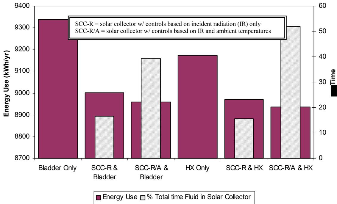
**Figure 4.7 – Geothermal Heat Pump Energy Use with Solar Collectors**
