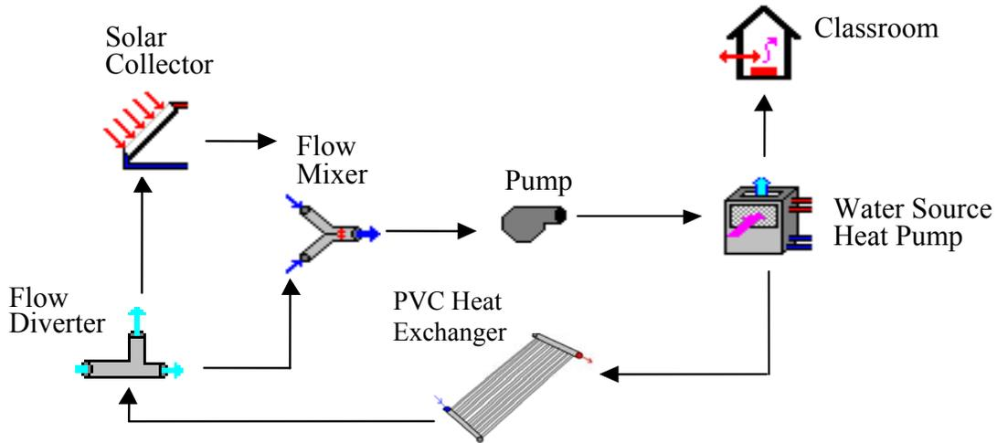
Figure 3.1 – Layout of TRNSYS model with Solar Collectors
