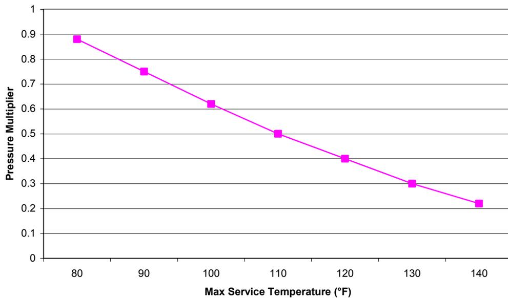
**Figure 5.4 – Thermal De-rating Factors for PVC Pressure Pipe [60]**
