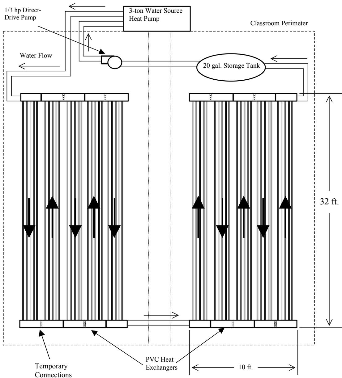
**Figure 5.2 – Layout of Geothermal Heat Pump System**
