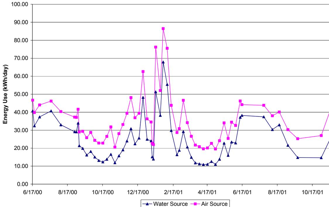
Figure 4.3 – TRNSYS Comparison of Water Source and Air Source Heat Pumps at WMES
