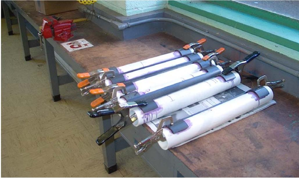
**Figure 5.3 – Assembly of Header Reinforcements**
