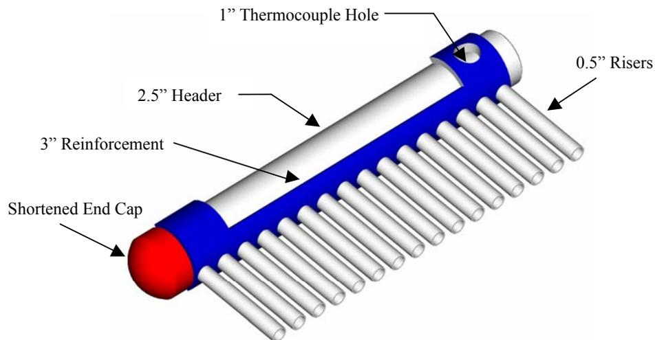
**Figure 5.1 – PVC Heat Exchanger Header Design**
