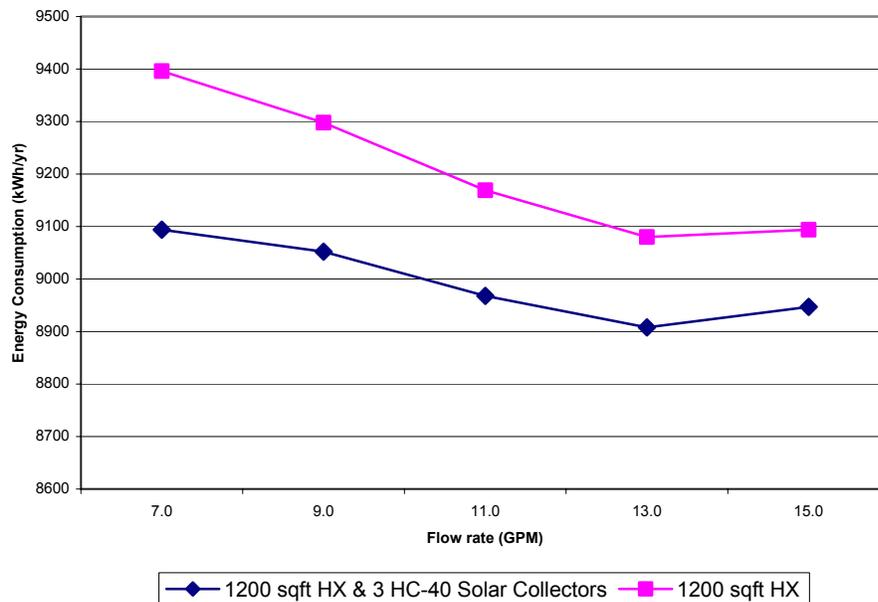
**Figure 4.9 – Heat Pump Annual Energy Use for Flow Rates Provided by Bard**
