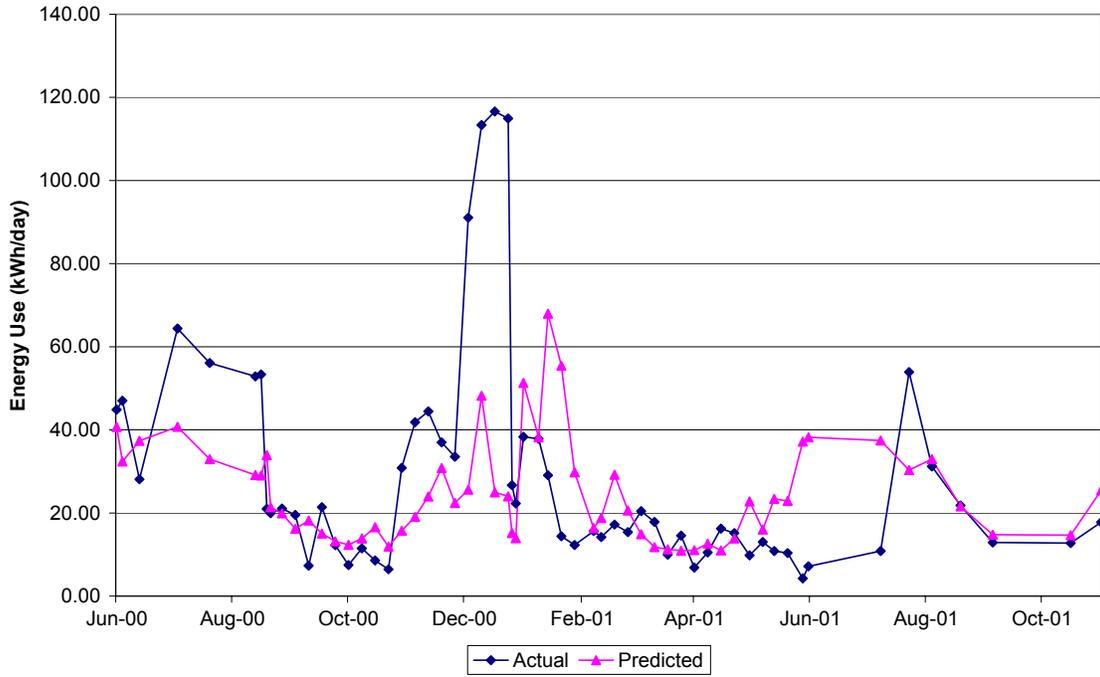
**Figure 4.1 – Predicted Vs. Experimental Energy Use for the Geothermal Heat Pump**
