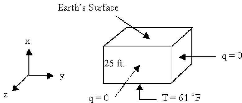
**Figure 2.3 – Boundary Conditions for Ground Temperatures**
