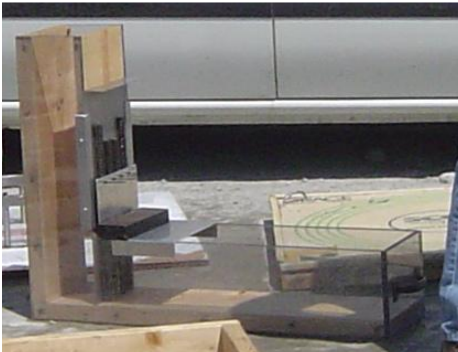
Figure 2.4 L-Box apparatus
