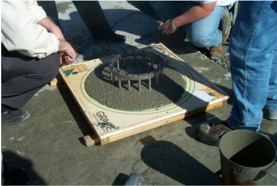
Figure 2.3 Measurement of the concrete spread.
